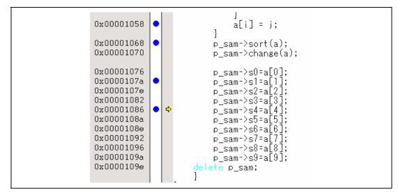
Figure 2.2 [Source] Window at Execution Halted (Sequential Break)
