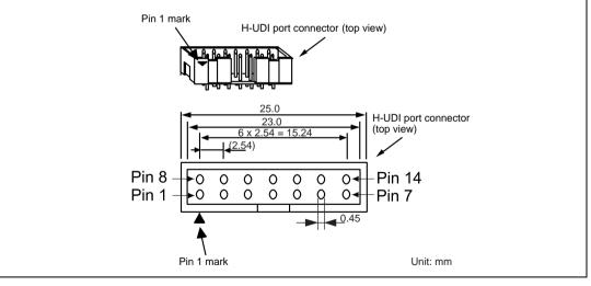
Figure 1.2 Pin Assignments of the H-UDI Port Connector (14 Pins)
