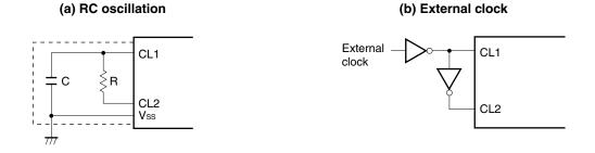
Caution When using the system clock oscillator, wire as follows in the area enclosed by the broken lines in the above figures to avoid an adverse effect from wiring capacitance.
