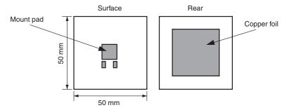
The mount pad on the surface and the copper foil on the rear are joined by thermal via.
