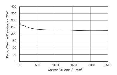
Measurement sample:  $\mu$ PD120N15TA Board material: Glass epoxy (single side) Board size: 50 mm x 50 mm x 1.6 mm
