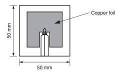
Figure 3-3. Thermal Resistance on Glass Epoxy Board (SC-74A)
