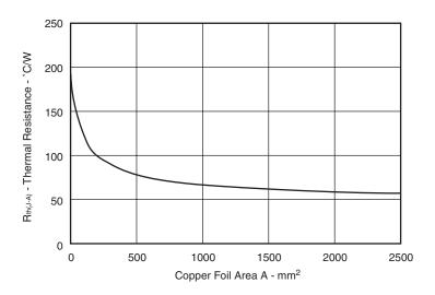
Measurement sample:  $\mu$ PD120N15T1B Board material: Glass epoxy (single side) Board size: 50 mm x 50 mm x 1.6 mm
