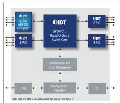
The SPS-1616 is IDT's RapidIO 2 switch that is targeted for applications that require several x1 links and also has one quad which support AES-128 encryption and can be used to scramble RapidIO packets for out of the box links
