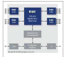
The CPS-1616 is IDT's RapidIO 2 switch that is targeted for applications that require several x1 links that can support up to 6.25 Gbaud per serial link. It has up to 16 x1 ports.
