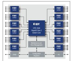
The CPS-1848 is IDT's largest RapidIO 2 switch, ideal for backplanes in large systems or on boards that require several high bandwidth connections of up to 20 Gbps per port. The CPS-1848 is the highest performance backplane switch in the embedded market.
