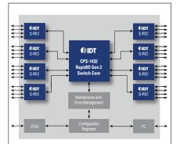
The CPS-1432 is IDT's RapidIO 2 switch that is ideal for boards that require several high bandwidth connections of up to 20 Gbps per port. The CPS-1432 can also be used in space constrained applications such as AMC or 6U/3U VPX where a large number of x4 links are used.
