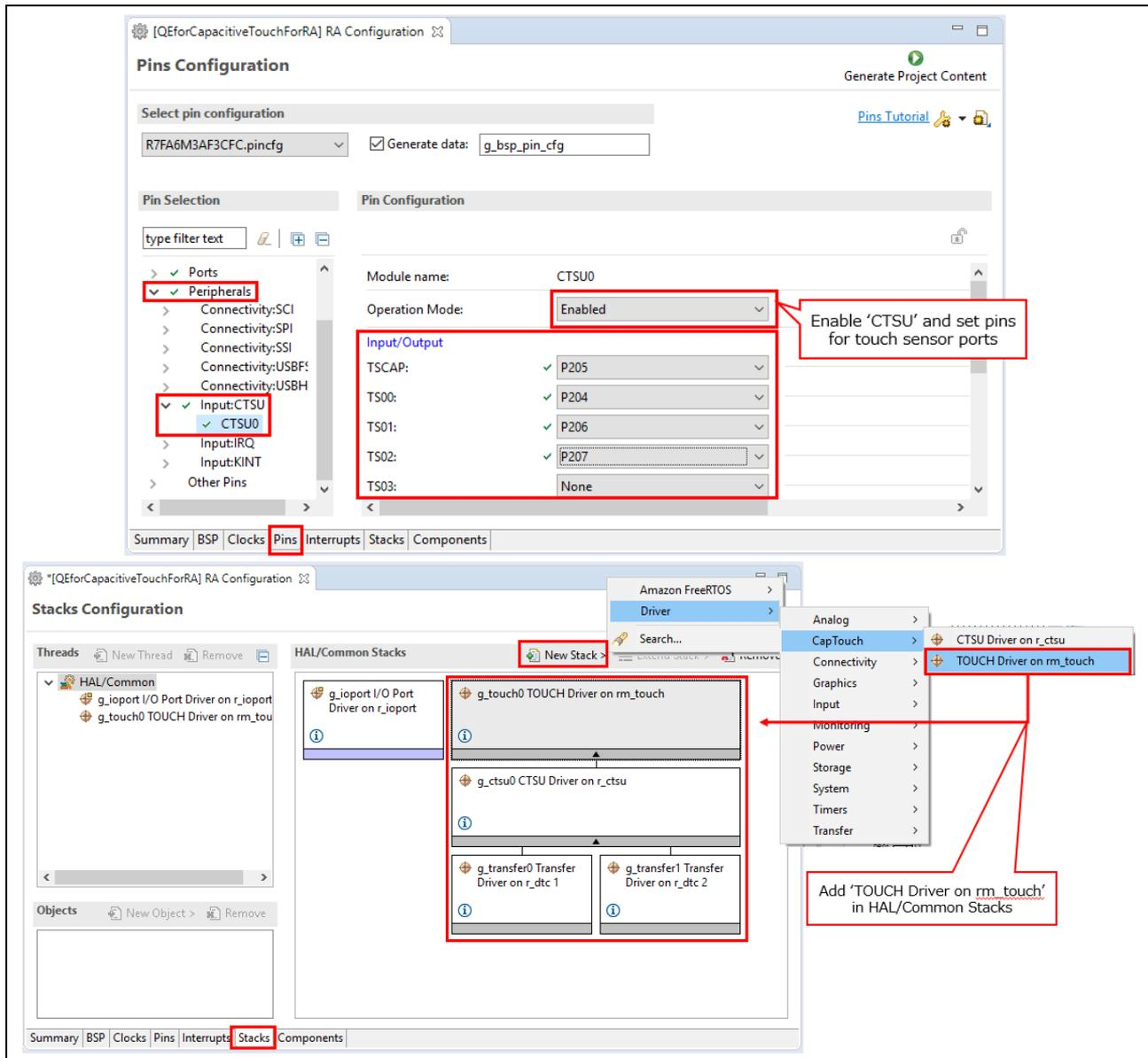
Figure 6 Adding FSP Components and Pin Setting
