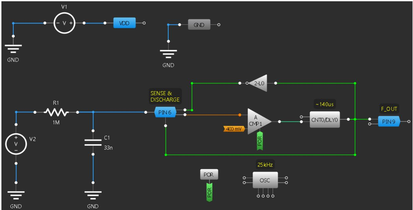
Figure 1. GreenPAK circuit design showing internal components and passive component connections
