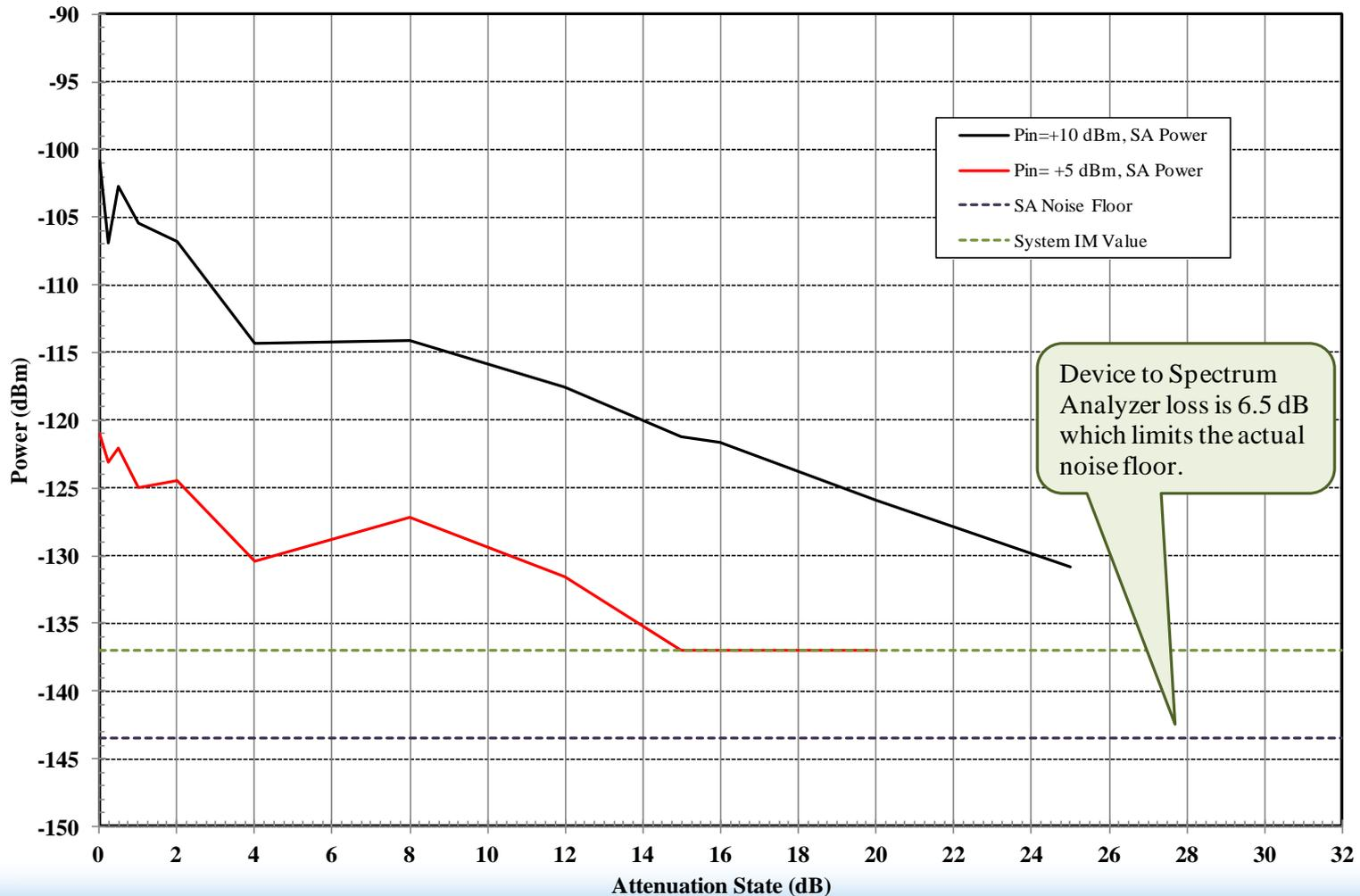
Device to Spectrum Analyzer loss is 6.5 dB which limits the actual noise floor.
