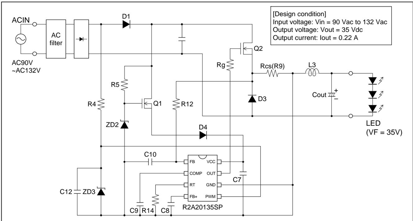
Figure 7.1 R2A20135EVB-ND1 Schematic
