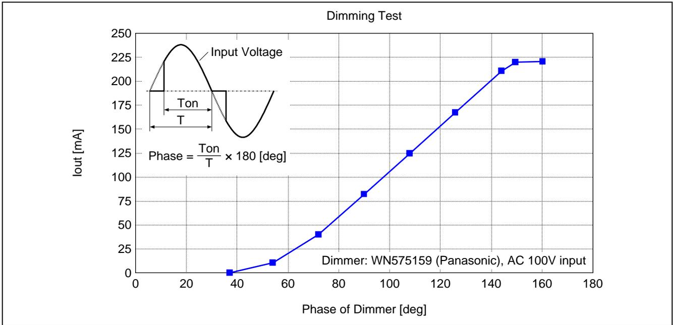
5.8 Dimming Characteristic (Trailing edge dimmer)
