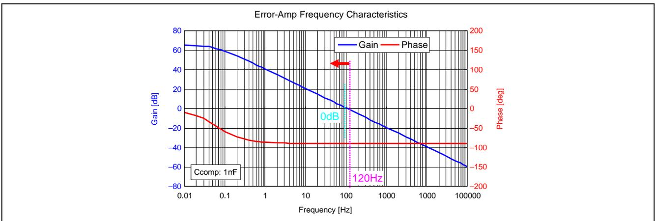
Figure 7.4 R2A20135EVB-ND1 Frequency Characteristics
