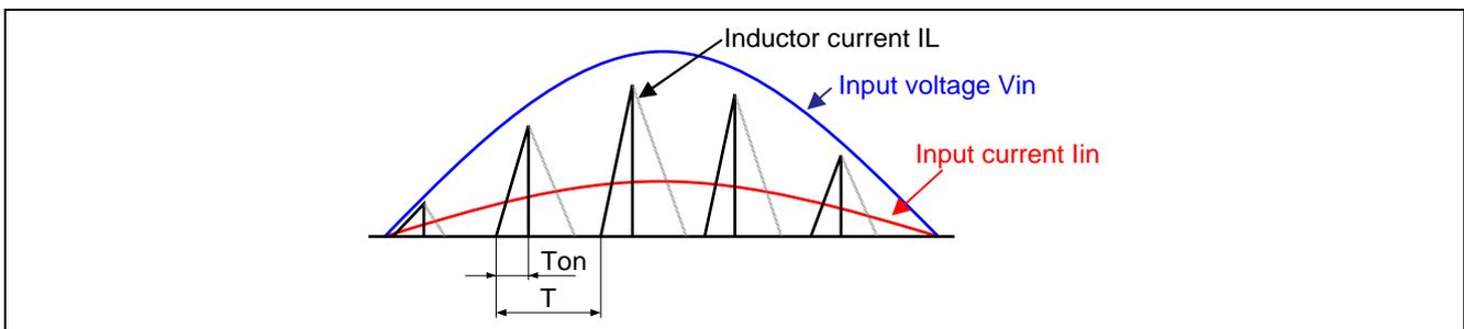
Figure 7.2 Input Current & Inductor Current
