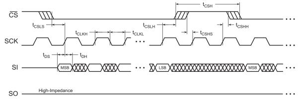
Figure 39. Serial Input Timing
