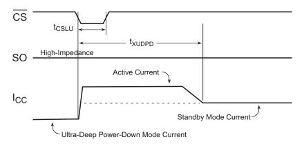
Figure 34. Exit Ultra-Deep Power-Down (Chip Select Toggle)
