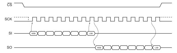
Figure 7. SPI Mode 0 and 3
