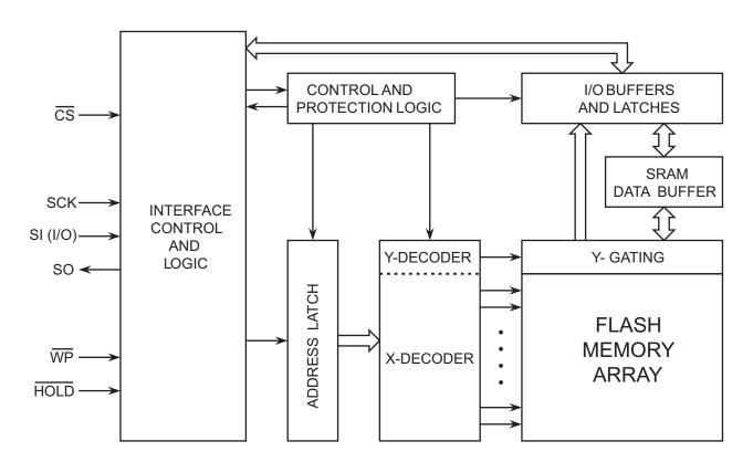
Figure 5. Block Diagram
