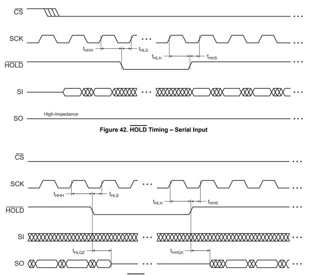
Figure 43. HOLD Timing - Serial Output
