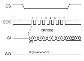
Figure 19. Write Enable
