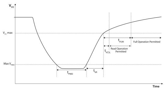
Figure 38. Power-Up Timing
