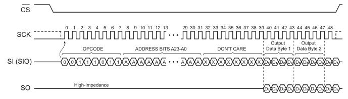
Figure 10. Dual-Output Read Array
