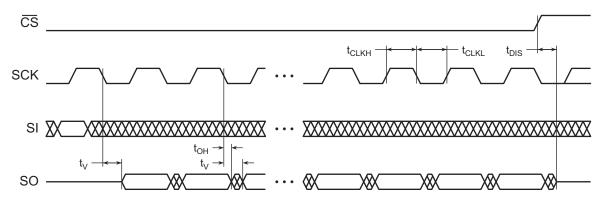
Figure 40. Serial Output Timing
