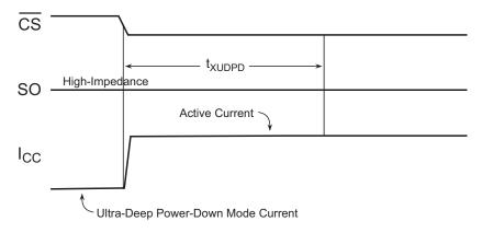
Figure 35. Exit Ultra-Deep Power-Down (Chip Select Low)
