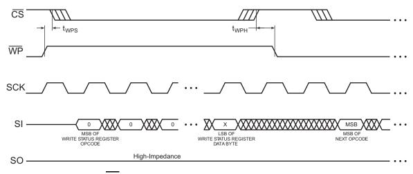
Figure 41. WP Timing for Write Status Register Command When BPL = 1
