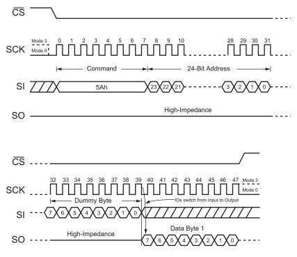
Figure 42. Read Serial Flash Discoverable Parameter Command
