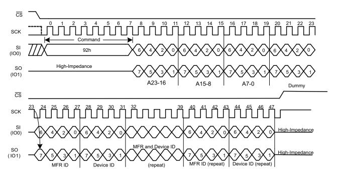
Figure 23. Dual I/O Read Manufacture ID/ Device ID Timing
