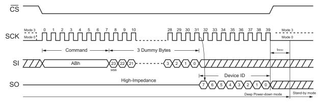
Figure 21. Release Power-Down / Device ID Command
