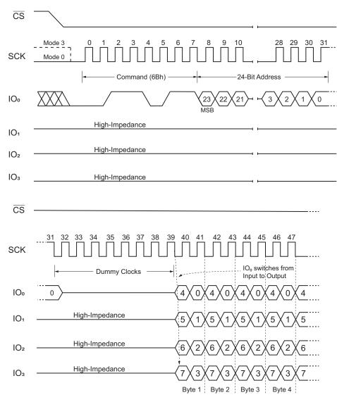
Figure 16. Fast Read Quad Output Command
