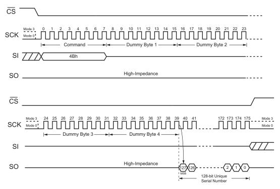
Figure 26. Read Unique ID Sequence Diagram
