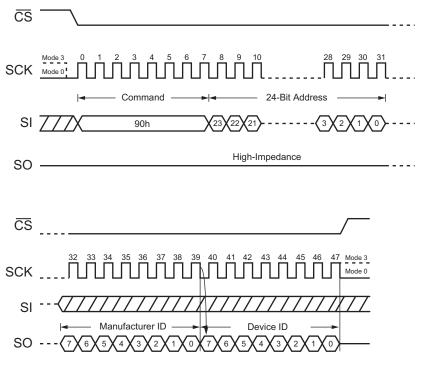
Figure 22. Read Manufacturer / Device ID Command
