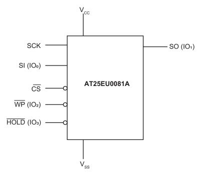
Figure 1. AT25EU0081A Logic Diagram
