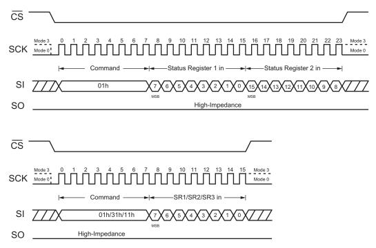
Figure 10. Write Status Register Command
