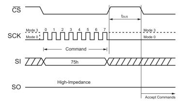
Figure 36. Program/Erase Suspend Command
