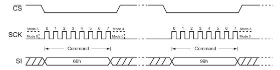
Figure 41. Enable Reset and Reset Command Sequence
