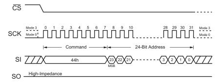
Figure 38. Erase Security Register Command
