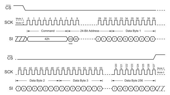
Figure 39. Program Security Register Command
