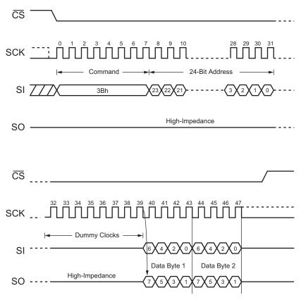
Figure 13. Fast Read Dual Output Command
