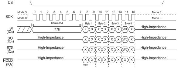
Figure 19. Set Burst with Wrap Command
