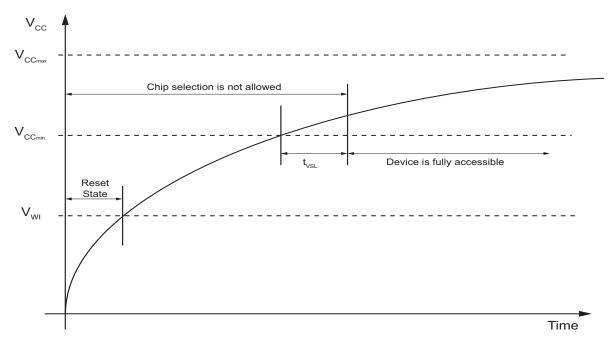
Figure 43. Power-Up Timing and Voltage Levels
