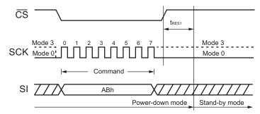
Figure 20. Release Power-Down Command
