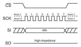
Figure 5. Write Enable Command for SPI Mode
