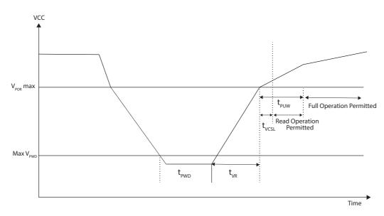
Figure 37. Power-Up Timing
