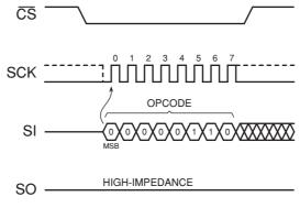
Figure 19. Write Enable
