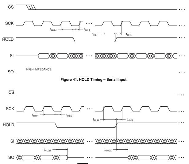
Figure 42. HOLD Timing – Serial Output
