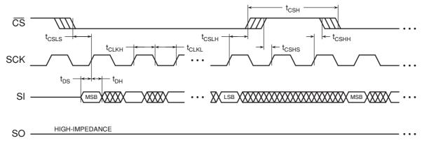
Figure 38. Serial Input Timing
