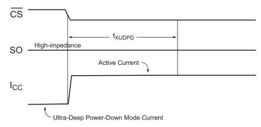
Figure 34. Exit Ultra-Deep Power-Down (Chip Select Low)
