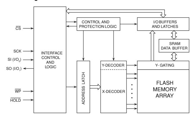
Figure 5. Block Diagram
