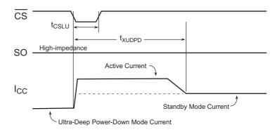
Figure 33. Exit Ultra-Deep Power-Down (Chip Select Toggle)
