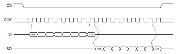
Figure 7. SPI Mode 0 and 3
