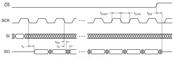
Figure 39. Serial Output Timing
