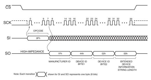
Figure 29. Read Manufacturer and Device ID
