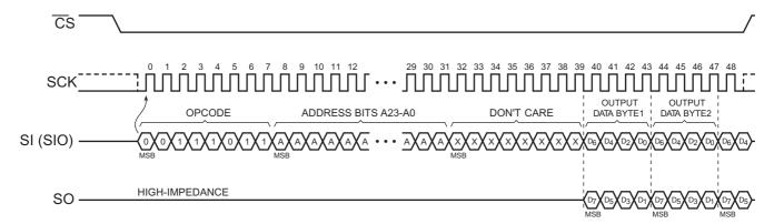
Figure 10. Dual-Output Read Array
