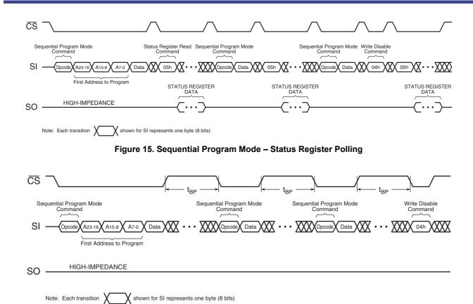
Figure 16. Sequential Program Mode - Waiting Maximum Byte Program Time
