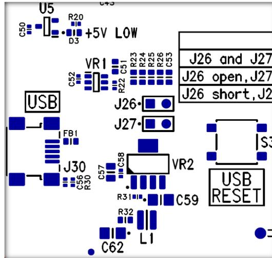
Figure 4: USB Interface Connector and Reset Switch
