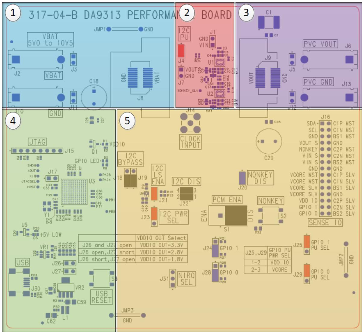
Figure 2: DA9313 Performance Board Sections (317-04-B Shown)
