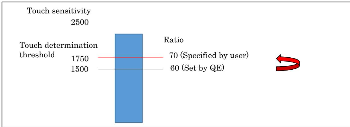
Figure 3 Example of changing the threshold ratio
