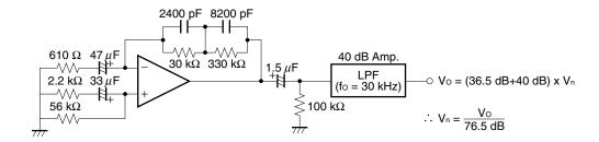
Fig.3 Flat Noise Measurement Circuit (FLAT+JIS A)
