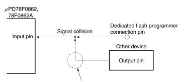
In the flash memory programming mode, the signal output by the device collides with the signal sent from the dedicated flash programmer. Therefore, isolate the signal of the other device.
