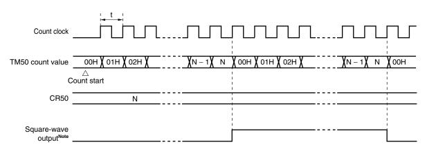
Figure 7-8. Square-Wave Output Operation Timing
