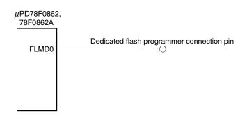
Figure 21-9. FLMD0 Pin Connection Example
