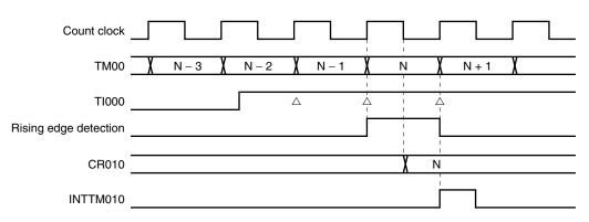
Figure 6-16. CR010 Capture Operation with Rising Edge Specified
