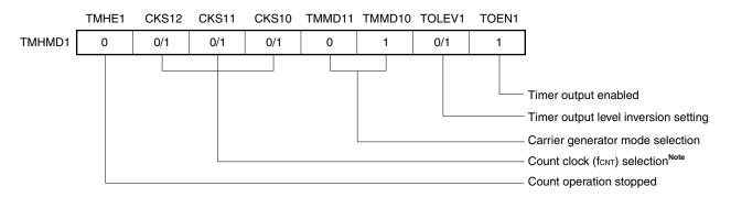
Note Check the setting of bit 1 (CSEL1) of the timer clock switch control register (CSEL) before setting CKS12, CKS11, and CKS10 to 0, 0, and 1, respectively (refer to Figure 8-7 Format of Timer Clock Switch Control Register (CSEL)).
