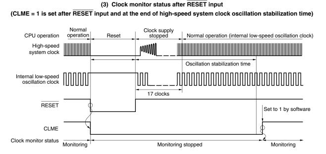
RESET input clears bit 0 (CLME) of the clock monitor mode register (CLM) to 0 and stops the clock monitor operation. When CLME is set to 1 by software at the end of the oscillation stabilization time (OSTS register reset value =  $05H (2^{16}/f_{XH})$ ) of the high-speed system clock, monitoring is started.
