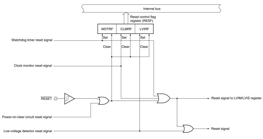
Figure 16-1. Block Diagram of Reset Function
