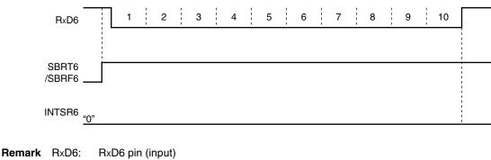
SBRT6: Bit 6 of asynchronous serial interface control register 6 (ASICL6) SBRF6: Bit 7 of ASICL6 INTSR6: Reception completion interrupt request
