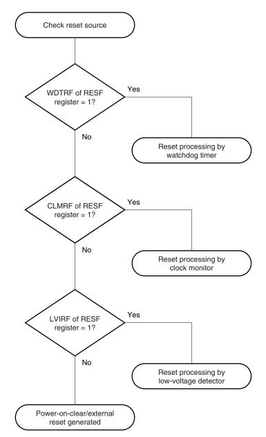
Figure 18-3. Example of Software Processing After Release of Reset (2/2)
