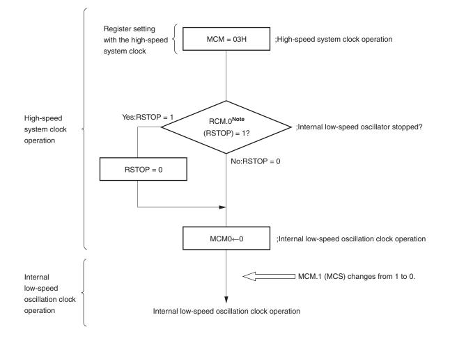
**Note** This is necessary only when "clock can be stopped by software" is selected for the internal low-speed oscillator by a mask option (option byte when using a flash memory version).
