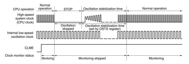
When bit 0 (CLME) of the clock monitor mode register (CLM) is set to 1 before entering STOP mode, monitoring automatically starts at the end of the high-speed system clock oscillation stabilization time. Monitoring is stopped in STOP mode and during the oscillation stabilization time.
