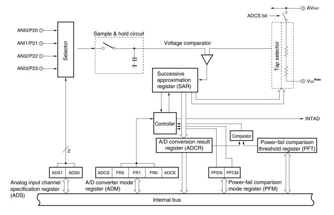
Figure 10-1. Block Diagram of A/D Converter
