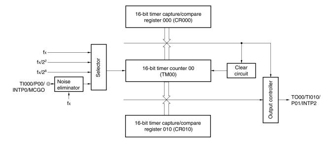
Figure 6-14. Configuration Diagram of PPG Output
