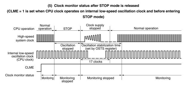
When bit 0 (CLME) of the clock monitor mode register (CLM) is set to 1 before entering STOP mode, monitoring automatically starts at the end of the high-speed system clock oscillation stabilization time. Monitoring is stopped in STOP mode and during the oscillation stabilization time.
