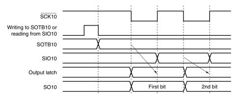
The first bit is directly latched by the SOTB10 register to the output latch at the falling (or rising) edge of the  $\overline{SCK10}$ , and output from the SO10 pin via an output selector. Then, the value of the SOTB10 register is transferred to the SIO10 register at the next rising (or falling) edge of  $\overline{SCK10}$ , and shifted one bit. At the same time, the first bit of the receive data is stored in the SIO10 register via the SI10 pin.
