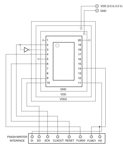
Figure 21-3. Example of Wiring Adapter for Flash Memory Writing in 3-Wire Serial I/O (CSI10 + HS) Mode
