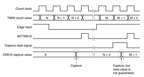
Figure 6-37. Capture Register Data Retention Timing
