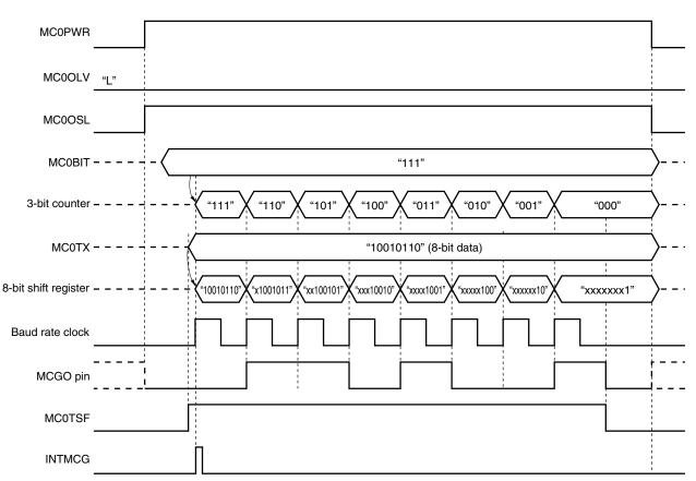
(2) Transmit timing (MC0OLV = 0, total transmit bit length = 8 bits)
