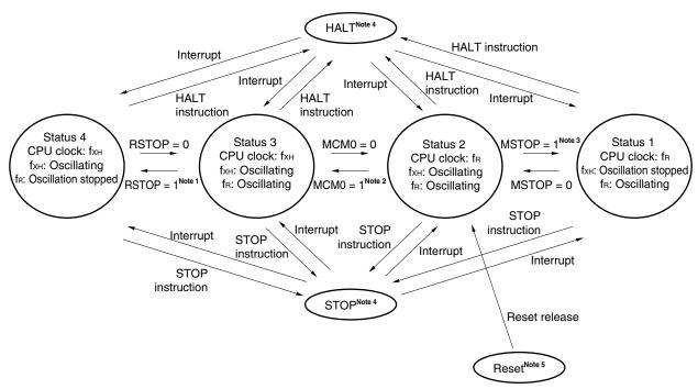
(1) When "Internal low-speed oscillator can be stopped by software" is selected by mask option
