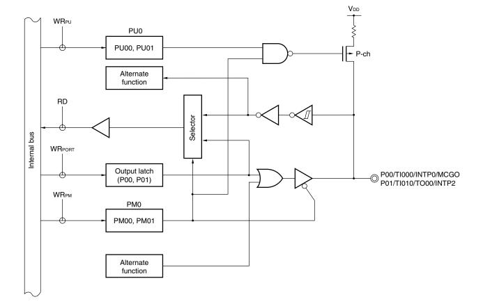
Figure 4-2. Block Diagram of P00 and P01
