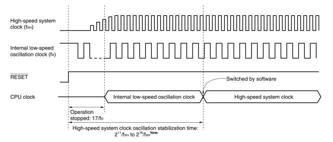
Figure 5-12. Timing Diagram of CPU Default Start Using Internal Low-Speed Oscillation Clock
