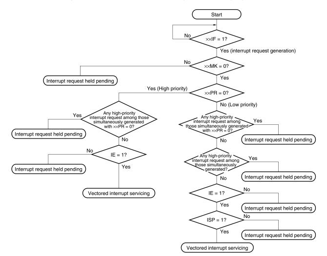
Figure 14-9. Interrupt Request Acknowledgment Processing Algorithm
