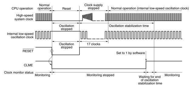
RESET input clears bit 0 (CLME) of the clock monitor mode register (CLM) to 0 and stops the clock monitor operation. Even if CLME is set to 1 by software during the oscillation stabilization time (OSTS register reset value =  $05H (2^{16}/f_{XH})$ ) of the high-speed system clock, monitoring is not performed until the oscillation stabilization time of the high-speed system clock ends. Monitoring is automatically started at the end of the oscillation stabilization time.
