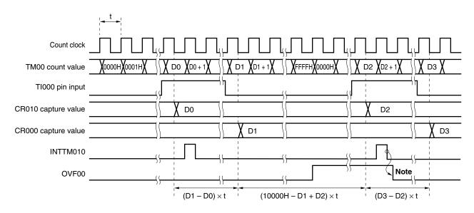
Figure 6-23. Timing of Pulse Width Measurement Operation with Free-Running Counter and Two Capture Registers (with Rising Edge Specified)
