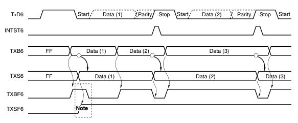
Figure 11-17. Timing of Starting Continuous Transmission
