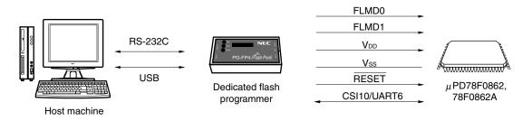
A host machine that controls the dedicated flash programmer is necessary.
