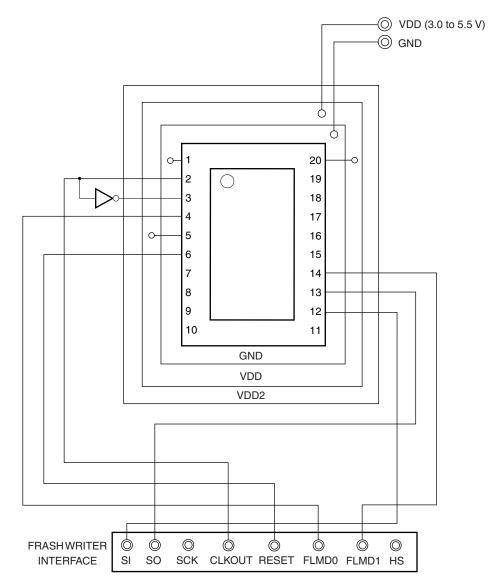
Figure 21-4. Example of Wiring Adapter for Flash Memory Writing in UART (UART6) Mode
