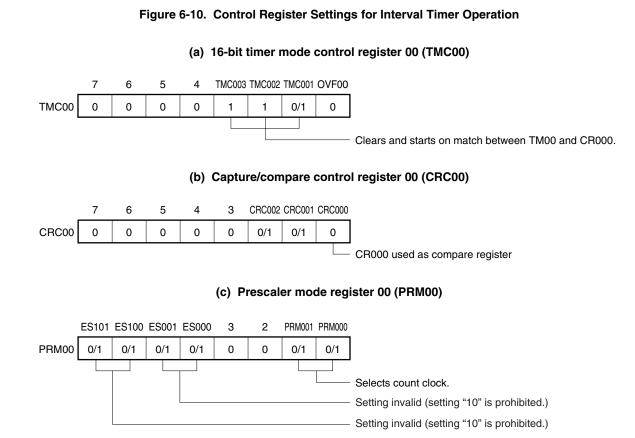
**Remark** 0/1: Setting 0 or 1 allows another function to be used simultaneously with the interval timer. See the description of the respective control registers for details.
