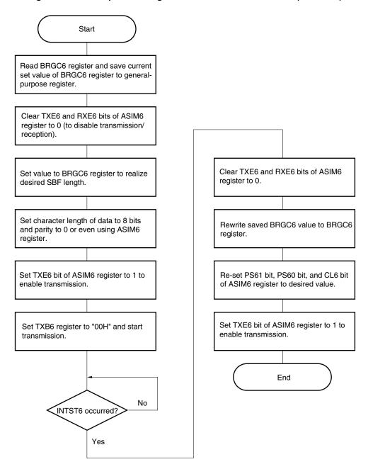
Figure 11-22. Example of Setting Procedure of SBF Transmission (Flowchart)
