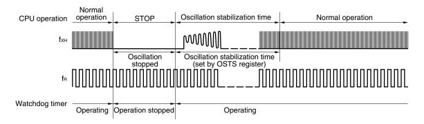
(3) When the CPU clock is the internal low-speed oscillation clock (fR) and the watchdog timer operation clock is the high-speed system clock (fxH) when the STOP instruction is executed
