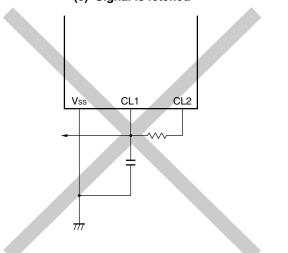
Figure 5-11. Examples of Incorrect Resonator Connection
