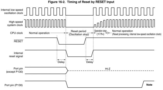
**Note** Set P130 to high-level output by software.
