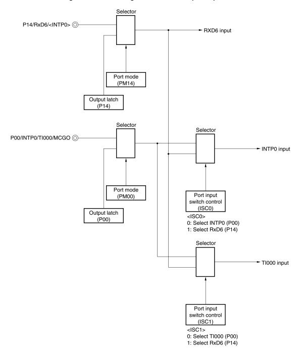
Figure 11-3. Port Configuration for LIN Reception Operation
