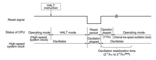
**Note** Waiting for the oscillation stabilization time is not required when the external RC oscillation clock or Internal high-speed oscillation clock is selected as the high-speed system clock by a mask option (option byte when using a flash memory version). Therefore, the CPU clock can be switched without reading the OSTC value.
