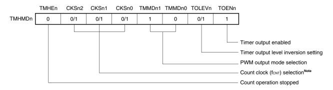
Note Check the setting of bit 0 (CSEL0) of the timer clock switch control register (CSEL) before setting CKS02, CKS01, and CKS00 to 1, 0, and 1, respectively, and check the setting of bit 1 (CSEL1) of the CSEL register before setting CKS12, CKS11, and CKS10 to 0, 0, and 1, respectively (refer to Figure 8-7 Format of Timer Clock Switch Control Register (CSEL)).
