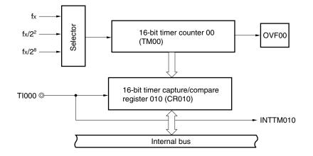
Figure 6-18. Configuration Diagram for Pulse Width Measurement with Free-Running Counter
