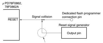
In the flash memory programming mode, the signal output by the reset signal generator collides with the signal output by the dedicated flash programmer. Therefore, isolate the signal of the reset signal generator.
