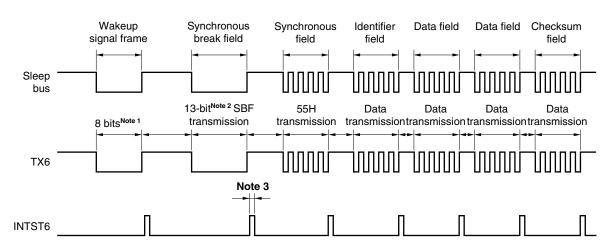
Figure 11-1. LIN Transmission Operation
