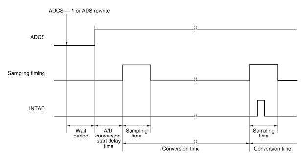
Figure 10-21. Timing of A/D Converter Sampling and A/D Conversion Start Delay
