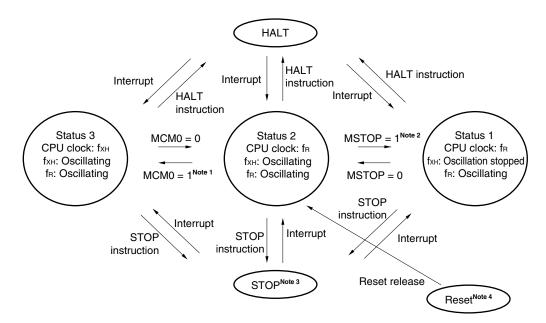
(2) When "Internal low-speed oscillator cannot be stopped" is selected by mask option
