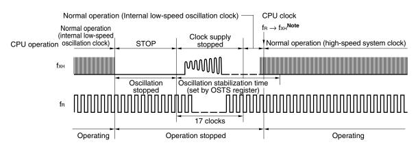
**Note** Confirm the oscillation stabilization time of fxH using the oscillation stabilization time counter status register (OSTC).
