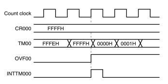
Figure 6-36. Operation Timing of OVF00 Flag
