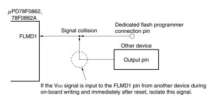
Figure 21-10. FLMD1 Pin Connection Example
