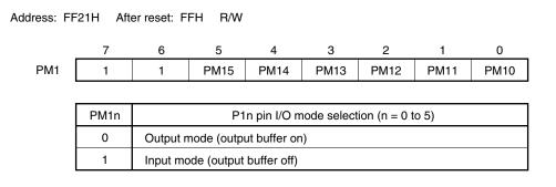
When using the P12/TOH1/SO10/(INTP3), P13/(TOH1)/TxD6/INTP1/(MCGO), or P15/TOH0/FLMD1 pin as a timer output, set the port mode register and port output latch as follows.
