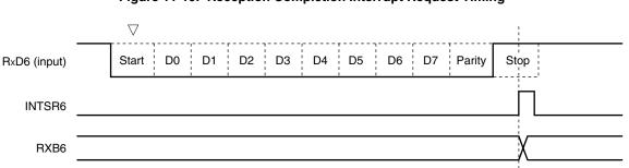
Figure 11-19. Reception Completion Interrupt Request Timing
