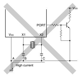
Figure 5-9. Examples of Incorrect Resonator Connection
