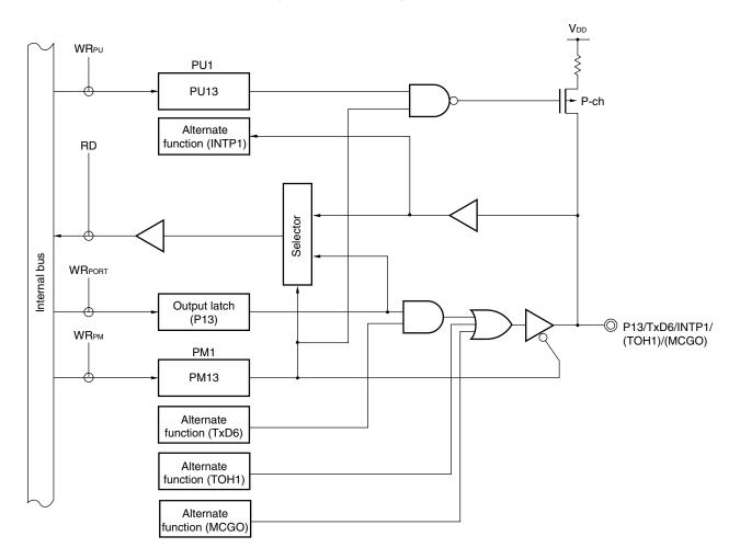
PU1: Pull-up resistor option register 1
