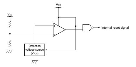
Figure 18-1. Block Diagram of Power-on-Clear Circuit
