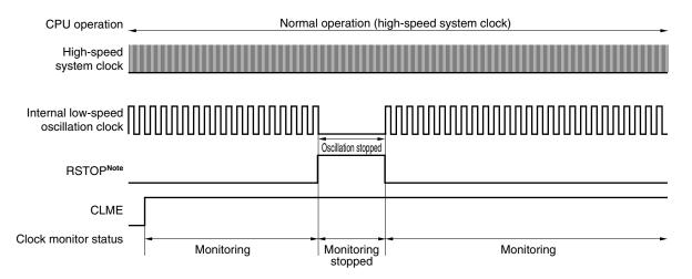
When bit 0 (CLME) of the clock monitor mode register (CLM) is set to 1 before or while oscillation of the internal low-speed oscillation clock is stopped, monitoring automatically starts after the internal low-speed oscillation clock is stopped. Monitoring is stopped when oscillation of the internal low-speed oscillation clock is stopped.
