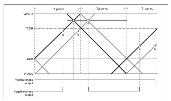
Figure 12.47 Example of Complementary PWM Mode Waveform Output (2)
