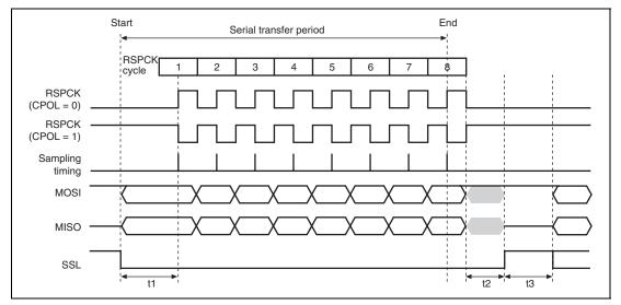
Figure 25.11 RSPI Transfer Format (CPHA = 0)
