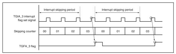
Figure 12.75 Example of Interrupt Skipping Operation
