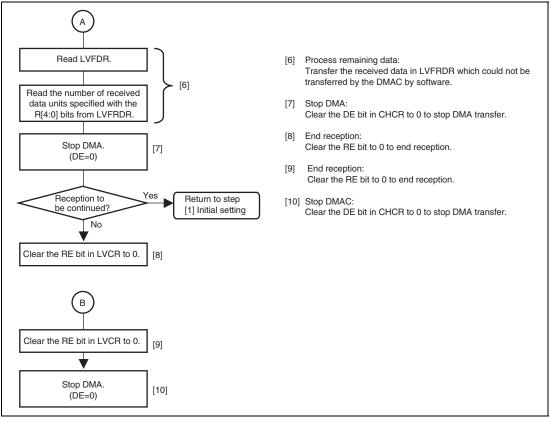
Figure 24.10 Example of Data Transfer in LVDS Receive FIFO Data Register by DMAC (2)
