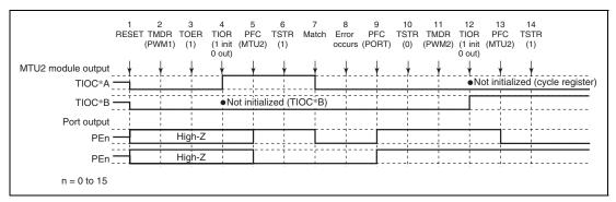
Figure 12.147 Error Occurrence in PWM Mode 1, Recovery in PWM Mode 2
