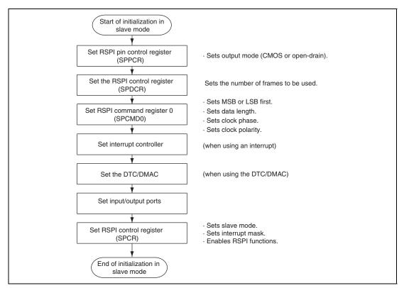
Figure 25.26 Example of Initialization Flowchart in Slave Mode
