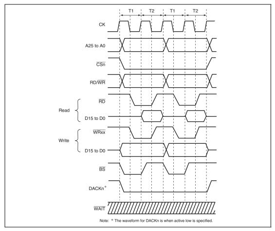
Figure 10.4 Continuous Access for Normal Space 2
