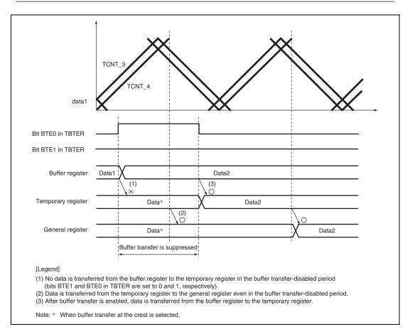
Figure 12.76 Example of Operation when Buffer Transfer is Suppressed (BTE1 = 0 and BTE0 = 1)
