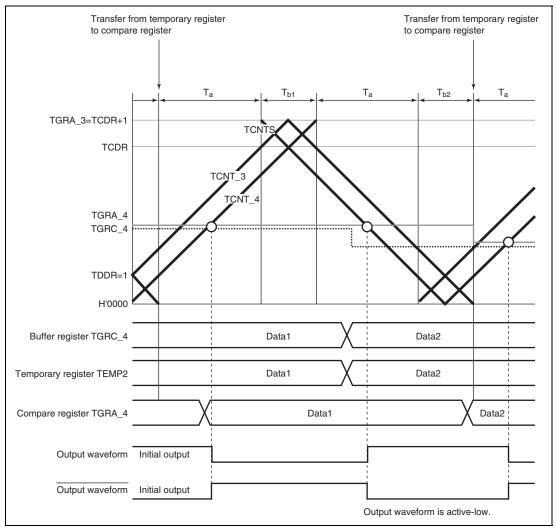
Figure 12.41 Example of Operation without Dead Time
