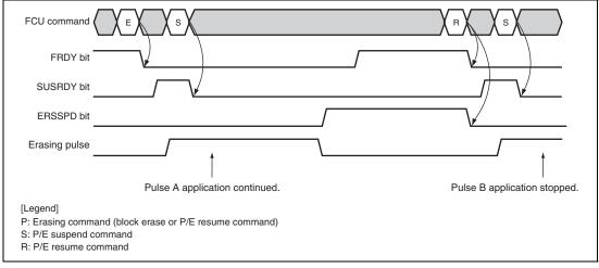
Figure 29.30 Suspending Erasure Processing (Erasure-Priority Mode)
