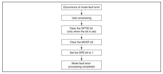
Figure 25.32 Error Processing (Mode Fault Error)
