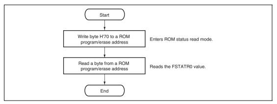
Figure 29.25 Procedure for Checking Status Register 0
