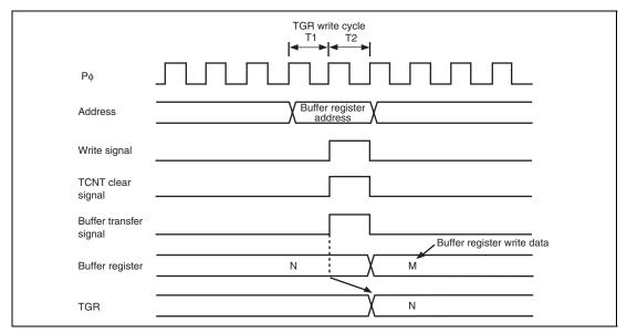
Figure 12.125 Contention between Buffer Register Write and TCNT Clear
