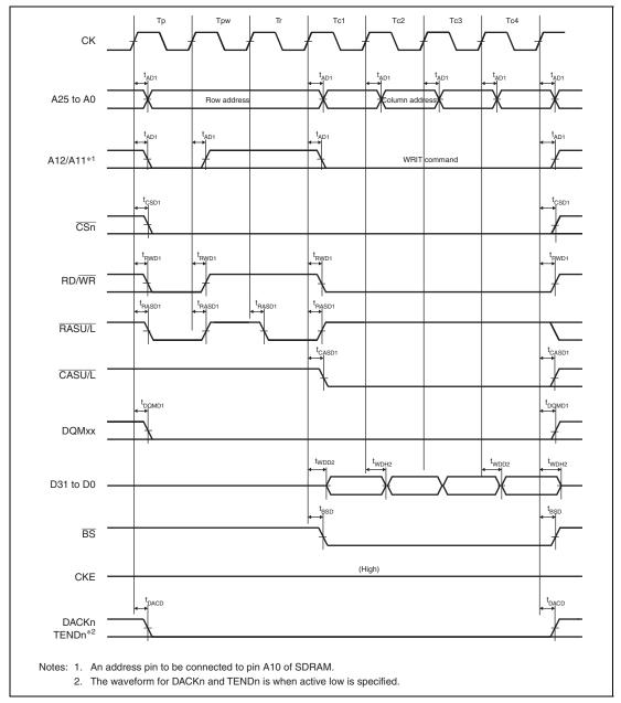
Figure 35.36 Synchronous DRAM Burst Write Bus Cycle (Four Write Cycles)
