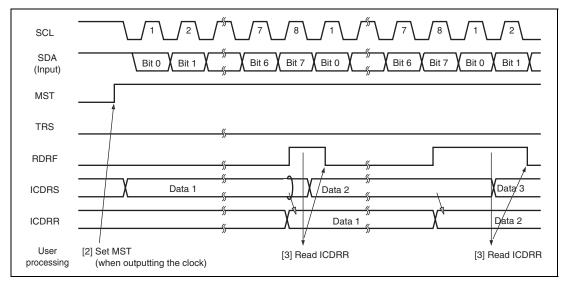
Figure 20.15 Receive Mode Operation Timing
