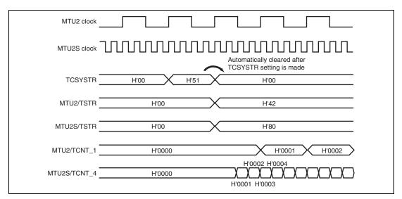
Figure 12.84 (3) Example of Synchronous Counter Start Operation (MTU2-to-MTU2S Clock Frequency Ratio = 1:4)
