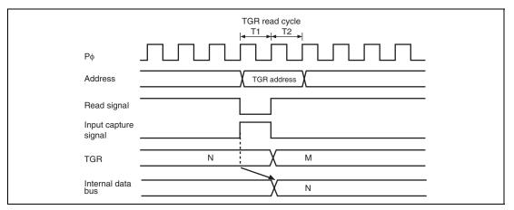
Figure 12.126 Contention between TGR Read and Input Capture (Channels 0 to 4)
