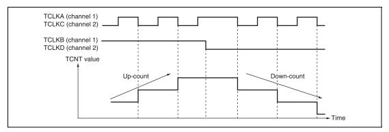
Figure 12.31 Example of Phase Counting Mode 2 Operation
