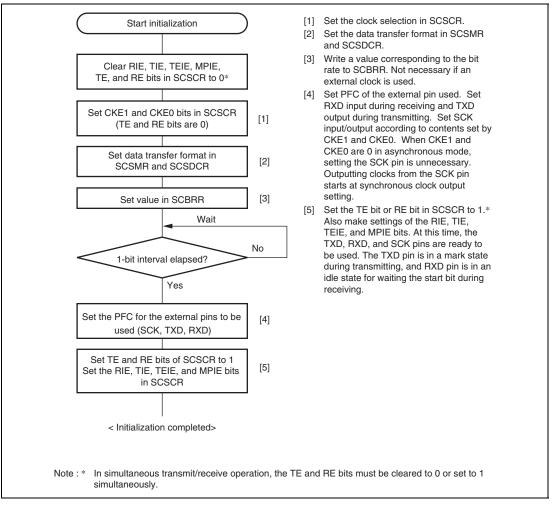
Figure 18.3 Sample Flowchart for SCI Initialization
