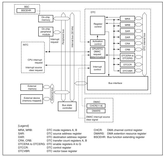
Figure 9.1 Block Diagram of DTC
