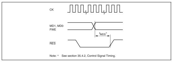
Figure 4.3 Reset Input Timing when Changing Operating Mode
