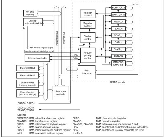
Figure 11.1 Block Diagram of DMAC
