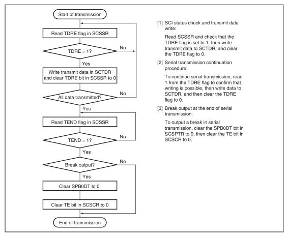
Figure 18.4 Sample Flowchart for Transmitting Serial Data
