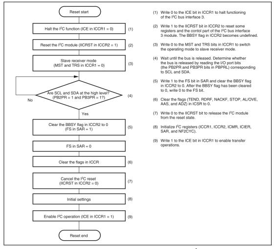
Figure 20.20 Sequence for Using the IICRST Bit to Reset I<sup>2</sup>C Bus Interface 3
