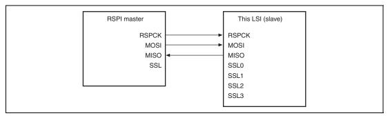
Figure 25.10 Master (Clock Synchronous)/Slave (Clock Synchronous) Configuration Example (This LSI = Slave, CPHA = 1)
