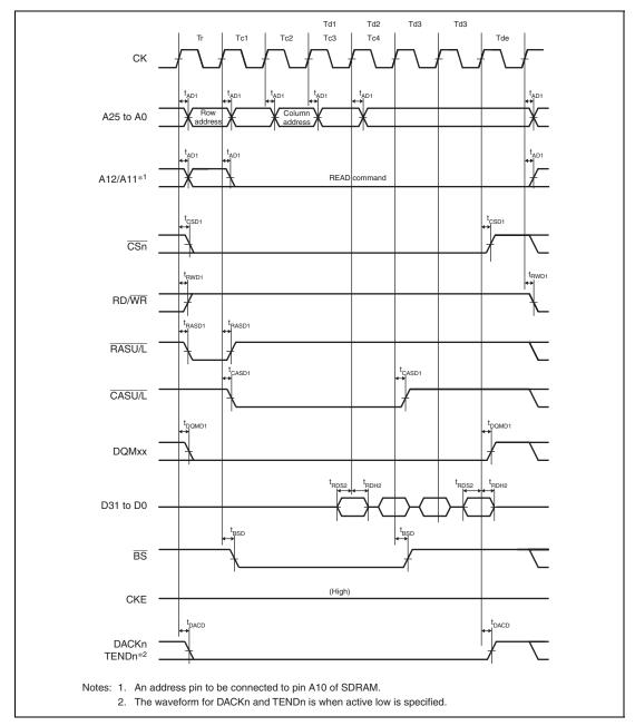
Figure 35.31 Synchronous DRAM Burst Read Bus Cycle (Four Read Cycles) (Bank Active Mode: ACT + READ Commands, CAS Latency 2, WTRCD = 0 Cycle)
