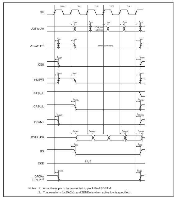
Figure 35.35 Synchronous DRAM Burst Write Bus Cycle (Four Write Cycles) (Bank Active Mode: WRITE Command, Same Row Address, WTRCD = 0 Cycle, TRWL = 0 Cycle)
