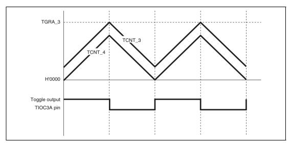
Figure 12.54 Example of Toggle Output Waveform Synchronized with PWM Output
