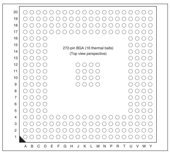
Figure 1.3 Pin Assignment Diagram (P-FBGA1717-272)
