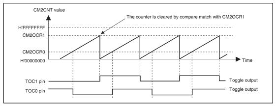
Figure 16.6 Example of Output Compare Operation
