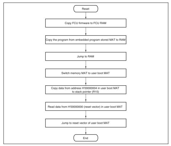
Figure 29.31 Overview of Boot Sequence in User Boot Mode
