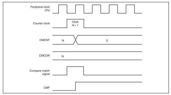
Figure 15.4 Timing of CMF Setting
