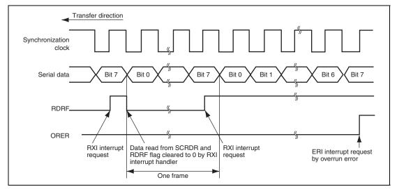
Figure 18.13 Example of SCI Receive Operation (when LSB-First Transfer is Selected)
