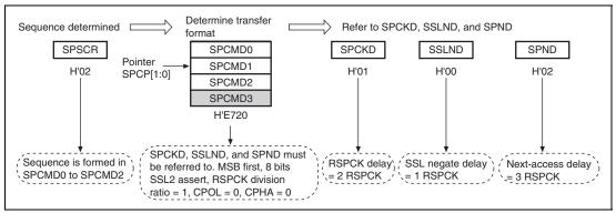
Figure 25.28 Determination Procedure of Serial Transfer Mode in Master Mode
