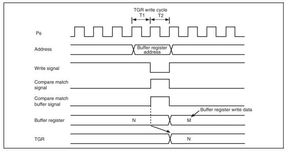
Figure 12.124 Contention between Buffer Register Write and Compare Match
