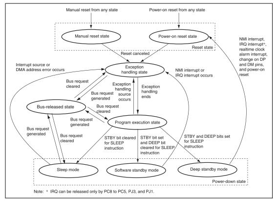
Figure 2.6 Transitions between Processing States
