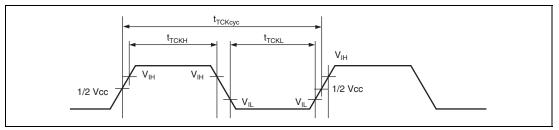
Figure 35.66 TCK Input Timing
