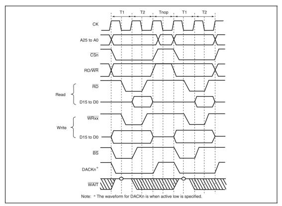
Figure 10.3 Continuous Access for Normal Space 1
