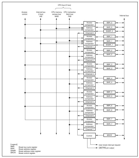
Figure 8.1 Block Diagram of UBC
