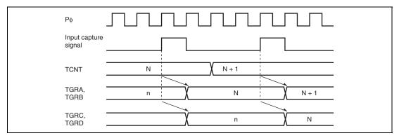
Figure 12.104 Buffer Operation Timing (Input Capture)
