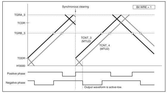
Figure 12.59 Example of Synchronous Clearing in Interval Tb at Crest (Timing (6) in Figure 12.56; Bit WRE in TWCR of MTU2 is 1)
