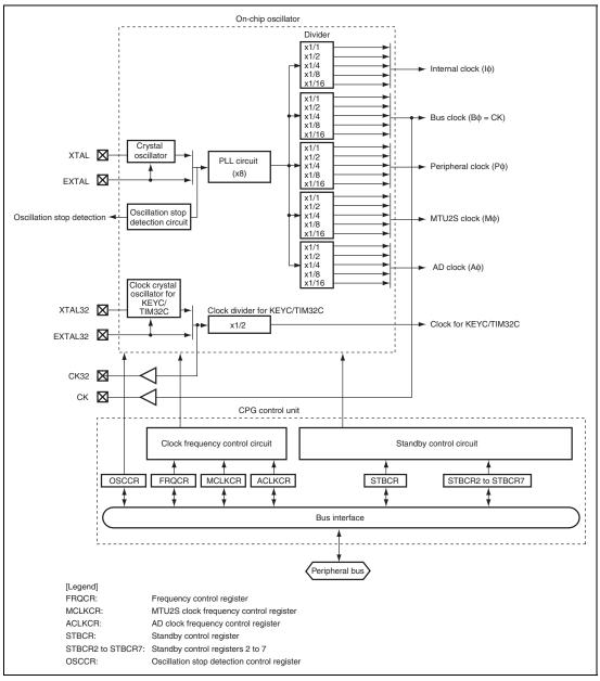
Figure 5.1 Block Diagram of Clock Pulse Generator
