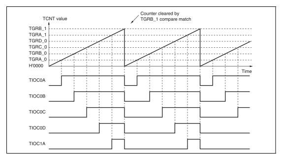
Figure 12.27 Example of PWM Mode Operation (2)
