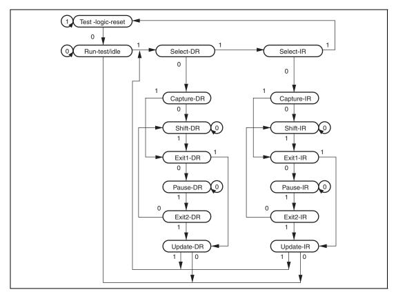
Figure 33.2 TAP Controller State Transitions
