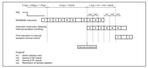
Figure 7.9 Example of Pipeline Operation when Interrupt is Accepted during RESBANK Instruction Execution (Register Banking with Register Bank Overflow)
