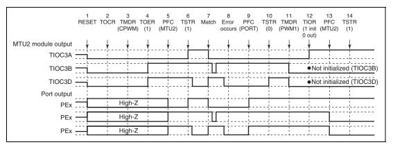
Figure 12.160 Error Occurrence in Complementary PWM Mode, Recovery in PWM Mode 1
