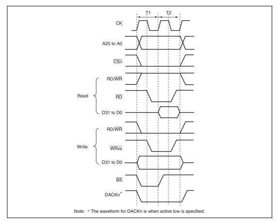
Figure 10.2 Normal Space Basic Access Timing (Access Wait 0)
