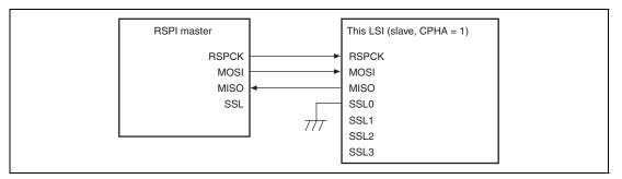
Figure 25.5 Single-Master/Single-Slave Configuration Example (This LSI = Slave, CPHA = 1)
