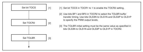
Figure 12.3 PWM Output Level Setting Procedure in Buffer Operation
