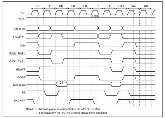
Figure 10.30 Low-Frequency Mode Access Timing
