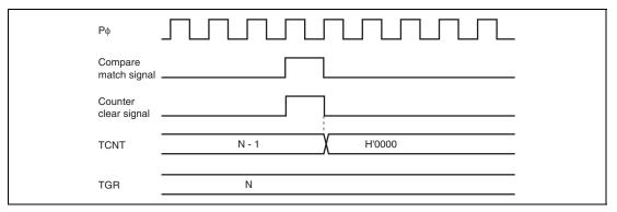
Figure 12.101 Counter Clear Timing (Compare Match) (Channel 5)
