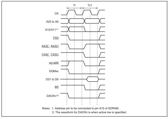
Figure 10.25 Single Write Timing (Bank Active, Different Bank)
