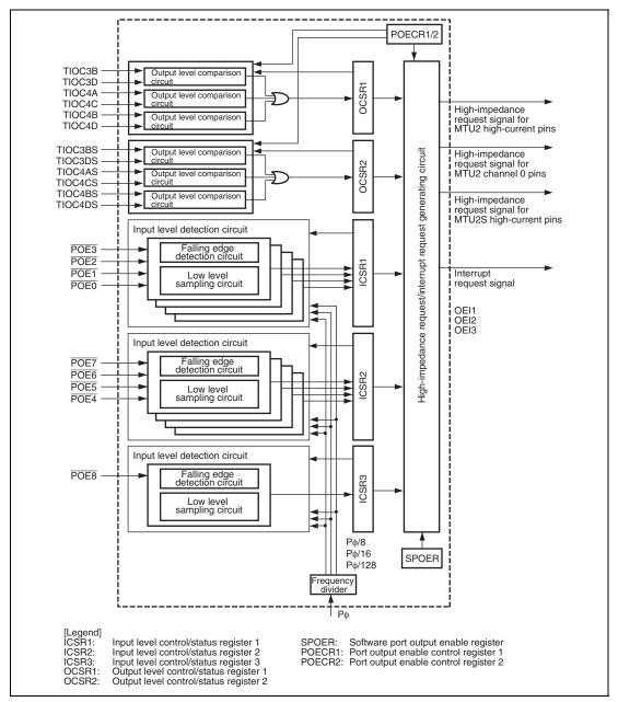
Figure 14.1 Block Diagram of POE2
