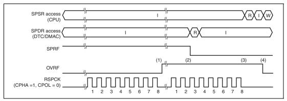
Figure 25.18 SPRF and OVRF Bit Operation Example
