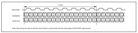
Figure 24.5 Received Data Bit Length
