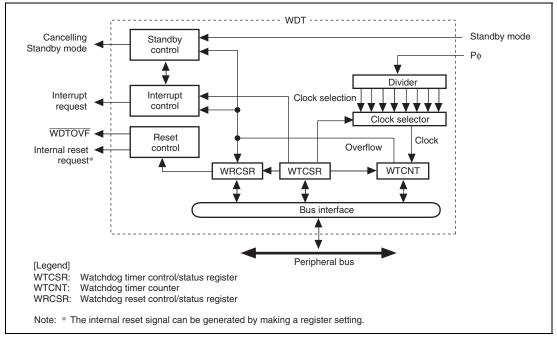
Figure 17.1 Block Diagram of WDT
