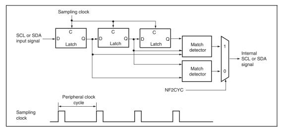
Figure 20.17 Block Diagram of Noise Filter
