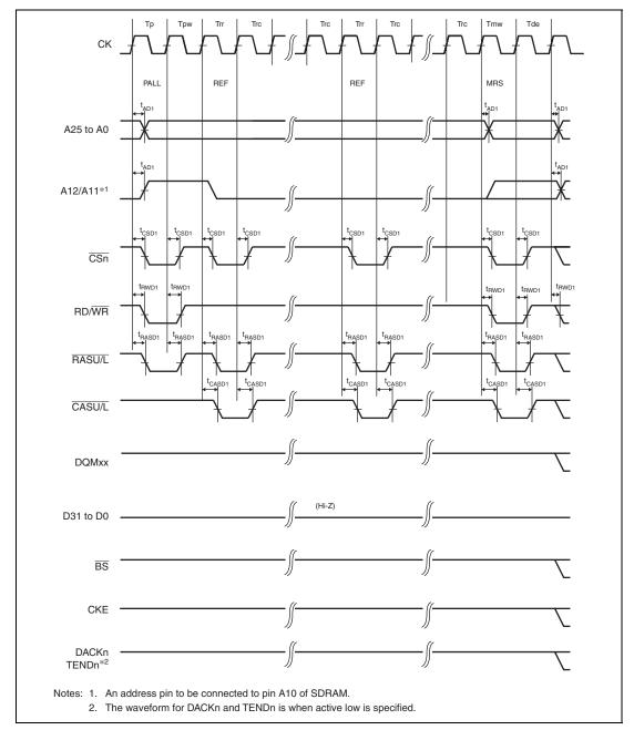
Figure 35.39 Synchronous DRAM Mode Register Write Timing (WTRP = 1 Cycle)
