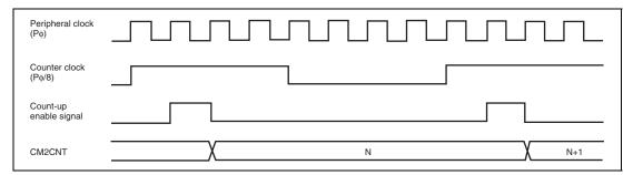
Figure 16.9 Count Timing (P\phi/8)
