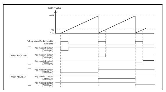
Figure 28.7 Operation Example with KSPC = 1
