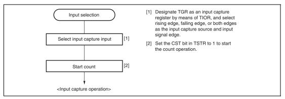
Figure 12.10 Example of Input Capture Operation Setting Procedure
