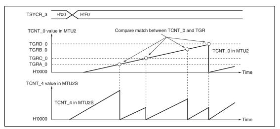
Figure 12.86 (2) Example of MTU2S Counter Clearing Caused by MTU2 Flag Setting Source (2)
