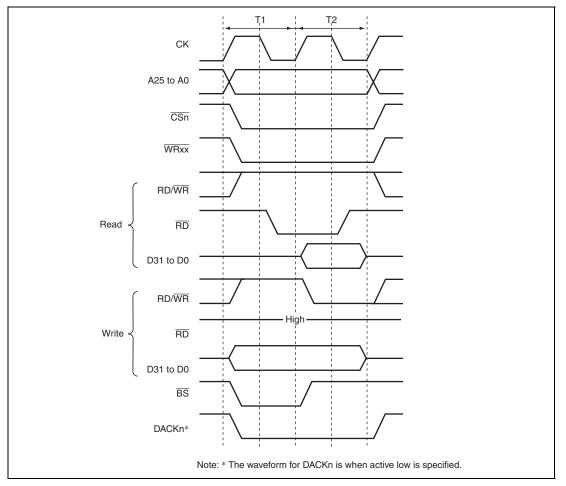
Figure 10.37 Basic Access Timing for SRAM with Byte Selection (BAS = 1)
