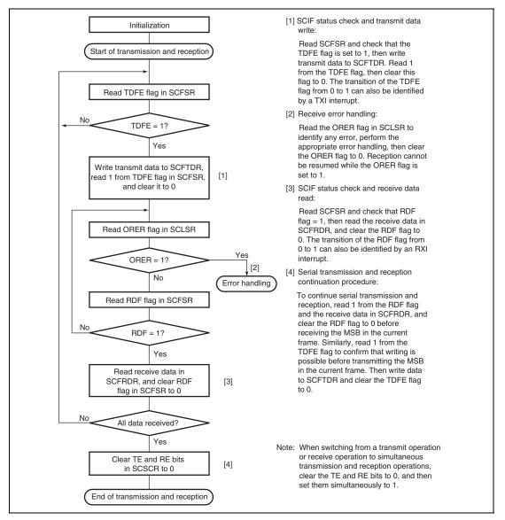
Figure 19.16 Sample Flowchart for Transmitting/Receiving Serial Data
