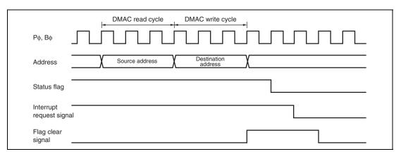
Figure 12.117 Timing for Status Flag Clearing by DTC Activation (Channels 0 to 4)
