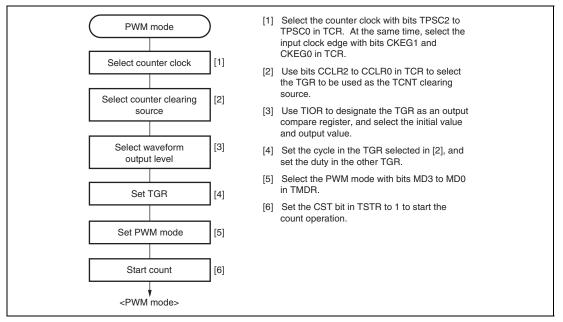
Figure 12.25 Example of PWM Mode Setting Procedure
