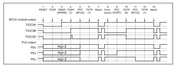
Figure 12.167 Error Occurrence in Reset-Synchronized PWM Mode, **Recovery in Reset-Synchronized PWM Mode**
