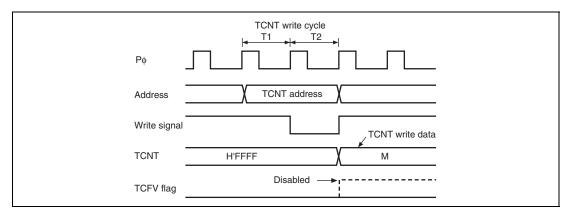
Figure 12.136 Contention between TCNT Write and Overflow
