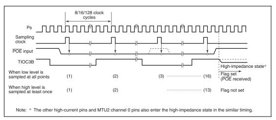
Figure 14.3 Low-Level Detection Operation
