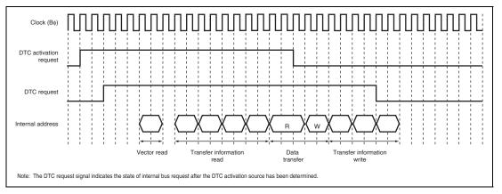
Figure 9.14 Example of DTC Operation Timing: Normal Transfer, Repeat Transfer, DTPR=1 (Activated by On-Chip Peripheral Module;  $I\phi$ :  $B\phi$ :  $P\phi = 1 : 1/2 : 1/2$ ; Data Transferred from On-Chip Peripheral Module to On-Chip RAM (High Speed); **Transfer Information is Written in 3 Cycles)**
