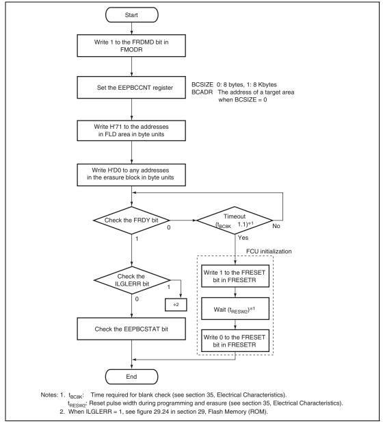
Figure 30.7 Procedure of the FLD Blank Check
