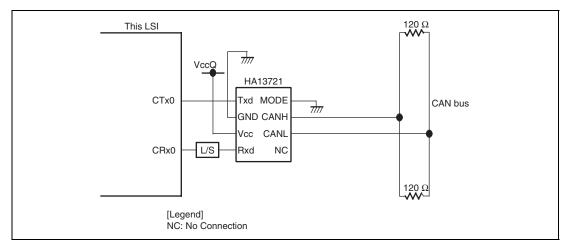
Figure 26.16 High-Speed CAN Interface Using HA13721
