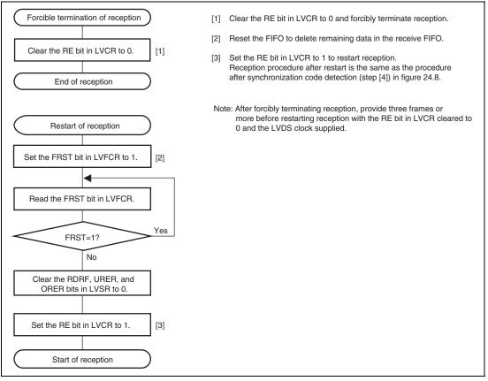
Figure 24.9 Sample Flowchart for Forcibly Terminating and Restarting LVDS Data Reception
