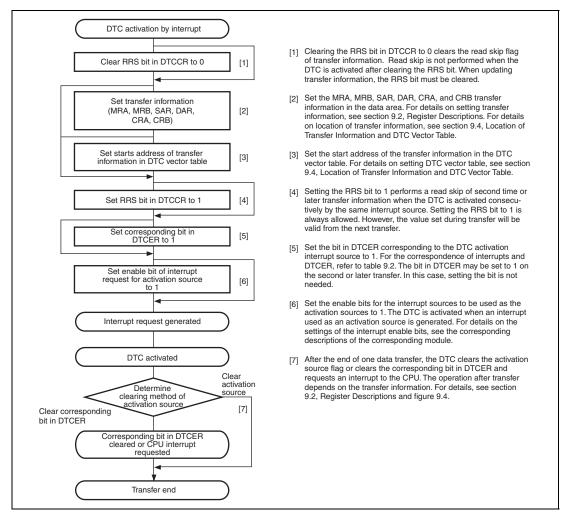
Figure 9.18 DTC Activation by Interrupt
