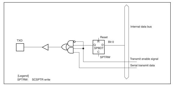
Figure 18.21 SPBDT Bit and TXD Pin
