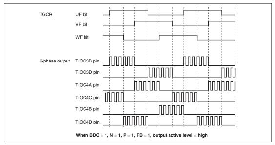
Figure 12.72 Example of Output Phase Switching by Means of UF, VF, and WF Bit Settings (2)
