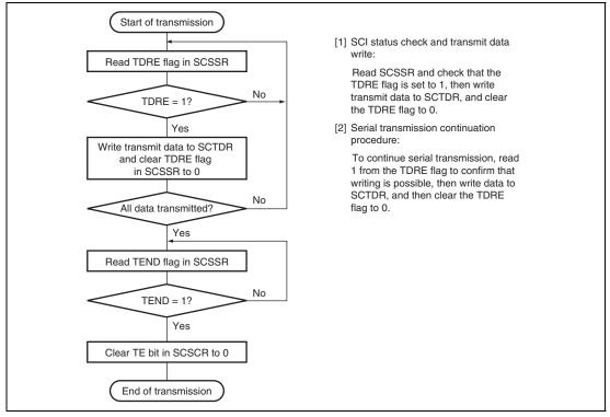
Figure 18.10 Sample Flowchart for Transmitting Serial Data
