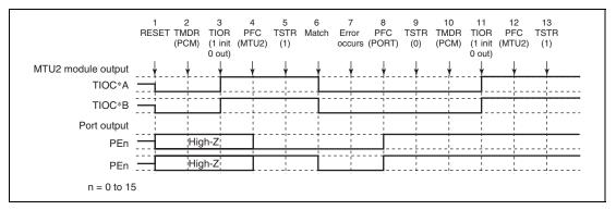
Figure 12.158 Error Occurrence in Phase Counting Mode, Recovery in Phase Counting Mode
