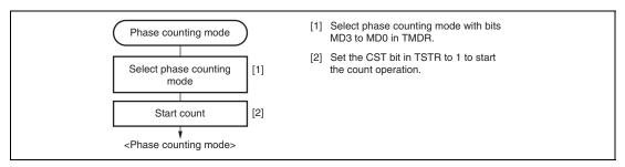
Figure 12.29 Example of Phase Counting Mode Setting Procedure
