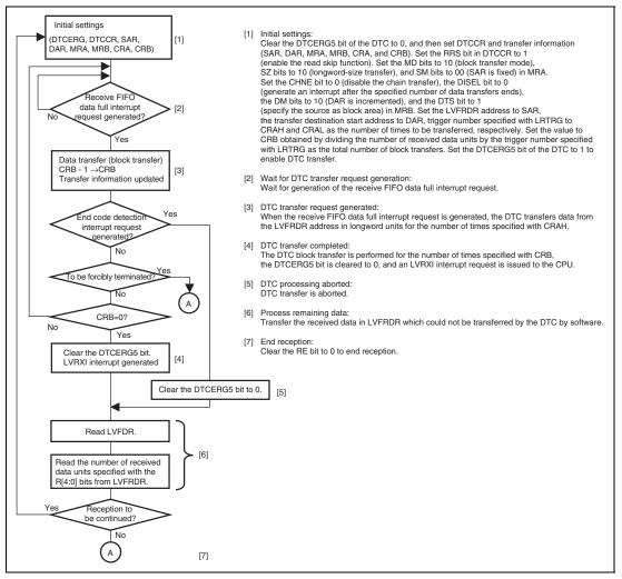
Figure 24.12 Example of Data Transfer from LVDS Receive FIFO Data Register by DTC (1)
