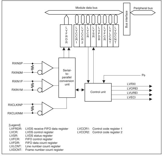
Figure 24.1 Block Diagram of LVDS
