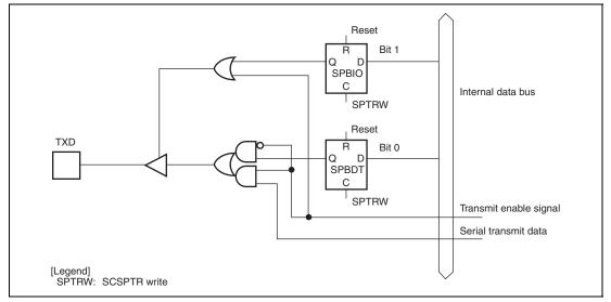
Figure 19.18 SPB2IO Bit, SPB2DT Bit, and TXD Pin
