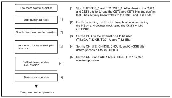
Figure 27.2 Example of Procedure for Setting Two-Phase Counter Operation
