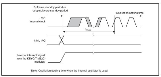
Figure 35.9 Oscillation Settling Time on Return from Standby (Return by an Interrupt)
