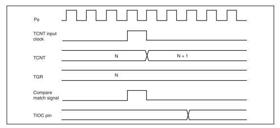
Figure 12.98 Output Compare Output Timing (Complementary PWM Mode/Reset Synchronous PWM Mode)
