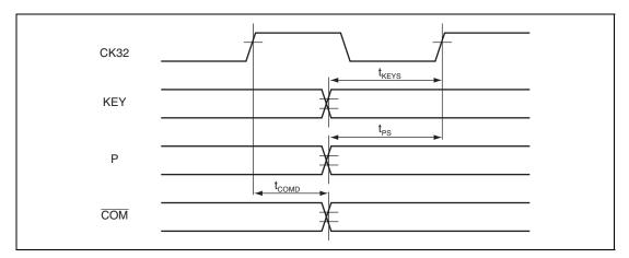
Figure 35.65 KEYC Input/Output Timing
