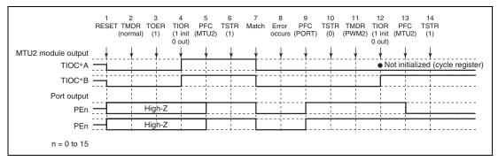
Figure 12.141 Error Occurrence in Normal Mode, Recovery in PWM Mode 2
