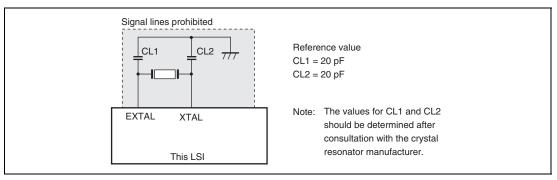
Figure 5.8 Note on Using a Crystal Resonator
