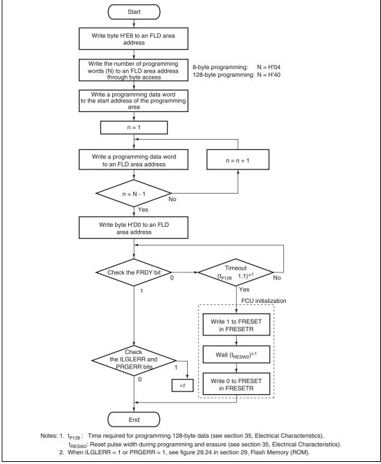
Figure 30.6 Procedure for FLD Programming
