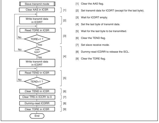
Figure 20.21 Sample Flowchart for Slave Transmit Mode
