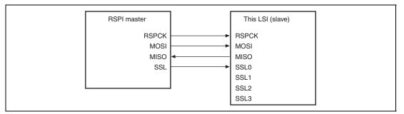
Figure 25.4 Single-Master/Single-Slave Configuration Example (This LSI = Slave)
