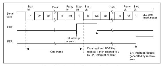
Figure 19.8 Example of SCIF Receive Operation (8-Bit Data with Parity and One Stop Bit when LSB-First Transfer is Selected)
