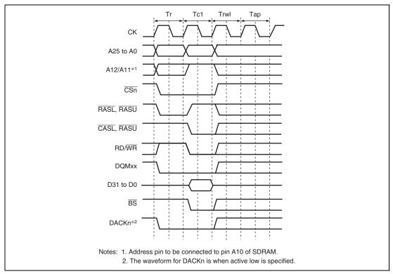
Figure 10.21 Single Write Basic Timing (Auto-Precharge)
