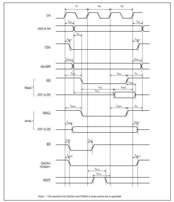
Figure 35.16 Basic Bus Timing for Normal Space (One Software Wait Cycle)
