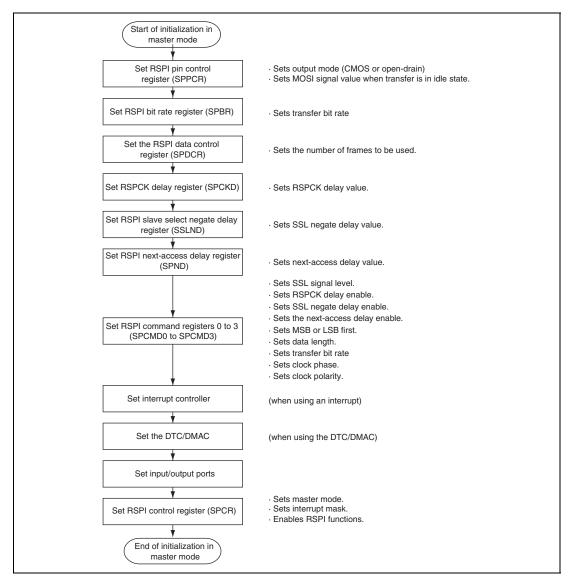
Figure 25.24 Example of Initialization Flowchart in Master Mode
