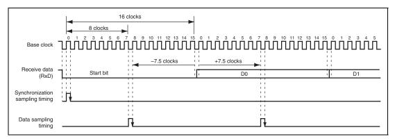
Figure 19.19 Receive Data Sampling Timing in Asynchronous Mode
