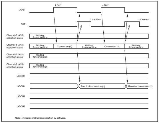
Figure 21.3 Example of A/D Converter Operation in Single Mode (Single-Cycle Scan Mode with AN1 Channel Selected)
