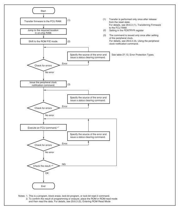
Figure 29.14 Overview of the Flow of Processing for Programming and Erasure
