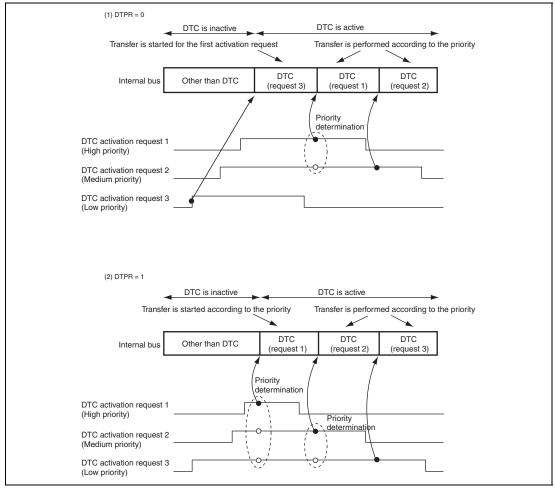
Figure 9.17 Example of DTC Activation According to Priority
