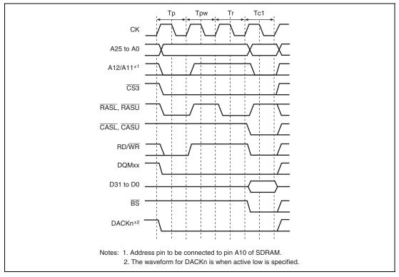
Figure 10.27 Single Write Timing (Bank Active, Different Row Addresses in the Same Bank)
