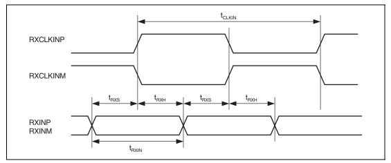
Figure 35.55 LVDS Input Timing
