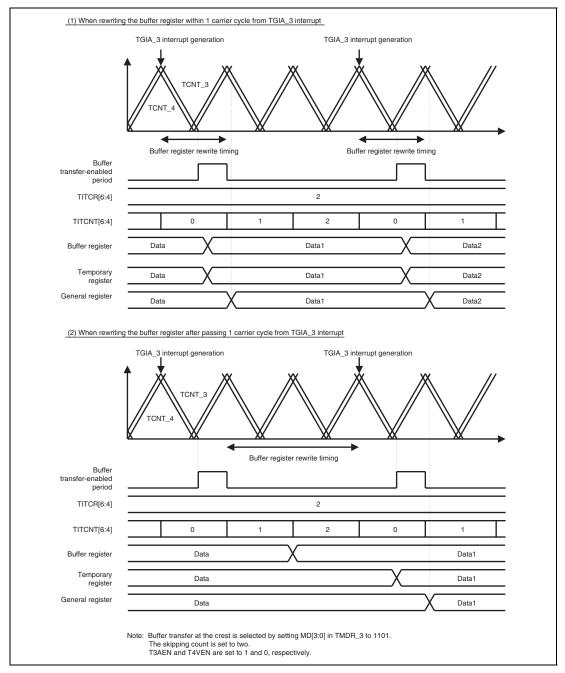
Figure 12.77 Example of Operation when Buffer Transfer is Linked with Interrupt Skipping (BTE1 = 1 and BTE0 = 0)
