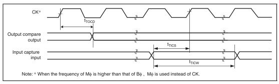
Figure 35.47 MTU2S Input/Output Timing
