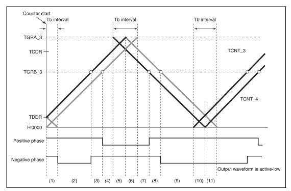
Figure 12.56 Timing for Synchronous Counter Clearing
