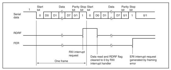
Figure 18.7 Example of SCI Receive Operation (8-Bit Data with Parity and One Stop Bit when LSB-First Transfer is Selected)
