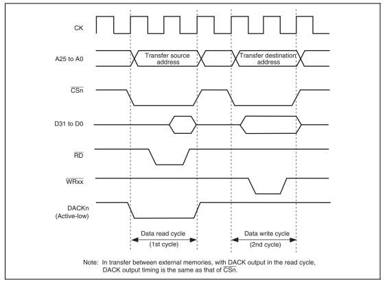
Figure 11.6 Example of DMA Transfer Timing in Dual Mode (Transfer Source: Normal Memory, Transfer Destination: Normal Memory)
