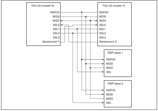
Figure 25.8 Multi-Master/Multi-Slave Configuration Example (This LSI = Master)
