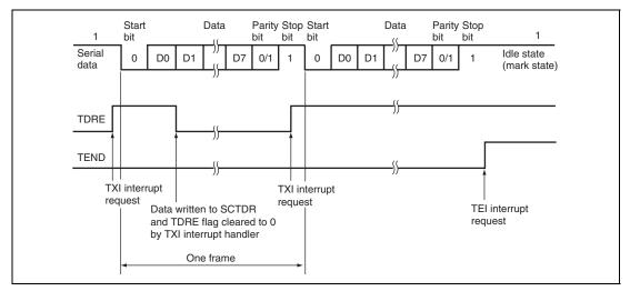
Figure 18.5 Example of Transmission in Asynchronous Mode (8-Bit Data with Parity and One Stop Bit when LSB-First Transfer is Selected)
