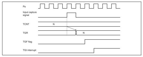
Figure 12.111 TGI Interrupt Timing (Input Capture) (Channels 0 to 4)
