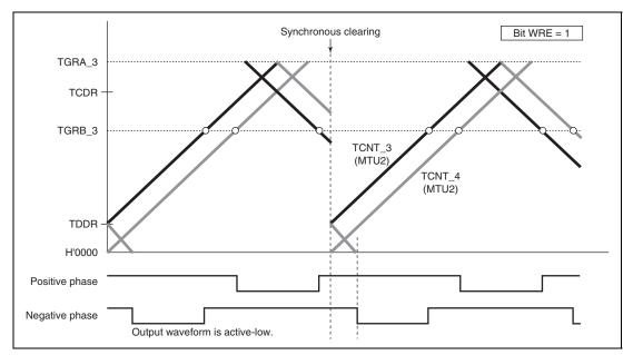
Figure 12.60 Example of Synchronous Clearing in Dead Time during Down-Counting (Timing (8) in Figure 12.56; Bit WRE in TWCR is 1)
