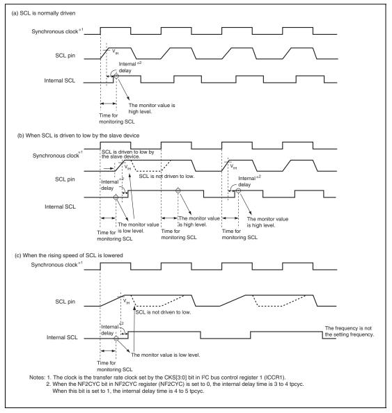
Figure 20.23 Bit Synchronous Circuit Timing
