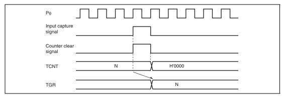
Figure 12.102 Counter Clear Timing (Input Capture) (Channels 0 to 5)
