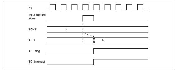
Figure 12.112 TGI Interrupt Timing (Input Capture) (Channel 5)
