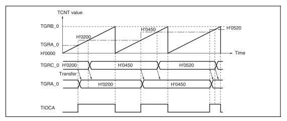
Figure 12.17 Example of Buffer Operation (1)
