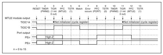
Figure 12.153 Error Occurrence in PWM Mode 2, Recovery in PWM Mode 2
