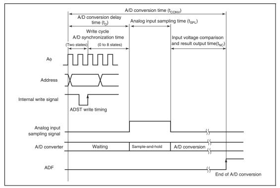
Figure 21.6 A/D Conversion Timing
