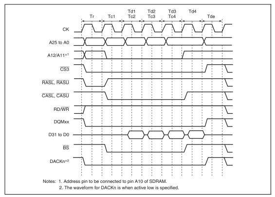
Figure 10.22 Burst Read Timing (Bank Active, Different Bank, CAS Latency 1)
