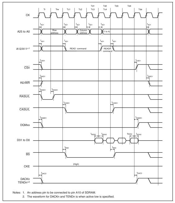
Figure 35.26 Synchronous DRAM Burst Read Bus Cycle (Four Read Cycles) (Auto Precharge, CAS Latency 2, WTRCD = 1 Cycle, WTRP = 0 Cycle)
