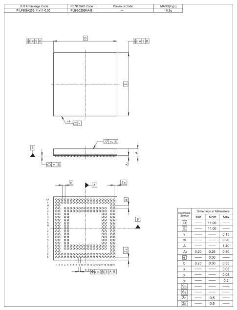
Figure D.1 Package Dimensions (1)
