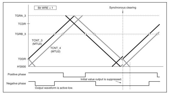
Figure 12.61 Example of Synchronous Clearing in Interval Tb at Trough (Timing (11) in Figure 12.56; Bit WRE in TWCR is 1)
