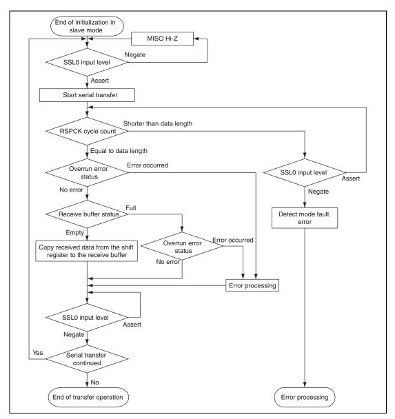
Figure 25.20 Example of Transfer Operation Flowchart in Slave Mode (CPHA = 0)
