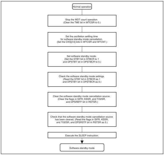
Figure 32.2 Software Standby Mode Setting Flow
