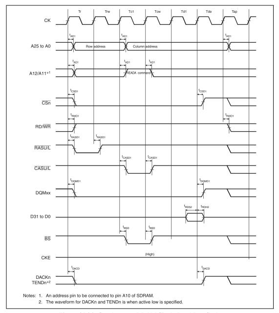
Figure 35.24 Synchronous DRAM Single Read Bus Cycle (Auto Precharge, CAS Latency 2, WTRCD = 1 Cycle, WTRP = 1 Cycle)
