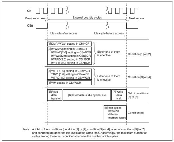
Figure 10.42 Idle Cycle Conditions
