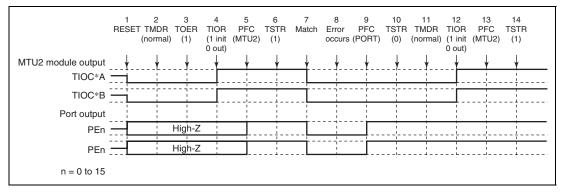
Figure 12.139 Error Occurrence in Normal Mode, Recovery in Normal Mode
