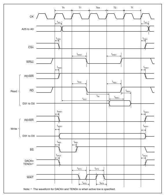
Figure 35.20 Bus Cycle of SRAM with Byte Selection (SW = 1 Cycle, HW = 1 Cycle, One Asynchronous External Wait Cycle, BAS = 0 (Write Cycle UB/LB Control))
