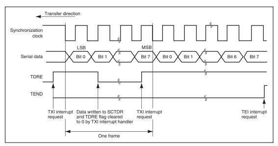
Figure 18.11 Example of SCI Transmit Operation (when LSB-First Transfer is Selected)
