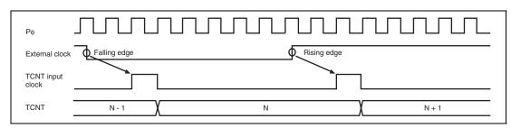
Figure 12.95 Count Timing in External Clock Operation (Channels 0 to 4)
