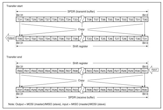
Figure 25.15 LSB First Transfer (32-Bit Data)
