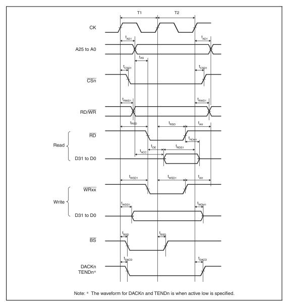
Figure 35.15 Basic Bus Timing for Normal Space (No Wait)
