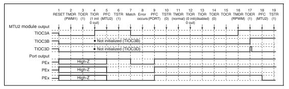
Figure 12.150 Error Occurrence in PWM Mode 1, Recovery in Reset-Synchronized PWM Mode
