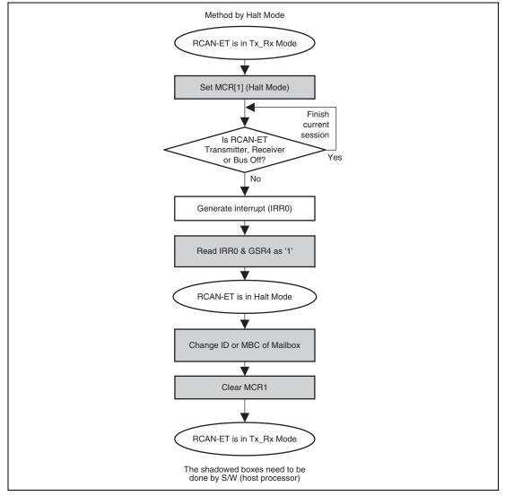
Figure 26.13 Change ID of Receive Box or Change Receive Box to Transmit Box
