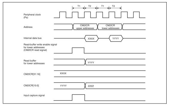
Figure 16.21 Conflict between CM2ICR Reading and Input Capture (when upper address data reading and input capture signal generation occur simultaneously)
