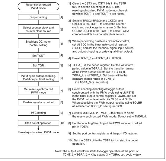
Figure 12.35 Procedure for Selecting Reset-Synchronized PWM Mode
