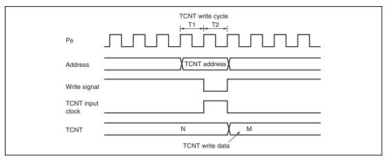
Figure 12.122 Contention between TCNT Write and Increment Operations
