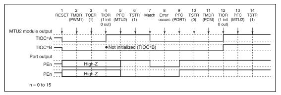
Figure 12.148 Error Occurrence in PWM Mode 1, Recovery in Phase Counting Mode
