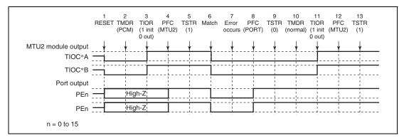
Figure 12.155 Error Occurrence in Phase Counting Mode, Recovery in Normal Mode
