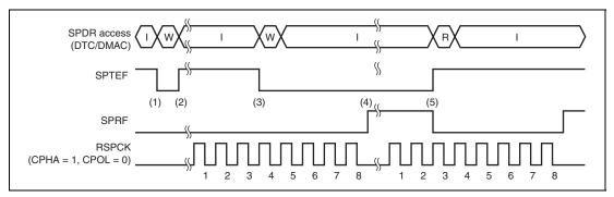
Figure 25.17 SPTEF and SPRF Bit Operation Example
