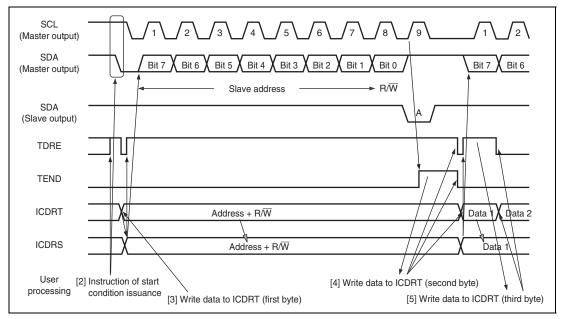
Figure 20.5 Master Transmit Mode Operation Timing (1)
