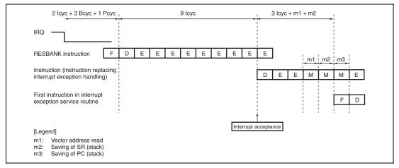
Figure 7.7 Example of Pipeline Operation when Interrupt is Accepted during RESBANK Instruction Execution (Register Banking without Register Bank Overflow)
