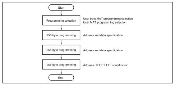
Figure 29.11 Procedure for ROM Programming in Boot Mode
