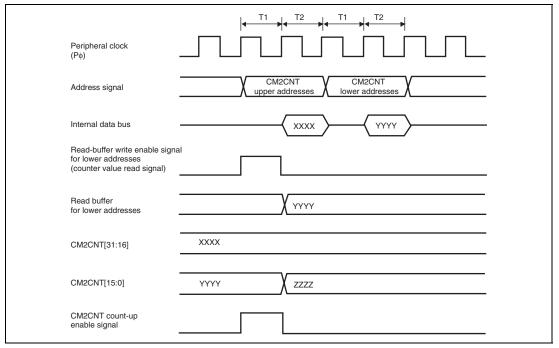
Figure 16.20 Conflict between CM2CNT Reading and Incrementing (when the upper address data reading and incrementing process occur simultaneously)
