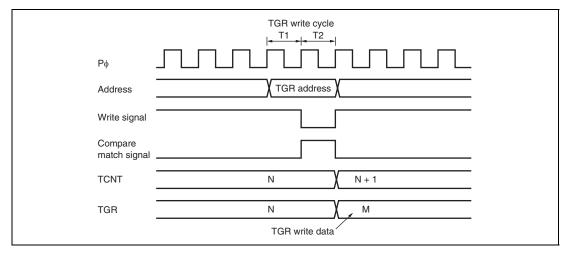
Figure 12.123 Contention between TGR Write and Compare Match
