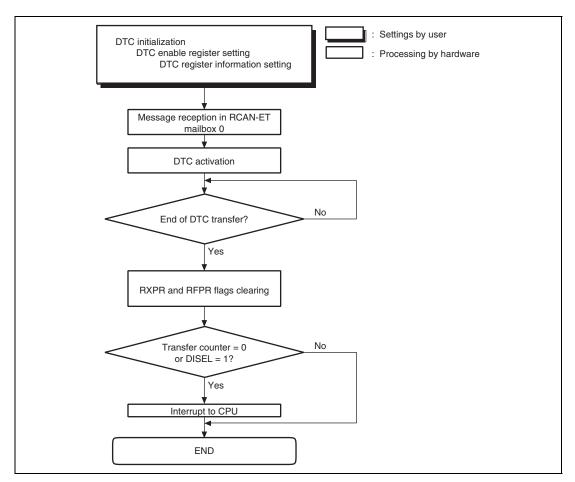
Figure 26.14 DTC Transfer Flowchart
