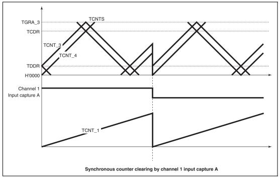
Figure 12.55 Counter Clearing Synchronized with Another Channel
