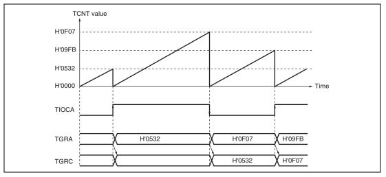
Figure 12.18 Example of Buffer Operation (2)
