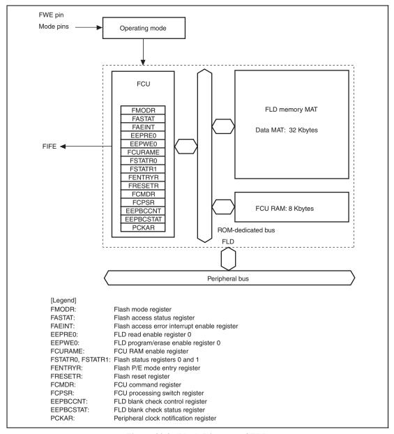
Figure 30.2 Block Diagram of FLD
