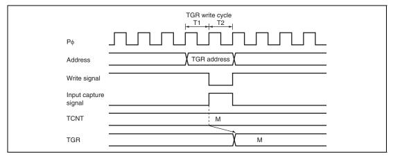
Figure 12.128 Contention between TGR Write and Input Capture (Channels 0 to 4)
