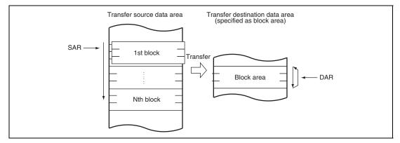
Figure 9.8 Memory Map in Block Transfer Mode (When Transfer Destination is Specified as Block Area)
