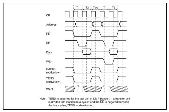
Figure 11.18 BSC Normal Memory Access (No Wait, Idle Cycle 1, Longword Access to 16-Bit Device)
