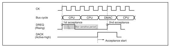
Figure 11.13 Example of DREQ Input Detection in Cycle Steal Mode Edge Detection
