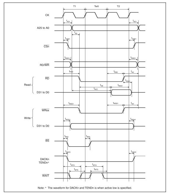
Figure 35.17 Basic Bus Timing for Normal Space (One External Wait Cycle)
