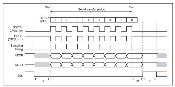
Figure 25.12 RSPI Transfer Format (CPHA = 1)
