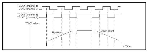
Figure 12.33 Example of Phase Counting Mode 4 Operation
