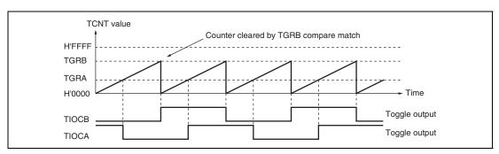
Figure 12.9 Example of Toggle Output Operation
