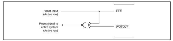
Figure 17.6 Example of System Reset Circuit Using WDTOVF Signal
