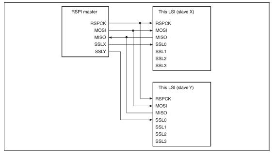
Figure 25.7 Single-Master/Multi-Slave Configuration Example (This LSI = Slave)
