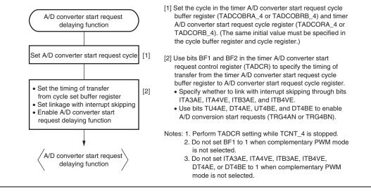
Figure 12.79 Example of Procedure for Specifying A/D Converter Start Request Delaying Function
