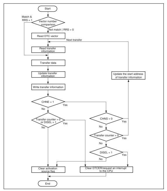
Figure 9.4 Flowchart of DTC Operation
