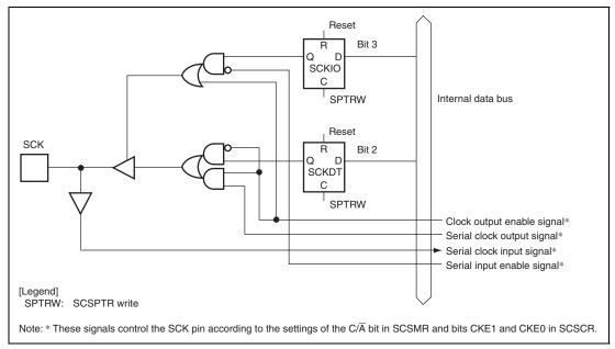
Figure 19.17 SCKIO Bit, SCKDT Bit, and SCK Pin
