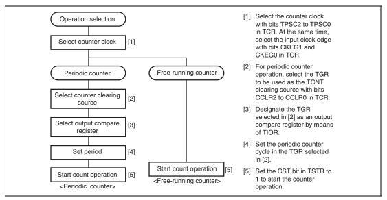
Figure 12.4 Example of Counter Operation Setting Procedure
