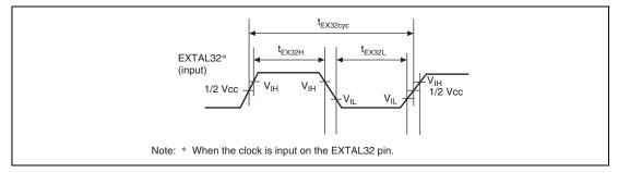
Figure 35.5 EXTAL32 Clock Input Timing
