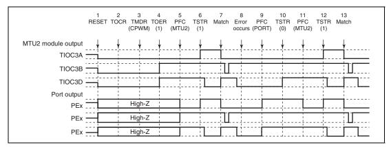
Figure 12.161 Error Occurrence in Complementary PWM Mode, Recovery in Complementary PWM Mode
