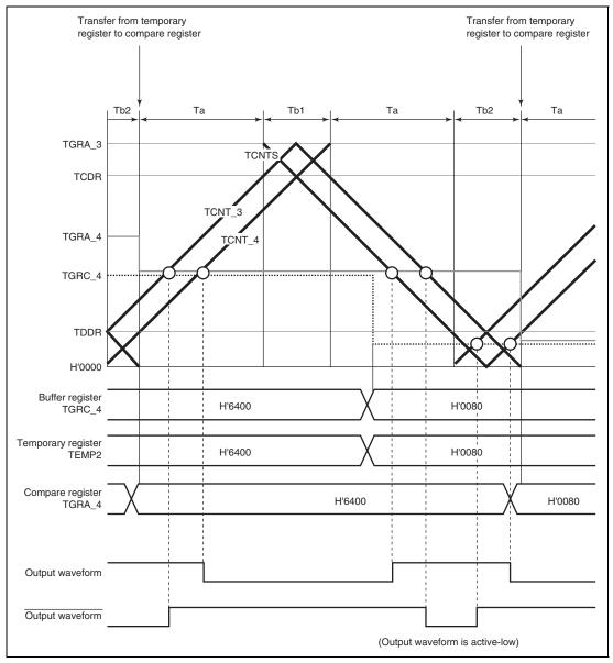
Figure 12.40 Example of Complementary PWM Mode Operation
