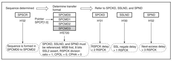
Figure 25.22 Determination Procedure of Serial Transfer Mode in Master Mode
