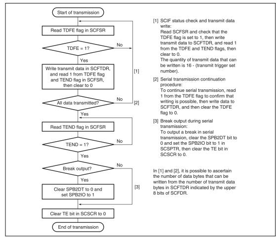
Figure 19.4 Sample Flowchart for Transmitting Serial Data
