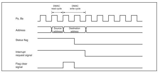
Figure 12.119 Timing for Status Flag Clearing by DMAC Activation
