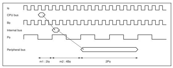
Figure 10.45 Timing of Write Access to On-Chip Peripheral I/O Registers and On-Chip RAM (for Data Retention) When Ιφ;Βφ:Ρφ = 4:4:1
