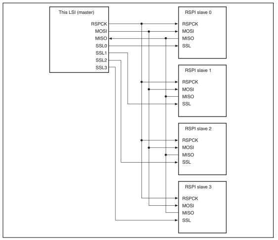
Figure 25.6 Single-Master/Multi-Slave Configuration Example (This LSI = Master)
