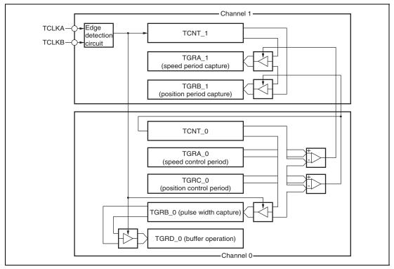
Figure 12.34 Phase Counting Mode Application Example
