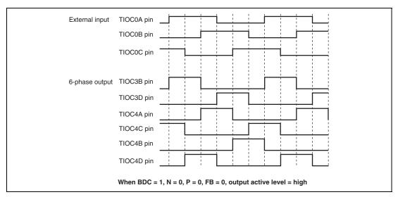
Figure 12.69 Example of Output Phase Switching by External Input (1)
