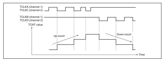
Figure 12.32 Example of Phase Counting Mode 3 Operation
