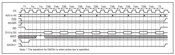
Figure 10.41 Burst ROM Access Timing (Clock Synchronous)
