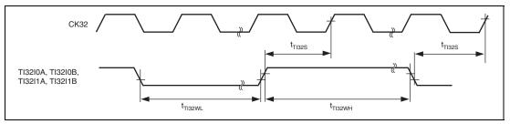
Figure 35.64 TIM32C Input/Output Timing
