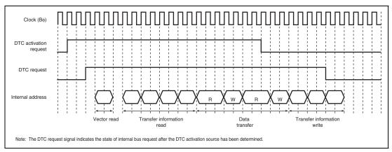
Figure 9.11 Example of DTC Operation Timing: Block Transfer Mode with Block Size = 2 (Activated by On-Chip Peripheral Module;  $I\phi : B\phi : P\phi = 1 : 1/2 : 1/2$ ; Data Transferred from On-Chip Peripheral Module to On-Chip RAM (High Speed); Transfer Information is Written in 3 Cycles)
