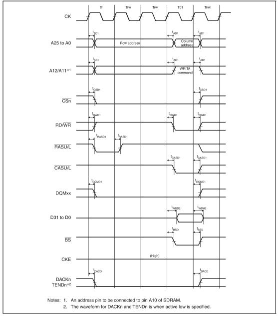
Figure 35.28 Synchronous DRAM Single Write Bus Cycle (Auto Precharge, WTRCD = 2 Cycles, TRWL = 1 Cycle)
