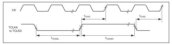
Figure 35.46 MTU2 Clock Input Timing
