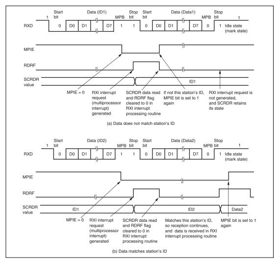
Figure 18.17 Example of SCI Receive Operation (8-Bit Data with Multiprocessor Bit and One Stop Bit when LSB-First Transfer is Selected)
