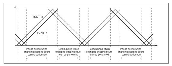
Figure 12.74 Periods during which Interrupt Skipping Count can be Changed
