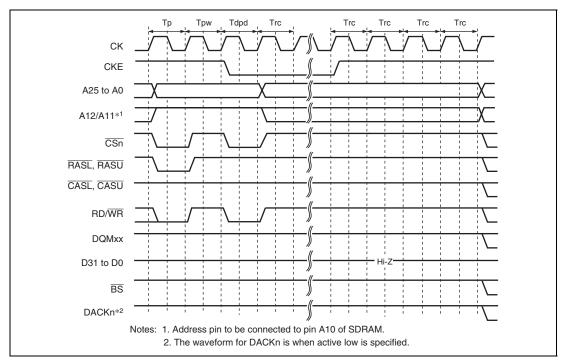
Figure 10.34 Deep Power-Down Mode Transition Timing
