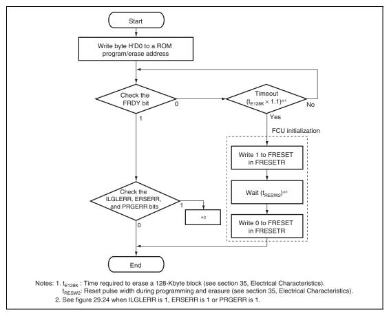
Figure 29.23 Procedure for Resuming Programming or Erasure
