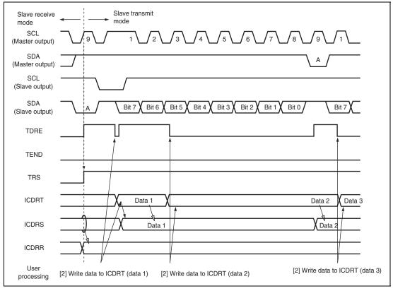
Figure 20.9 Slave Transmit Mode Operation Timing (1)
