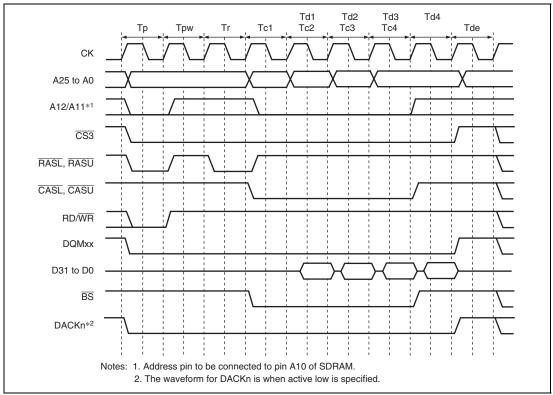
Figure 10.24 Burst Read Timing (Bank Active, Different Row Addresses in the Same Bank, CAS Latency 1)
