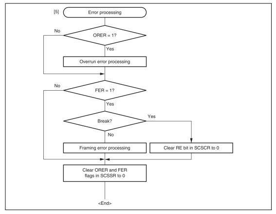
Figure 18.18 Sample Multiprocessor Serial Reception Flowchart (2)
