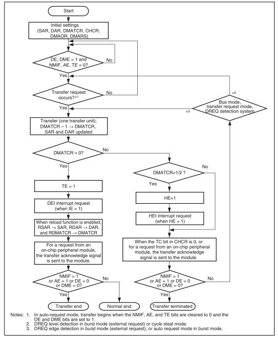
Figure 11.2 DMA Transfer Flowchart
