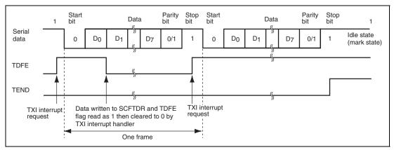
Figure 19.5 Example of Transmit Operation (8-Bit Data with Parity and One Stop Bit when LSB-First Transfer is Selected)
