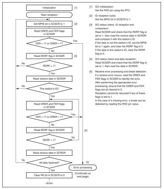
Figure 18.18 Sample Multiprocessor Serial Reception Flowchart (1)
