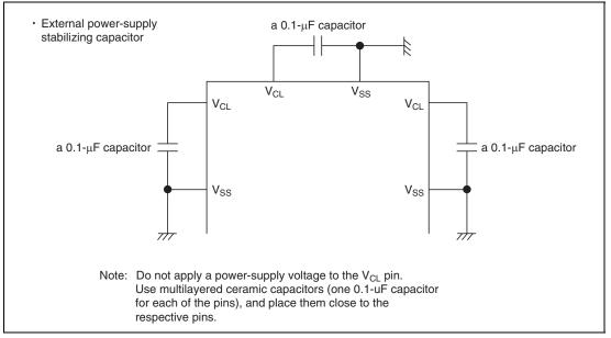
Figure 35.70 Connection of VCL Capacitors
