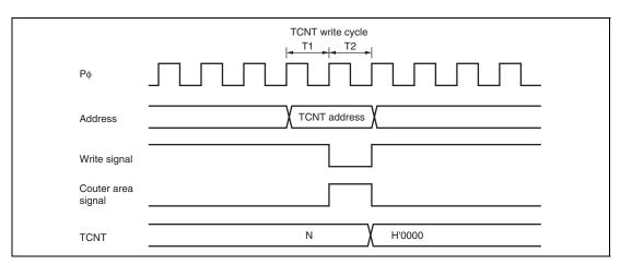
Figure 12.121 Contention between TCNT Write and Clear Operations
