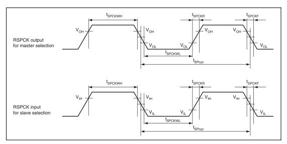
Figure 35.58 RSPI Clock Timing
