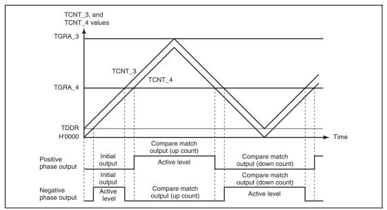
Figure 12.2 Complementary PWM Mode Output Level Example
