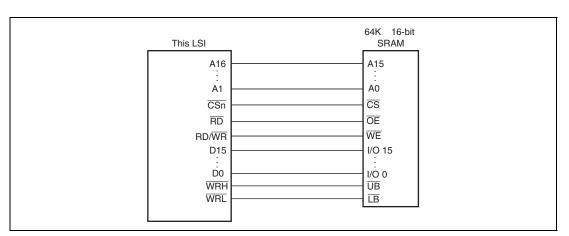
Figure 10.40 Example of Connection with 16-Bit Data-Width SRAM with Byte Selection
