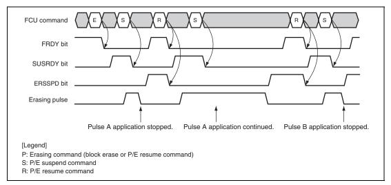
Figure 29.29 Suspending Erasure Processing (Suspension-Priority Mode)
