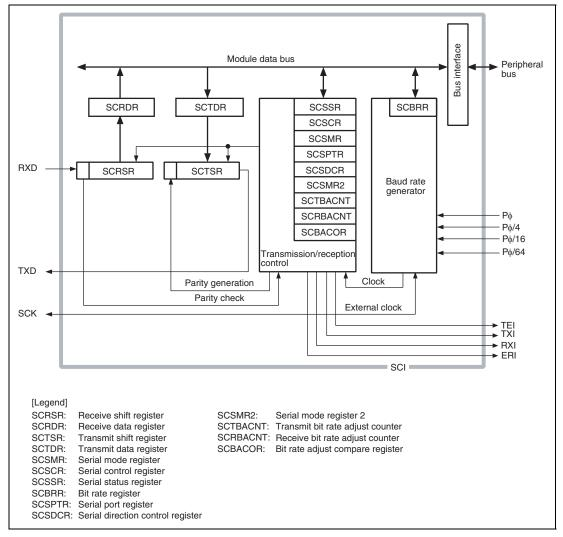
Figure 18.1 Block Diagram of SCI
