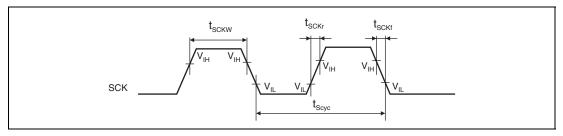
Figure 35.51 SCK Input Clock Timing
