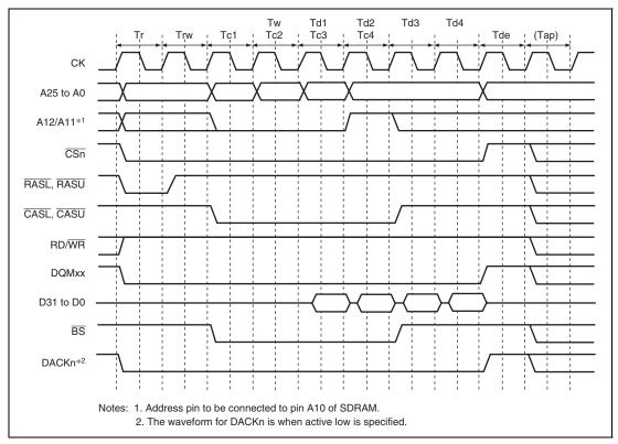
Figure 10.18 Burst Read Wait Specification Timing (CAS Latency 2, WTRCD[1:0] = 1 Cycle, Auto-Precharge)
