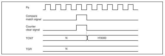
Figure 12.100 Counter Clear Timing (Compare Match) (Channels 0 to 4)
