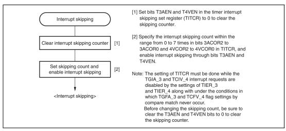
Figure 12.73 Example of Interrupt Skipping Operation Setting Procedure
