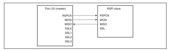
Figure 25.9 Master (Clock Synchronous)/Slave (Clock Synchronous) Configuration Example (This LSI = Master)
