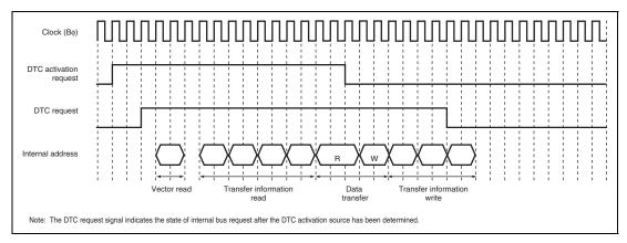
Figure 9.10 Example of DTC Operation Timing: Normal Transfer Mode or Repeat Transfer Mode (Activated by On-Chip Peripheral Module;  $I\phi : B\phi : P\phi = 1 : 1/2 : 1/2$ ; Data Transferred from On-Chip Peripheral Module to On-Chip RAM (High Speed); Transfer Information is Written in 3 Cycles)
