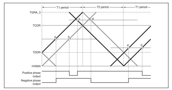
Figure 12.46 Example of Complementary PWM Mode Waveform Output (1)
