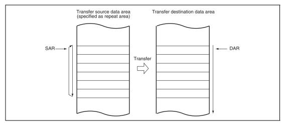
Figure 9.7 Memory Map in Repeat Transfer Mode (When Transfer Source is Specified as Repeat Area)
