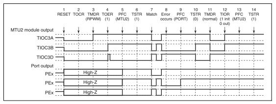
Figure 12.164 Error Occurrence in Reset-Synchronized PWM Mode, Recovery in Normal Mode
