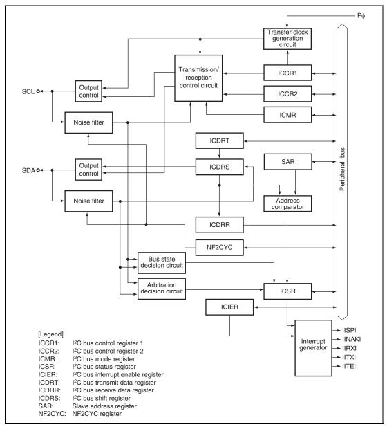
Figure 20.1 Block Diagram of I<sup>2</sup>C Bus Interface 3
