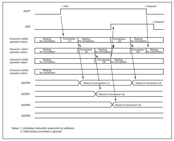
Figure 21.4 Example of A/D Converter Operation in 4-Channel Scan Mode (Continuous Scan Mode with Three Channels AN0 to AN2 Selected)
