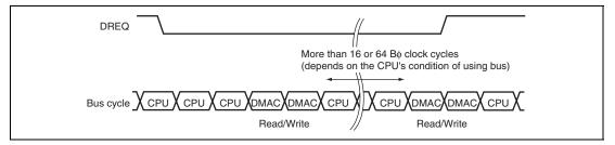
Figure 11.10 Example of DMA Transfer in Cycle-Steal Intermittent Mode (Dual Address, DREQ Low Level Detection)
