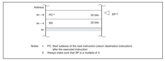
Figure 7.3 Stack after Interrupt Exception Handling
