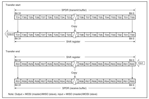
Figure 25.13 MSB First Transfer (32-Bit Data)
