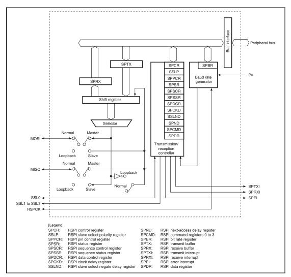
Figure 25.1 Block Diagram of RSPI (for One Channel)
