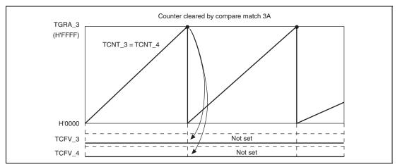
Figure 12.134 Reset Synchronous PWM Mode Overflow Flag
