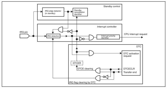
Figure 7.13 Block Diagram of Interrupt Control for an IRQ Signal
