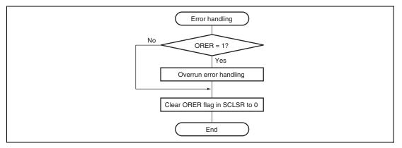
Figure 19.14 Sample Flowchart for Receiving Serial Data (2)
