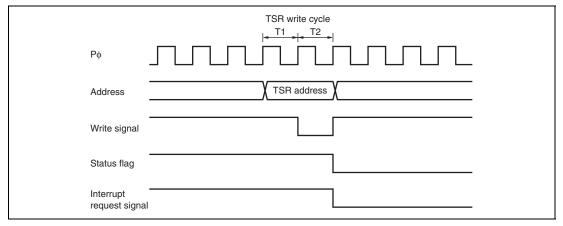
Figure 12.116 Timing for Status Flag Clearing by CPU (Channel 5)
