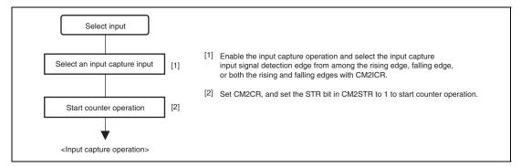
Figure 16.7 Procedure for Setting Input Capture Operation
