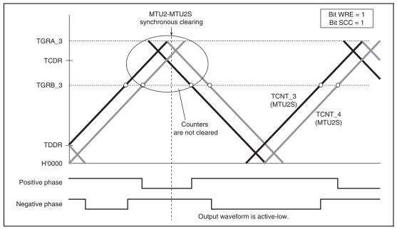
Figure 12.65 Example of Synchronous Clearing in Interval Tb at Crest (Timing (6) in Figure 12.56; Bit WRE is 1 and Bit SCC is 1 in TWCR of MTU2S)
