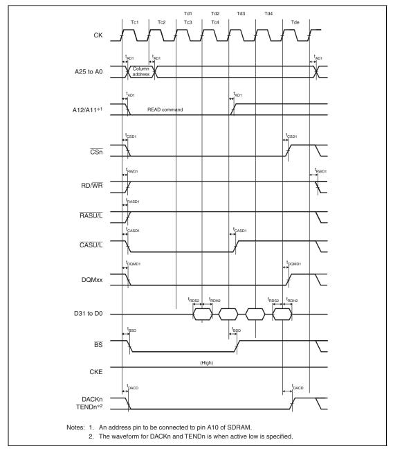
Figure 35.32 Synchronous DRAM Burst Read Bus Cycle (Four Read Cycles) (Bank Active Mode: READ Command, Same Row Address, CAS Latency 2, WTRCD = 0 Cycle)
