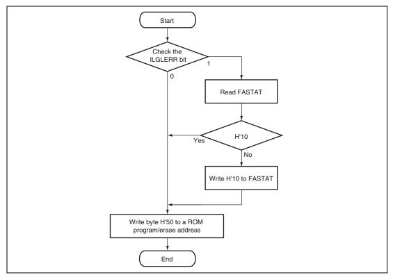
Figure 29.24 Procedure for Clearing Status Register 0
