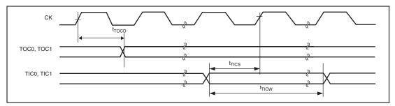
Figure 35.63 CMT2 Input/Output Timing
