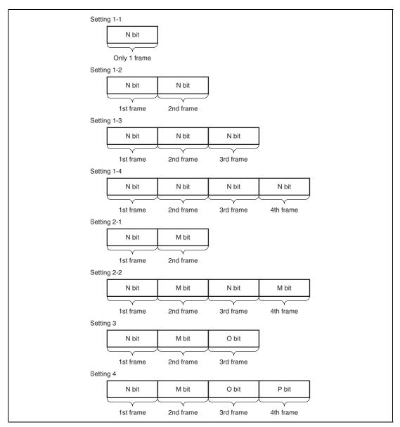
Figure 25.2 Data format for the RSPI
