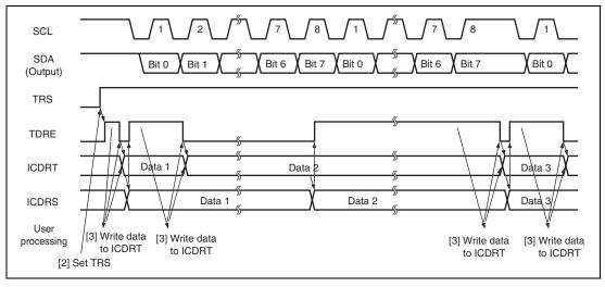
Figure 20.14 Transmit Mode Operation Timing
