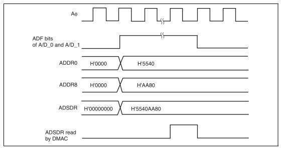
Figure 21.8 Example of ADSDR Access by DMAC (When AD0FCE and AD1FCE in ADSSR are 1)
