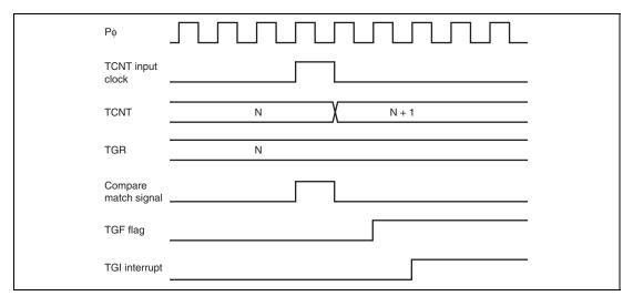
Figure 12.109 TGI Interrupt Timing (Compare Match) (Channels 0 to 4)
