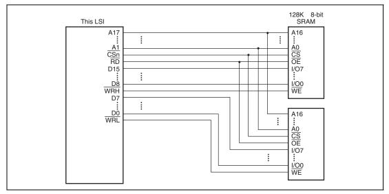
Figure 10.6 Example of 16-Bit Data-Width SRAM Connection
