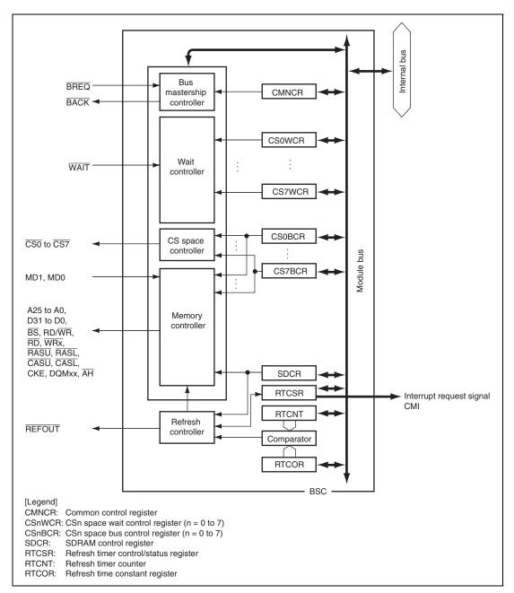
Figure 10.1 Block Diagram of BSC
