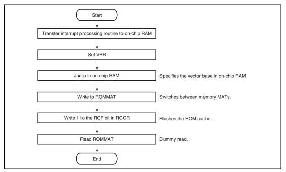
Figure 29.33 Example of MAT Switching Steps
