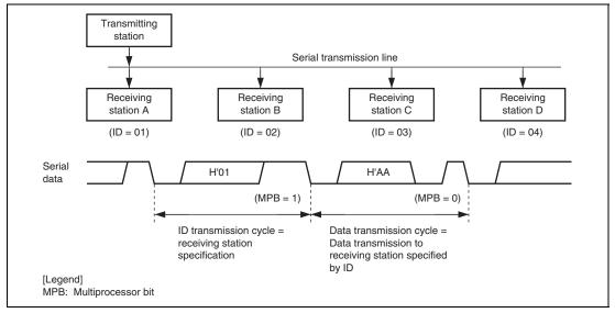
Figure 18.15 Example of Communication Using Multiprocessor Format (Transmission of Data H'AA to Receiving Station A)
