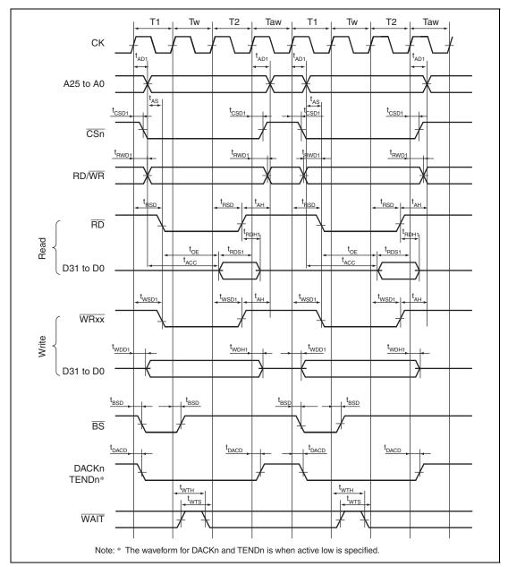
Figure 35.18 Basic Bus Timing for Normal Space (One Software Wait Cycle, External Wait Cycle Valid (WM Bit = 0), No Idle Cycle)
