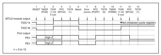
Figure 12.157 Error Occurrence in Phase Counting Mode, Recovery in PWM Mode 2
