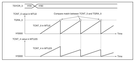
Figure 12.86 (1) Example of MTU2S Counter Clearing Caused by MTU2 Flag Setting Source (1)
