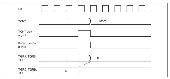
Figure 12.105 Buffer Transfer Timing (when TCNT Cleared)
