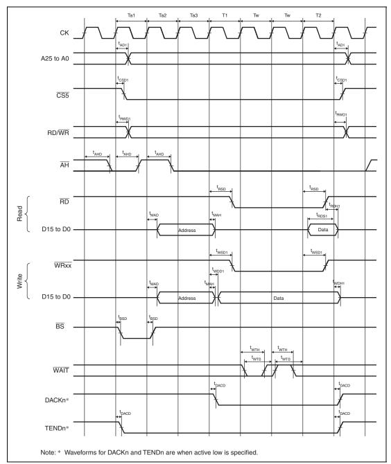
Figure 35.19 MPX-I/O Interface Bus Cycle (Three Address Cycles, One Software Wait Cycle, One External Wait Cycle)
