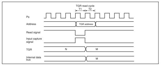
Figure 12.127 Contention between TGR Read and Input Capture (Channel 5)
