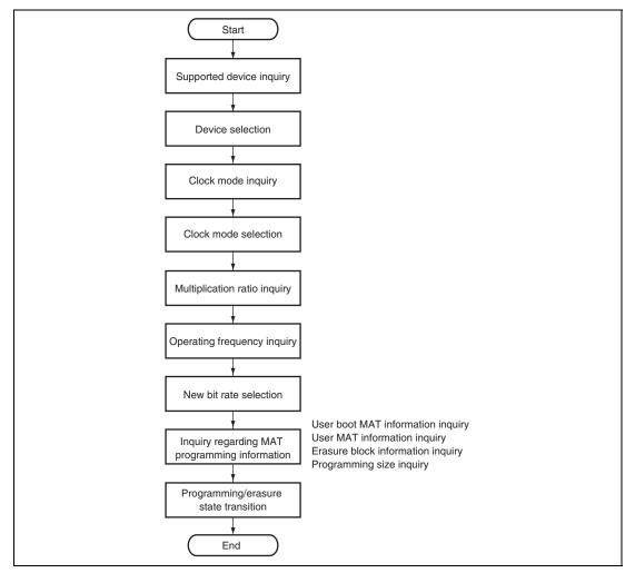
Figure 29.9 Example of Procedure to Use Inquiry/Selection Host Commands
