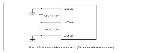
Figure 24.15 Recommended External Circuitry for LVDS Circuit
