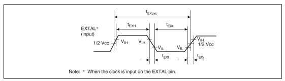
Figure 35.3 EXTAL Clock Input Timing
