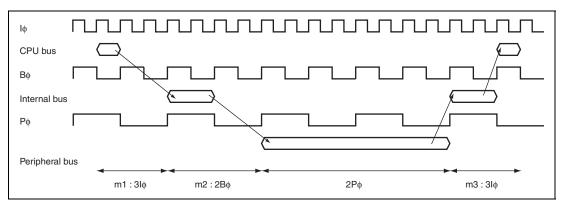
Figure 10.46 Timing of Read Access to On-Chip Peripheral I/O Registers and On-Chip RAM (for Data Retention) When I\(\phi\): P\(\phi\) = 4:2:1
