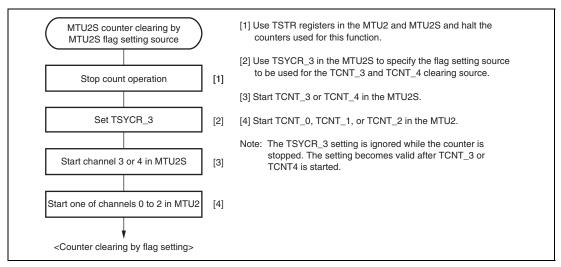
Figure 12.85 Example of Procedure for Specifying MTU2S Counter Clearing by MTU2 Flag Setting Source
