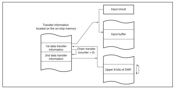
Figure 9.19 Chain Transfer when Transfer Counter = 0
