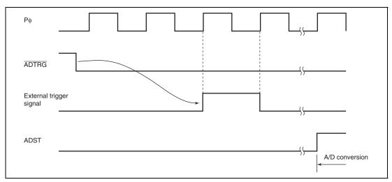
Figure 21.7 External Trigger Input Timing
