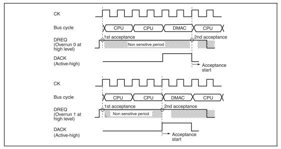
Figure 11.14 Example of DREQ Input Detection in Cycle Steal Mode Level Detection
