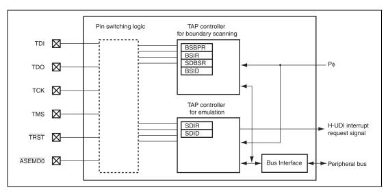
Figure 33.1 Block Diagram of H-UDI
