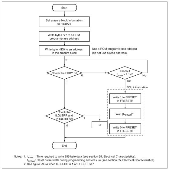
Figure 29.27 Procedure for Writing to the Lock Bit
