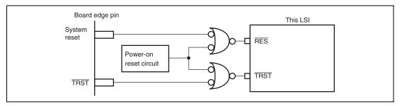
Figure 33.6 Sample Design of Reset-Related Signals Which Do Not Cause Interference
