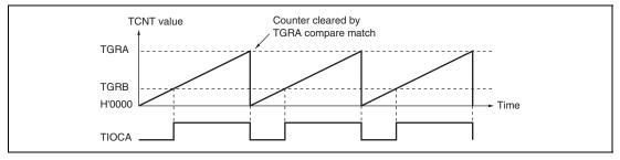
Figure 12.26 Example of PWM Mode Operation (1)
