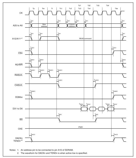
Figure 35.33 Synchronous DRAM Burst Read Bus Cycle (Four Read Cycles) (Bank Active Mode: PRE + ACT + READ Commands, Different Row Addresses, **CAS Latency 2, WTRCD = 0 Cycle)**
