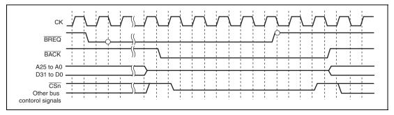
Figure 10.44 Bus Arbitration Timing
