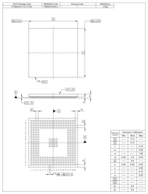
Figure D.2 Package Dimensions (2)
