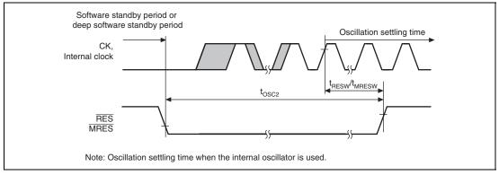
Figure 35.8 Oscillation Settling Time on Return from Standby (Return by Reset)
