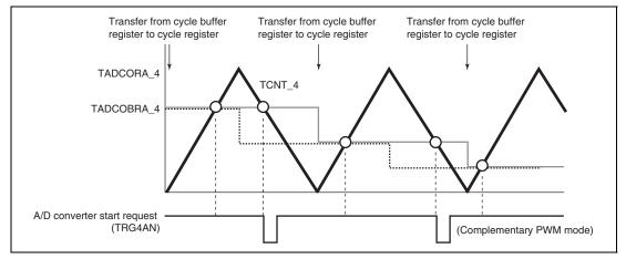
Figure 12.80 Basic Example of A/D Converter Start Request Signal (TRG4AN) Operation
