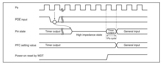
Figure 14.5 Pin State when a Power-On Reset is Issued from the Watchdog Timer
