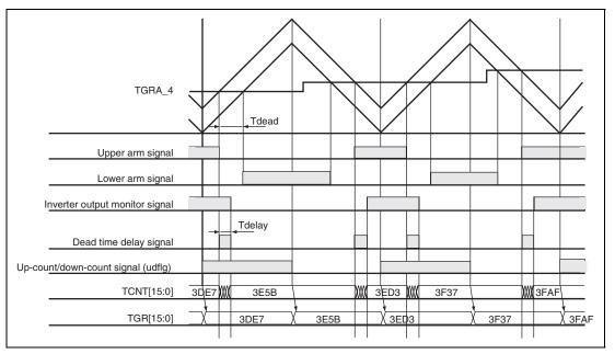
Figure 12.92 TCNT Capturing at Crest and/or Trough in Complementary PWM Operation
