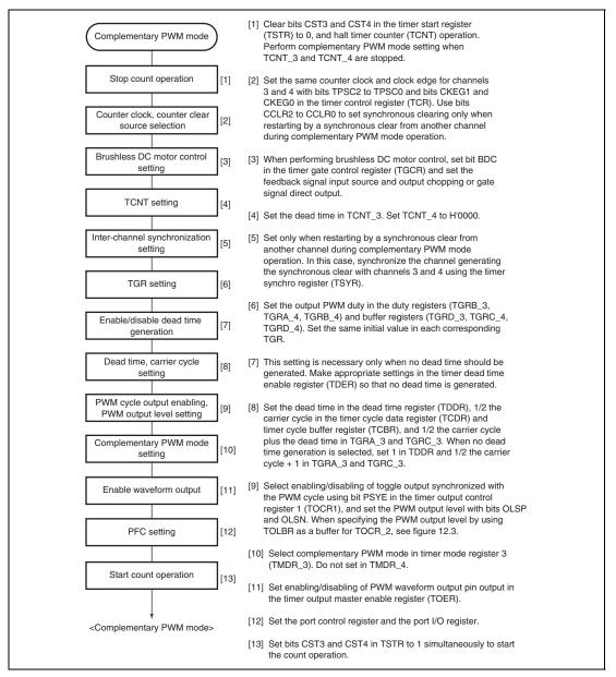
Figure 12.38 Example of Complementary PWM Mode Setting Procedure
