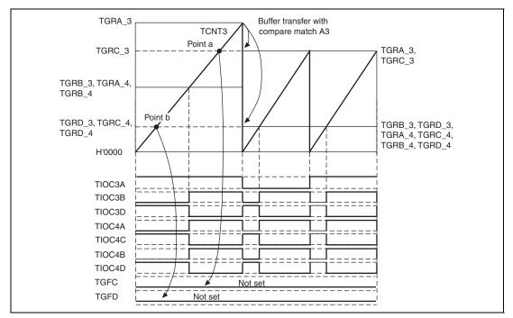
Figure 12.133 Buffer Operation and Compare-Match Flags in Reset Synchronous PWM Mode
