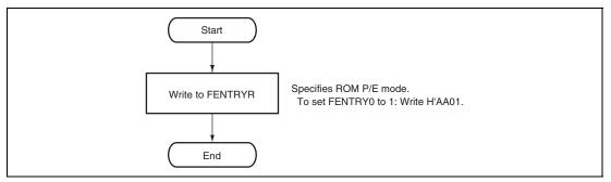
Figure 29.16 Procedure for Transition to ROM P/E Mode
