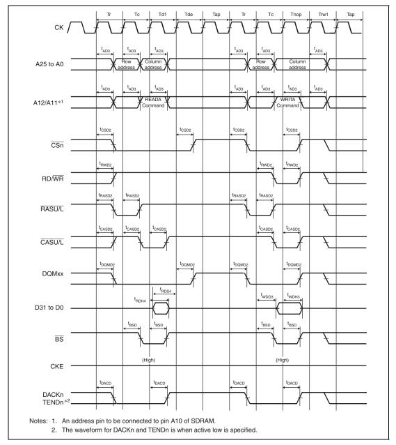
Figure 35.40 Synchronous DRAM Access Timing in Low-Frequency Mode (Auto-Precharge Mode, TRWL = 2 Cycles)
