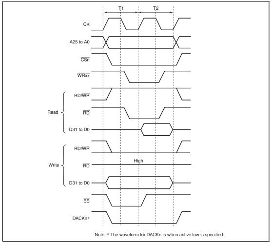
Figure 10.36 Basic Access Timing for SRAM with Byte Selection (BAS = 0)
