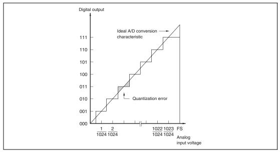
Figure 21.9 Definitions of A/D Conversion Accuracy
