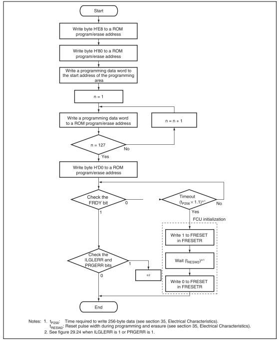
Figure 29.20 Procedure for ROM Programming
