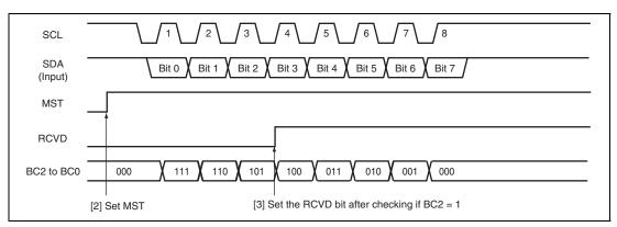
Figure 20.16 Operation Timing for Receiving One Byte (MST = 1)
