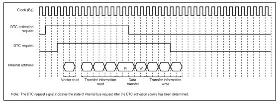
Figure 9.13 Example of DTC Operation Timing:
