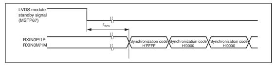
Figure 35.56 LVDS Reception Start Settling Time
