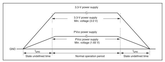
Figure 35.1 Power-On/Power-Off Sequence
