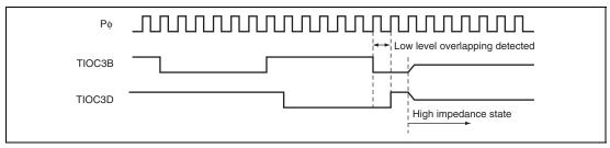
Figure 14.4 Output-Level Compare Operation
