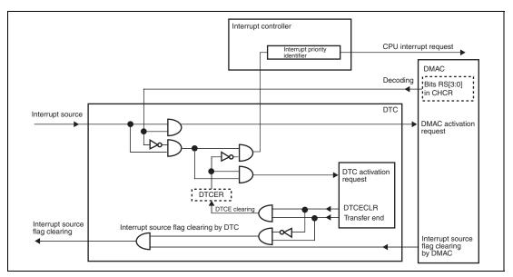
Figure 7.14 Block Diagram of Controlling an On-Chip Peripheral Module Interrupt
