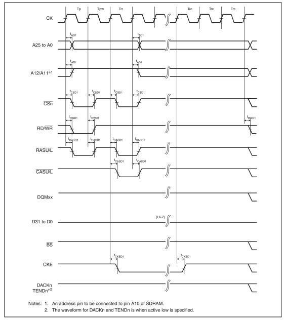
Figure 35.38 Synchronous DRAM Self-Refreshing Timing (WTRP = 1 Cycle)
