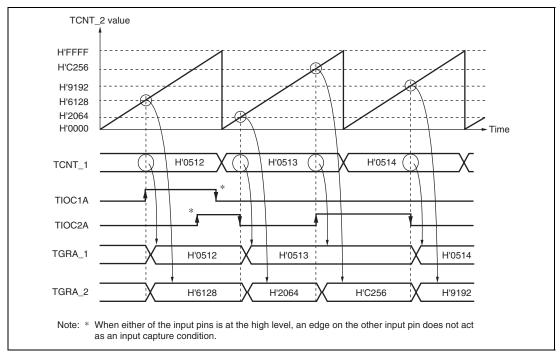
Figure 12.23 Cascaded Operation Example (c)
