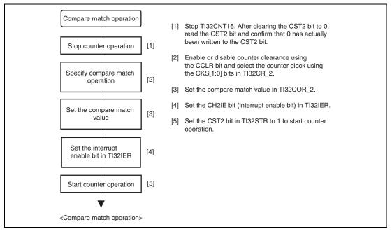
Figure 27.6 Example of Procedure for Setting Compare Match Operation
