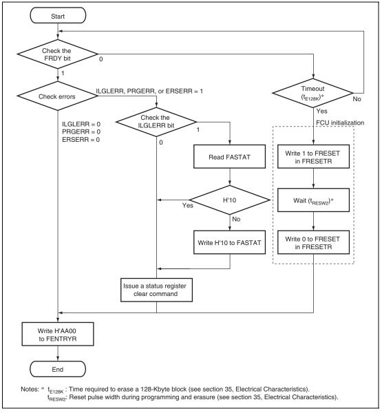
Figure 29.18 Procedure for Transition to ROM Read Mode
