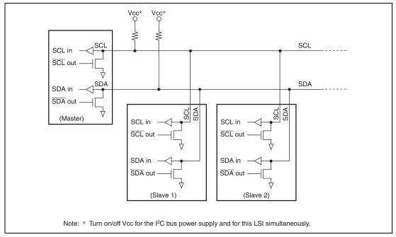
Figure 20.2 External Circuit Connections of I/O Pins
