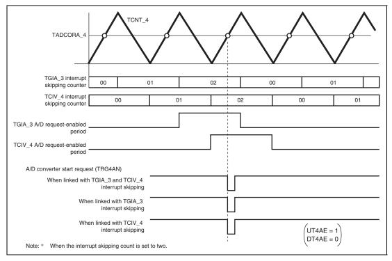
Figure 12.82 Example of A/D Converter Start Request Signal (TRG4AN) Operation Linked with Interrupt Skipping
