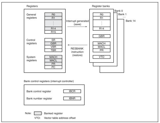
Figure 7.10 Overview of Register Bank Configuration
