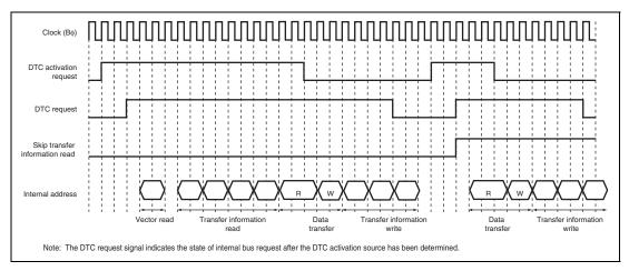
Figure 9.5 Transfer Information Read Skip Timing (Activated by On-Chip Peripheral Module;  $I\phi: B\phi: P\phi=1:1/2:1/2$ ; Data Transferred from On-Chip Peripheral Module to On-Chip RAM (High Speed); Transfer Information is Written in 3 Cycles)
