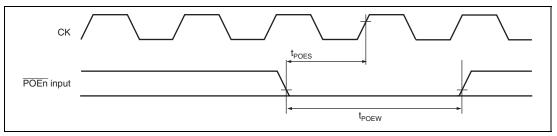
Figure 35.48 POE2 Input Timing
