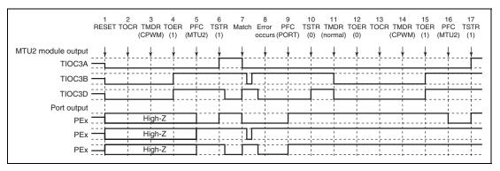
Figure 12.162 Error Occurrence in Complementary PWM Mode, Recovery in Complementary PWM Mode
