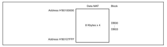
Figure 30.3 Block Configuration of Data MAT
