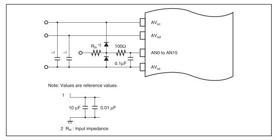
Figure 21.12 Example of Analog Input Pin Protection Circuit
