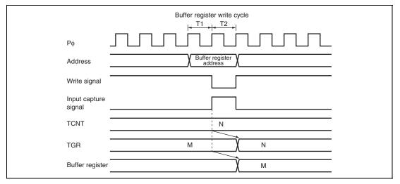
Figure 12.130 Contention between Buffer Register Write and Input Capture
