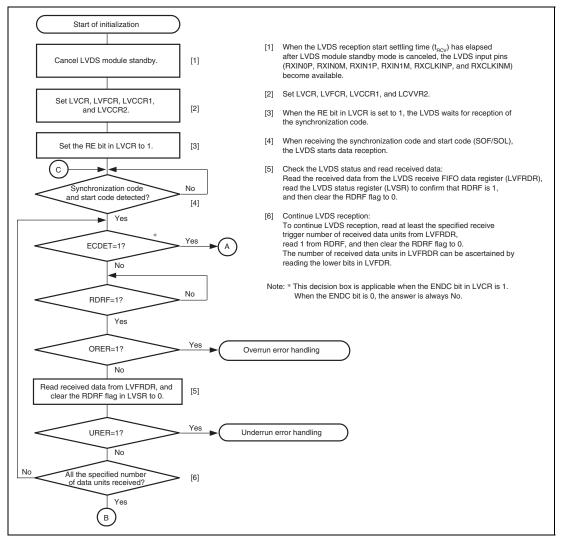
Figure 24.8 Sample Flowchart for Receiving LVDS Data (1)
