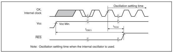
Figure 35.7 Power-On Oscillation Settling Time
