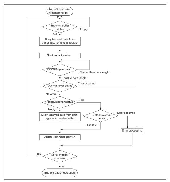
Figure 25.30 Example of Transfer Operation Flowchart in Master Mode
