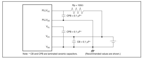
Figure 5.9 Recommended External Circuitry around PLL
