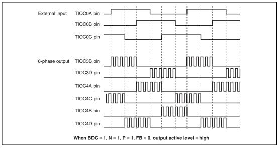
Figure 12.70 Example of Output Phase Switching by External Input (2)
