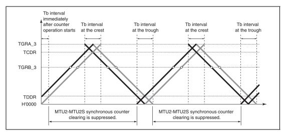
Figure 12.62 MTU2-MTU2S Synchronous Clearing-Suppressed Interval Specified by SCC Bit in TWCR
