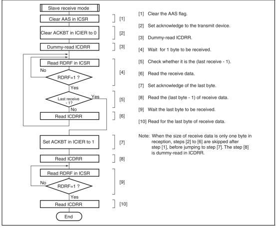
Figure 20.22 Sample Flowchart for Slave Receive Mode
