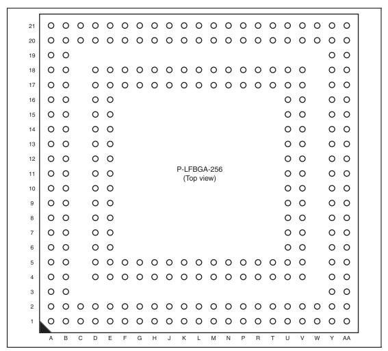
Figure 1.2 Pin Assignment Diagram (P-LFBGA1111-256)
