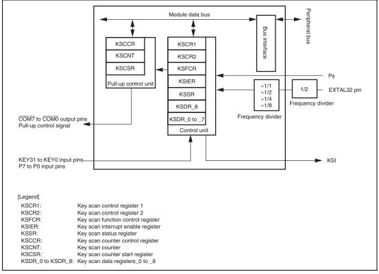
Figure 28.1 Block Diagram of KEYC
