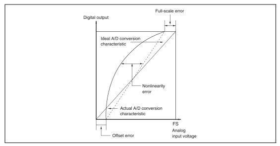
Figure 21.10 Definitions of A/D Conversion Accuracy
