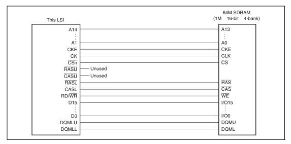
Figure 10.15 Example of 16-Bit Data Width SDRAM Connection (RASU and CASU are Not Used)
