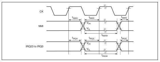
Figure 35.12 Interrupt Signal Input Timing
