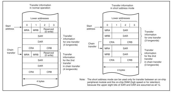
Figure 9.2 Transfer Information on Data Area
