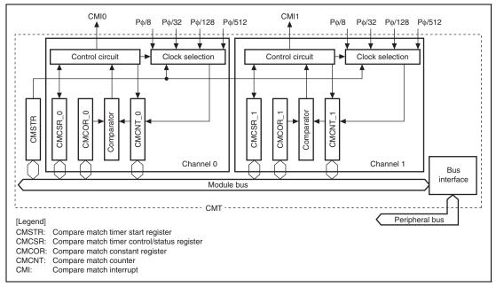
Figure 15.1 Block Diagram of CMT
