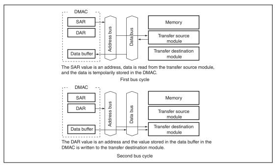
Figure 11.5 Data Flow of Dual Address Mode
