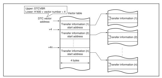
Figure 9.3 Correspondence between DTC Vector Address and Transfer Information
