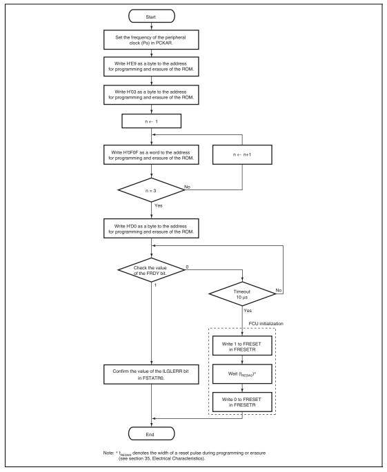
Figure 29.17 Flow for Using the Peripheral Clock Notification Command
