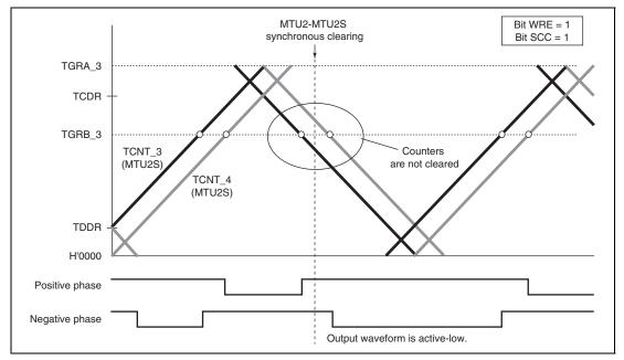
Figure 12.66 Example of Synchronous Clearing in Dead Time during Down-Counting (Timing (8) in Figure 12.56; Bit WRE is 1 and Bit SCC is 1 in TWCR of MTU2S)
