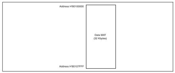
Figure 30.1 Memory MAT Configuration in FLD
