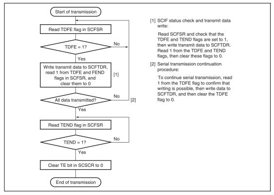
Figure 19.11 Sample Flowchart for Transmitting Serial Data
