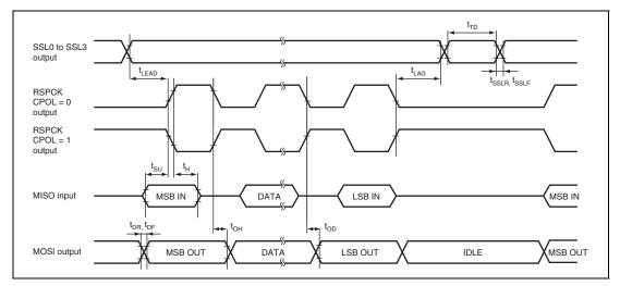
Figure 35.59 RSPI Timing (Master, CPHA = 0)
