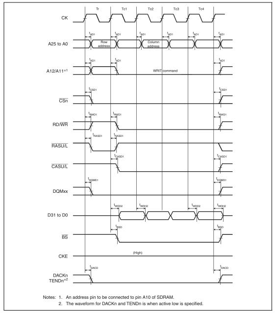
Figure 35.34 Synchronous DRAM Burst Write Bus Cycle (Four Write Cycles) (Bank Active Mode: ACT + WRITE Commands, WTRCD = 0 Cycle, TRWL = 0 Cycle)
