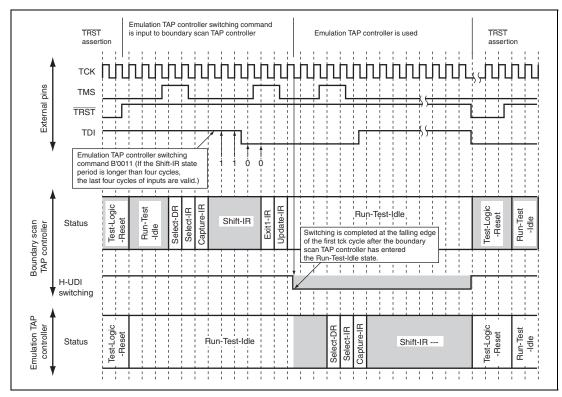
Figure 33.3 Sequence of Switching from Boundary Scan TAP Controller to Emulation TAP Controller
