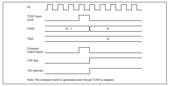
Figure 12.110 TGI Interrupt Timing (Compare Match) (Channel 5)
