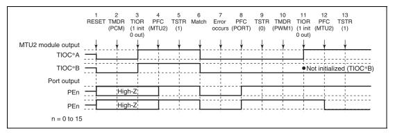
Figure 12.156 Error Occurrence in Phase Counting Mode, Recovery in PWM Mode 1
