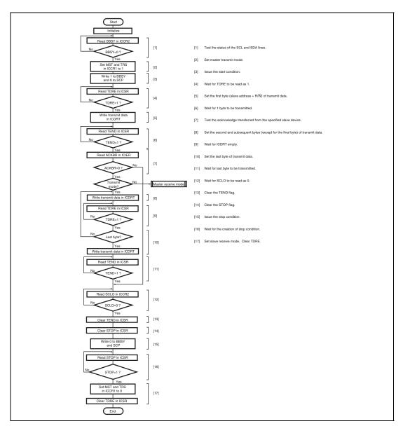
Figure 20.18 Sample Flowchart for Master Transmit Mode
