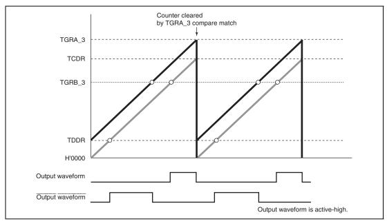
Figure 12.68 Example of Counter Clearing Operation by TGRA\_3 Compare Match
