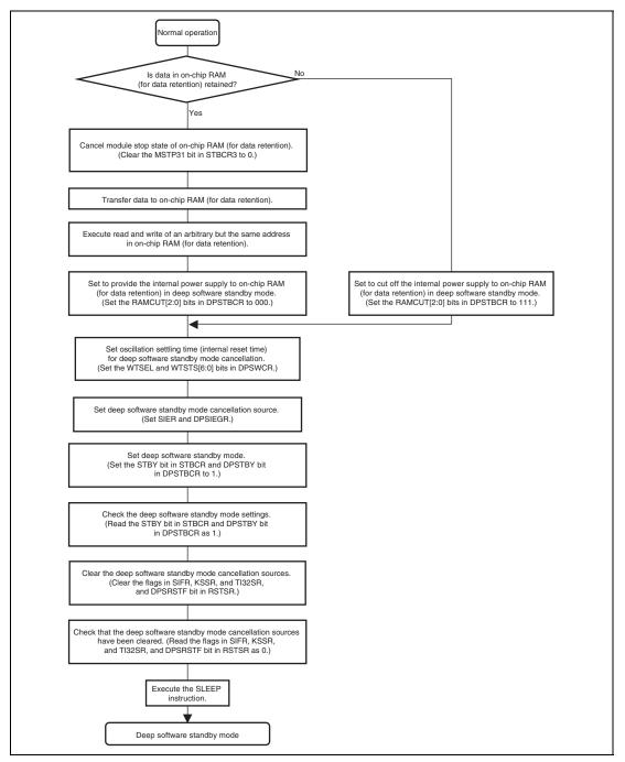
Figure 32.4 Flowchart of Transition to Deep Software Standby Mode
