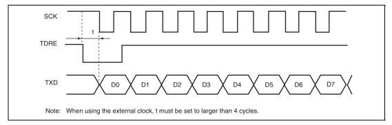
Figure 18.23 Example of Clock Synchronous Transfer Using DMAC or DTC (when LSB-First Transfer is Selected)
