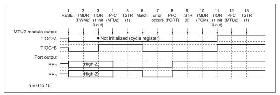
Figure 12.154 Error Occurrence in PWM Mode 2, Recovery in Phase Counting Mode
