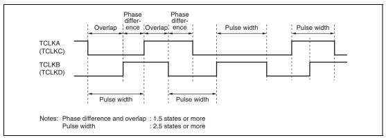
Figure 12.120 Phase Difference, Overlap, and Pulse Width in Phase Counting Mode
