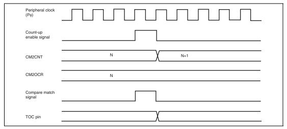
Figure 16.10 Output Compare Output Timing
