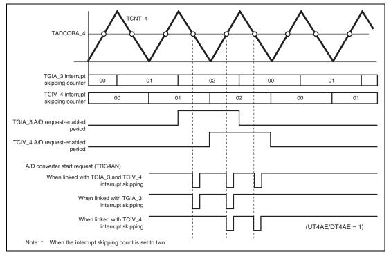
Figure 12.81 Example of A/D Converter Start Request Signal (TRG4AN) Operation Linked with Interrupt Skipping
