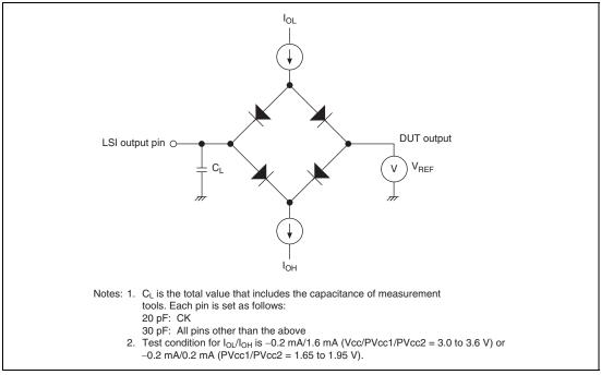
Figure 35.68 Output Load Circuit
