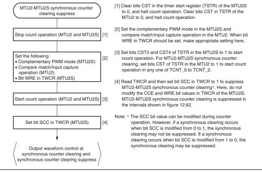
Figure 12.63 Example of Procedure for Suppressing MTU2-MTU2S Synchronous Counter Clearing
