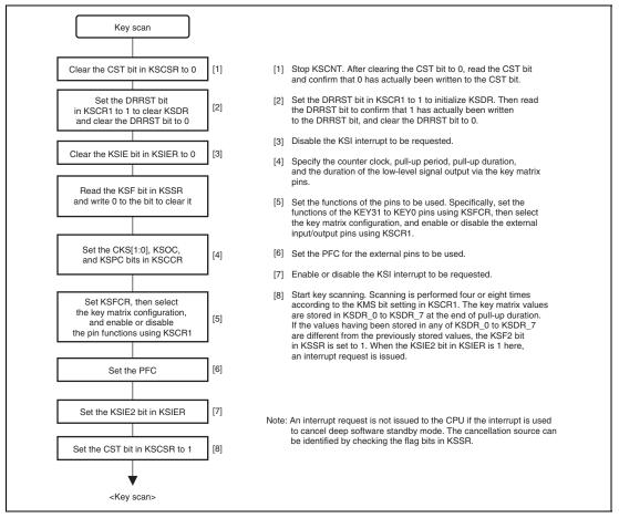
Figure 28.5 Key Scan Setting Procedure
