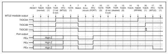
Figure 12.144 Error Occurrence in Normal Mode, Recovery in Reset-Synchronized PWM Mode
