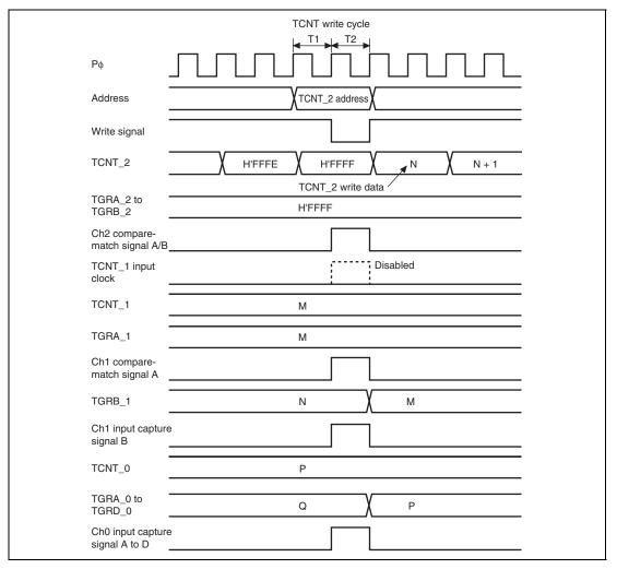
Figure 12.131 TCNT\_2 Write and Overflow/Underflow Contention with Cascade Connection
