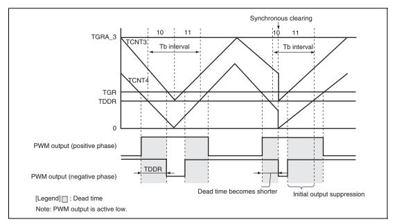
Figure 12.137 Example of Synchronous Clearing for Condition 1
