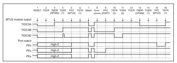
Figure 12.166 Error Occurrence in Reset-Synchronized PWM Mode, Recovery in Complementary PWM Mode
