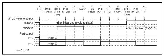
Figure 12.152 Error Occurrence in PWM Mode 2, Recovery in PWM Mode 1
