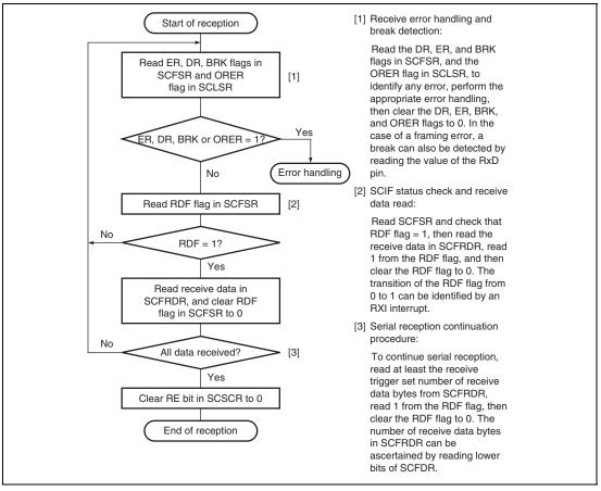
Figure 19.6 Sample Flowchart for Receiving Serial Data (1)
