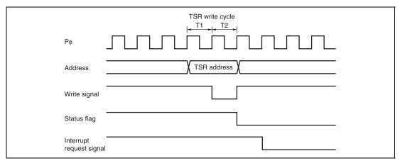
Figure 12.115 Timing for Status Flag Clearing by CPU (Channels 0 to 4)
