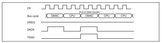
Figure 11.17 Example of DMA Transfer End Signal Timing (Cycle Steal Mode Level Detection)
