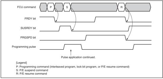
Figure 29.28 Suspending Programming Processing
