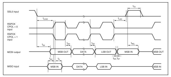
Figure 35.61 RSPI Timing (Slave, CPHA = 0)
