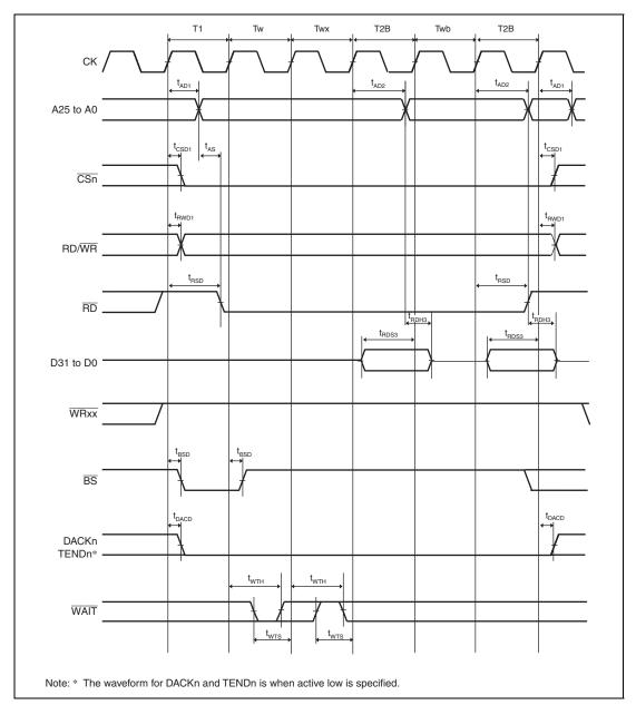
Figure 35.22 Burst ROM Read Cycle (One Software Wait Cycle, One Asynchronous External Burst Wait Cycle, Two-Cycle Burst)
