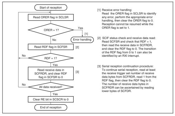
Figure 19.13 Sample Flowchart for Receiving Serial Data (1)
