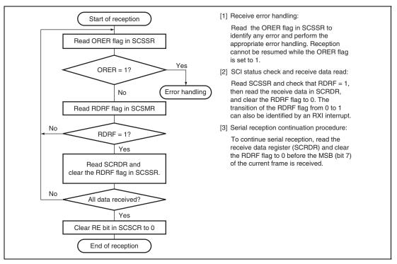
Figure 18.12 Sample Flowchart for Receiving Serial Data (1)
