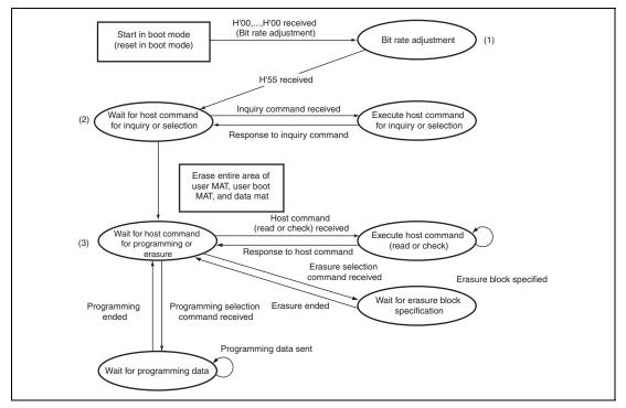
Figure 29.6 State Transition in Boot Mode
