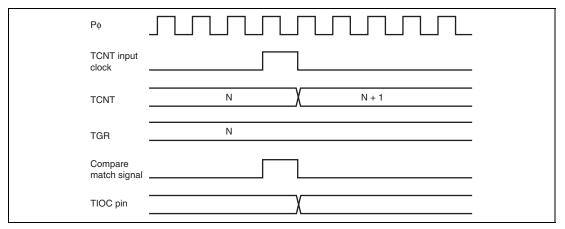
Figure 12.97 Output Compare Output Timing (Normal Mode/PWM Mode)
