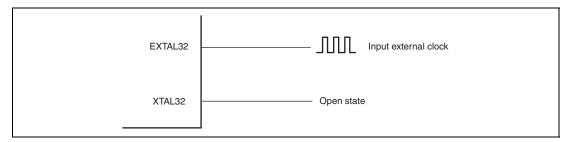
Figure 5.6 Example of Connecting an External Clock
