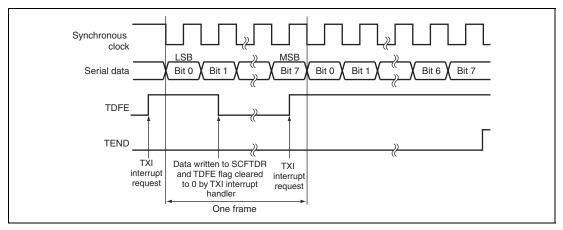
Figure 19.12 Example of SCIF Transmit Operation (when LSB-First Transfer is Selected)
