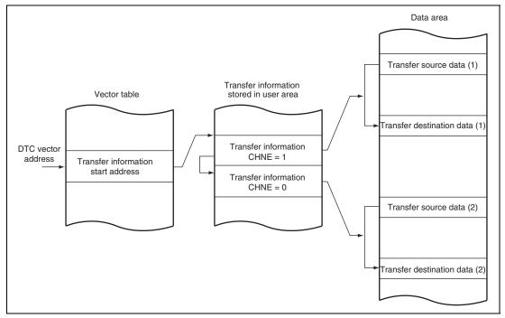
Figure 9.9 Operation of Chain Transfer
