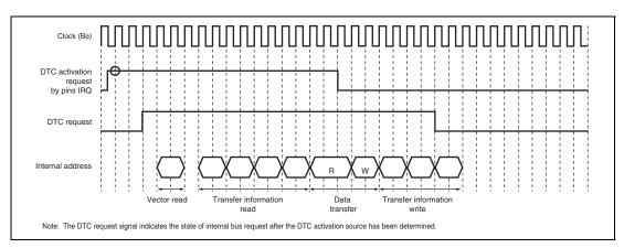
Figure 9.15 Example of DTC Operation Timing: Normal Transfer, Repeat Transfer, (Activated by IRQ;  $I\phi$ :  $B\phi$ :  $P\phi = 1: 1/2: 1/2$ ; Data Transferred from On-Chip Peripheral Module to On-Chip RAM (High Speed); **Transfer Information is Written in 3 Cycles)**
