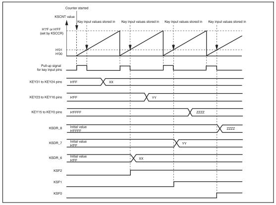
Figure 28.2 Example of Key Input Operation (32-Key Input)
