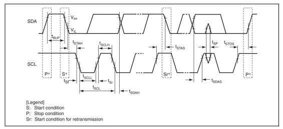
Figure 35.54 IIC3 Input/Output Timing
