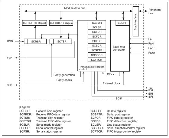
Figure 19.1 Block Diagram of SCIF
