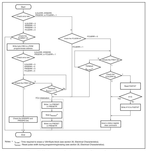
Figure 29.22 Procedure for Programming/Erasure Suspension
