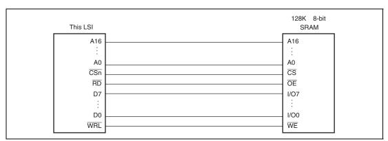
Figure 10.7 Example of 8-Bit Data-Width SRAM Connection
