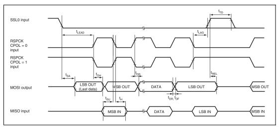
Figure 35.62 RSPI Timing (Slave, CPHA = 1)
