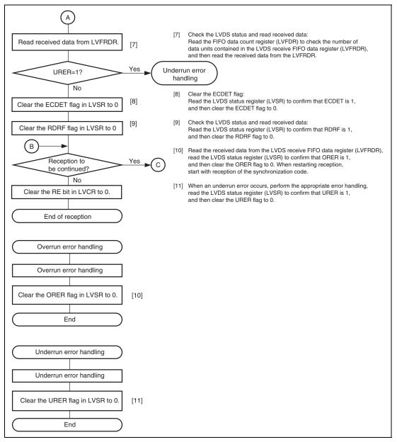
Figure 24.8 Sample Flowchart for Receiving LVDS Data (2)
