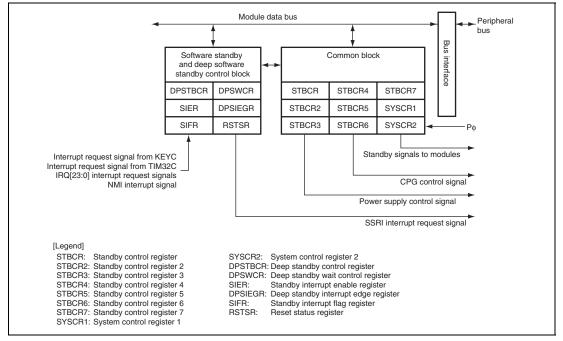
Figure 32.1 Power-Down Mode Block Diagram
