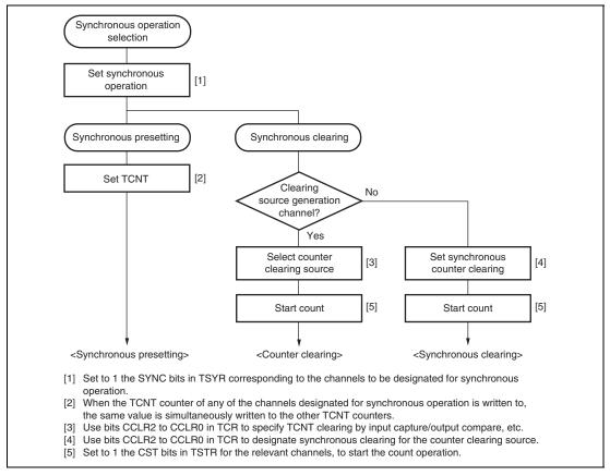
Figure 12.12 Example of Synchronous Operation Setting Procedure
