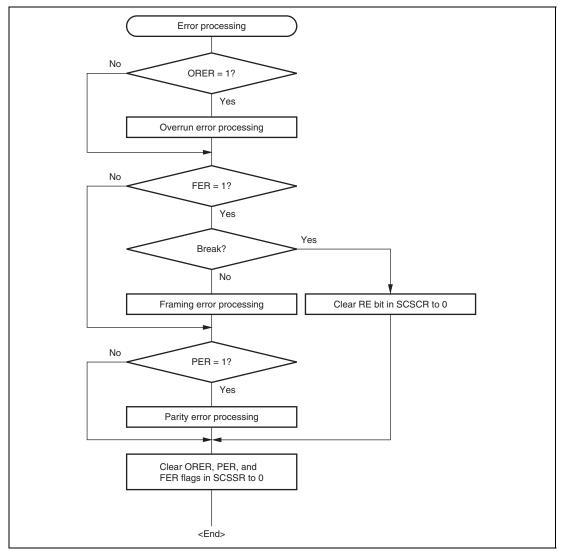
Figure 18.6 Sample Flowchart for Receiving Serial Data (2)
