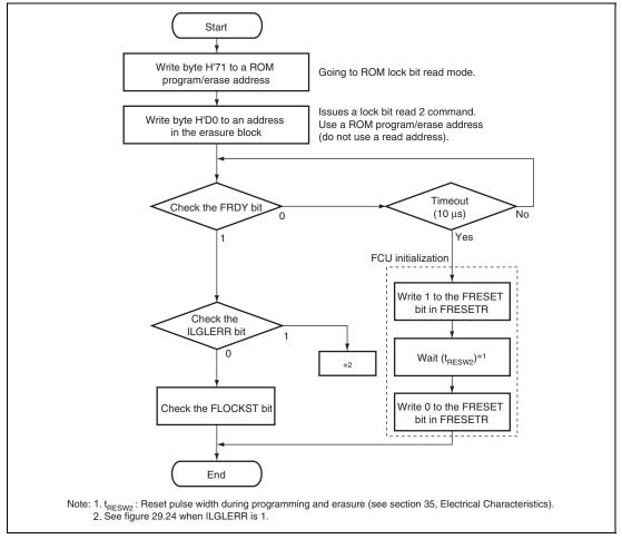
Figure 29.26 Procedure for Reading Lock Bit in Register Read Mode
