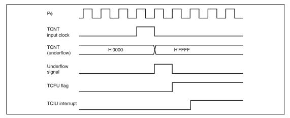
Figure 12.114 TCIU Interrupt Setting Timing
