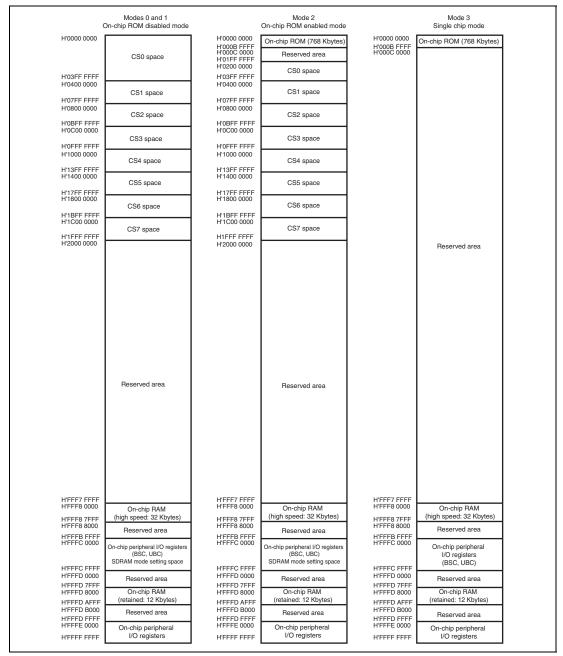
Figure 4.2 Address Map in Each Operating Mode (SH72314L)
