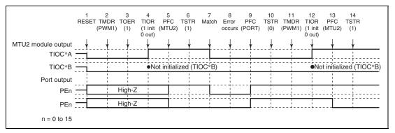
Figure 12.146 Error Occurrence in PWM Mode 1, Recovery in PWM Mode 1
