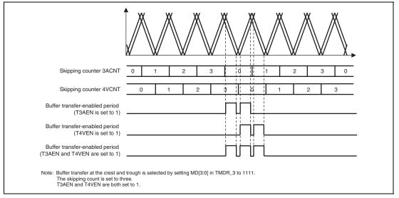
Figure 12.78 Relationship between Bits T3AEN and T4VEN in TITCR and Buffer Transfer-Enabled Period
