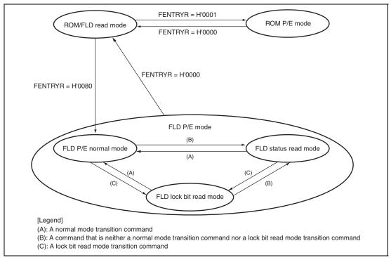
Figure 30.5 FCU Mode Transition Diagram (FLD-Related Modes)
