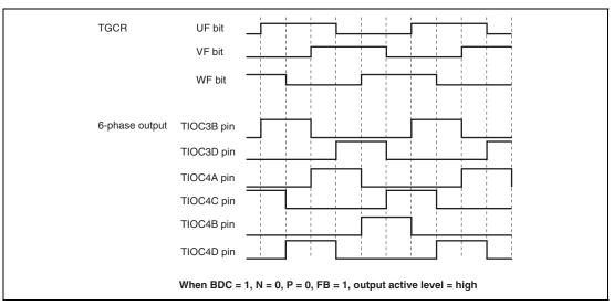
Figure 12.71 Example of Output Phase Switching by Means of UF, VF, and WF Bit Settings (1)
