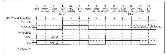
Figure 12.140 Error Occurrence in Normal Mode, Recovery in PWM Mode 1
