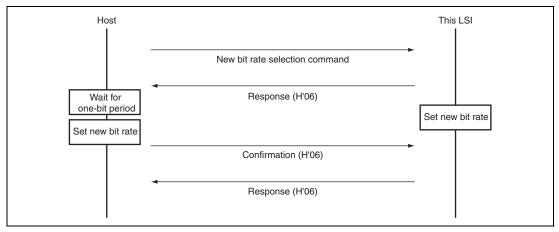
Figure 29.10 New Bit Rate Selection Sequence
