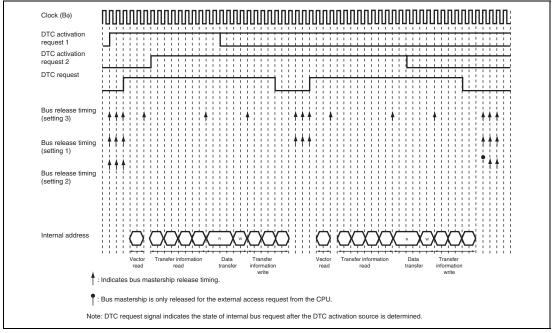
Figure 9.16 Example of DTC Operation Timing: Conflict of Two Activation Requests in Normal Transfer Mode (Activated by On-Chip Peripheral Module;  $I\phi : B\phi : P\phi = 1 : 1/2 : 1/2$ ; Data Transferred from On-Chip Peripheral Module to On-Chip RAM (High Speed); **Transfer Information is Written in 3 Cycles)**
