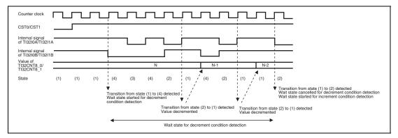
Figure 27.4 Example of TI32CNT8 Decrement Operation in Normal Two-Phase Counter Mode
