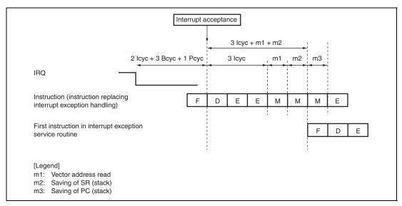
Figure 7.6 Example of Pipeline Operation when IRQ Interrupt is Accepted (Register Banking without Register Bank Overflow)
