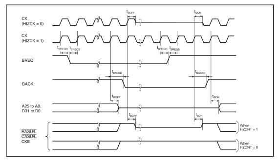
Figure 35.13 Bus Release Timing
