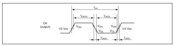
Figure 35.4 CK Clock Output Timing
