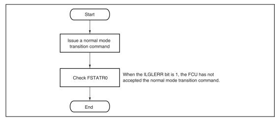
Figure 29.19 Procedure to Use ROM P/E Normal Mode Transition Command
