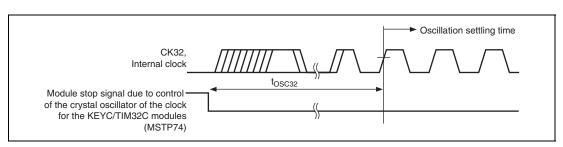
Figure 35.10 EXTAL32 Clock Oscillation Settling Time
