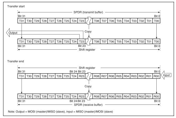
Figure 25.14 MSB First Transfer (24-Bit Data)
