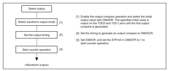
Figure 16.5 Procedure for Setting Output Compare Operation
