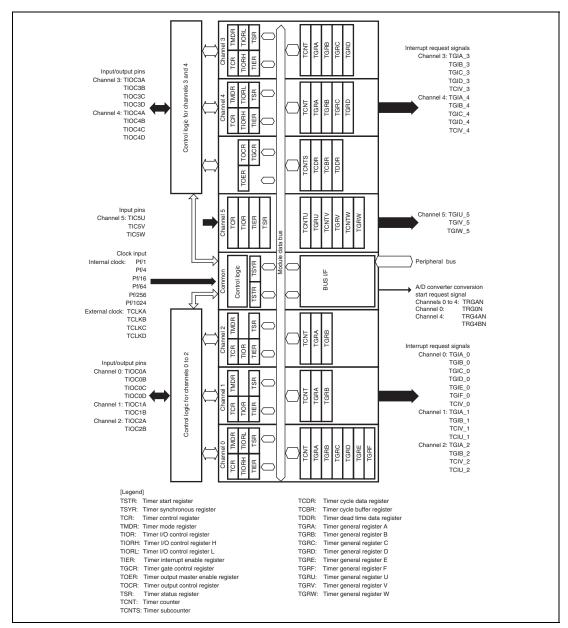
Figure 12.1 Block Diagram of MTU2
