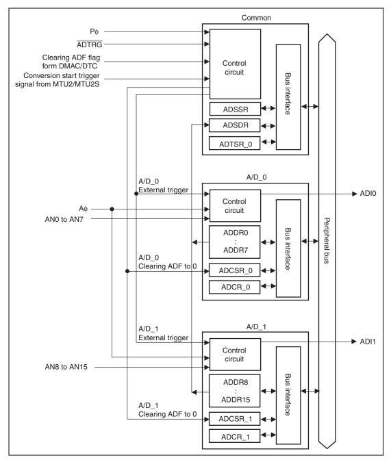
Figure 21.2 the Structure of the A/D Converter
