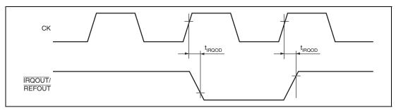
Figure 35.14 Interrupt Signal Output Timing
