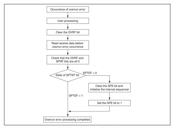
Figure 25.31 Error Processing (Overrun Error)
