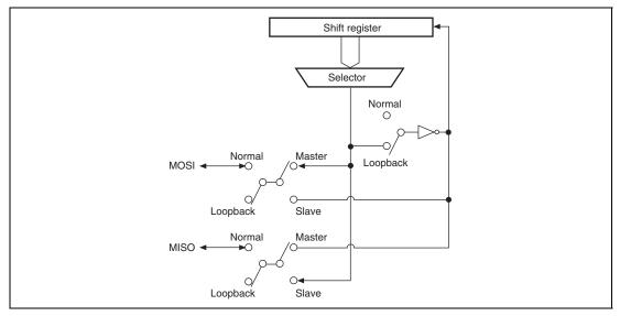
Figure 25.33 Configuration of Shift Register Input/Output Paths in Loopback Mode (Master Mode)
