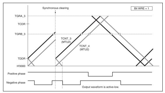
Figure 12.58 Example of Synchronous Clearing in Dead Time during Up-Counting (Timing (3) in Figure 12.56; Bit WRE in TWCR of MTU2 is 1)
