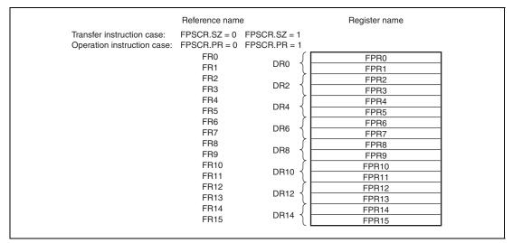
Figure 3.4 Floating-Point Registers
