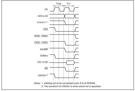
Figure 10.26 Single Write Timing (Bank Active, Same Row Addresses in the Same Bank)
