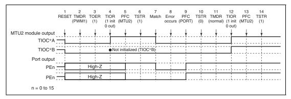
Figure 12.145 Error Occurrence in PWM Mode 1, Recovery in Normal Mode
