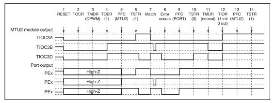
Figure 12.159 Error Occurrence in Complementary PWM Mode, **Recovery in Normal Mode**
