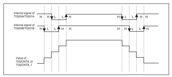
Figure 27.5 Example of TI32CNT8 Operation in High-Speed Two-Phase Counter Mode
