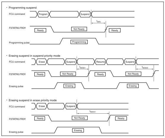
Figure 35.69 Flash Programming/Erasing Suspend Timing
