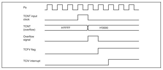
Figure 12.113 TCIV Interrupt Setting Timing
