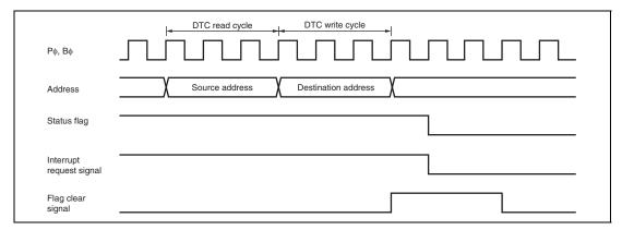
Figure 12.118 Timing for Status Flag Clearing by DTC Activation (Channel 5)
