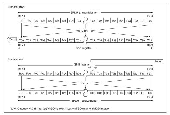
Figure 25.16 LSB First Transfer (24-Bit Data)
