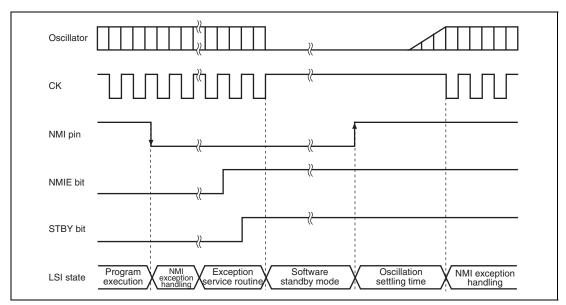
Figure 32.3 NMI Timing in Software Standby Mode (Application Example)
