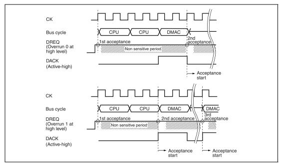
Figure 11.16 Example of DREQ Input Detection in Burst Mode Level Detection
