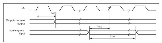
Figure 35.45 MTU2 Input/Output Timing
