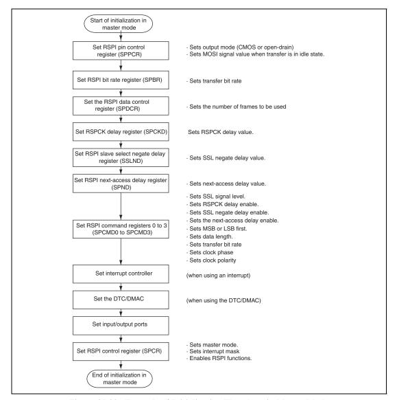
Figure 25.29 Example of Initialization Flowchart in Master Mode
