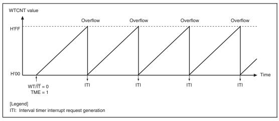
Figure 17.5 Operation in Interval Timer Mode
