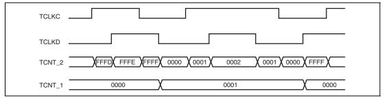
Figure 12.21 Cascaded Operation Example (a)
