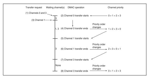
Figure 11.4 Changes in Channel Priority in Round-Robin Mode
