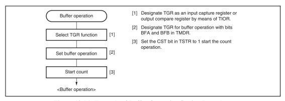
Figure 12.16 Example of Buffer Operation Setting Procedure
