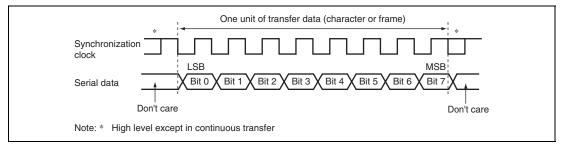
Figure 18.8 Data Format in Clock Synchronous Communication (when LSB-First Transfer is Selected)
