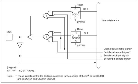
Figure 18.20 SCKIO Bit, SCKDT Bit, and SCK Pin
