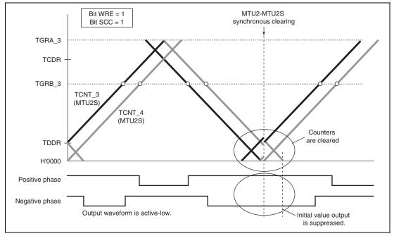
Figure 12.67 Example of Synchronous Clearing in Interval Tb at Trough (Timing (11) in Figure 12.56; Bit WRE is 1 and Bit SCC is 1 in TWCR of MTU2S)
