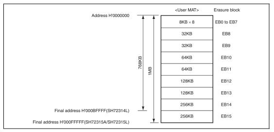
Figure 29.3 Block Configuration of User MAT
