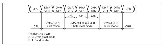
Figure 11.12 Bus State when Multiple Channels are Operating
