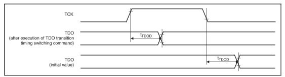
Figure 33.4 H-UDI Data Transfer Timing
