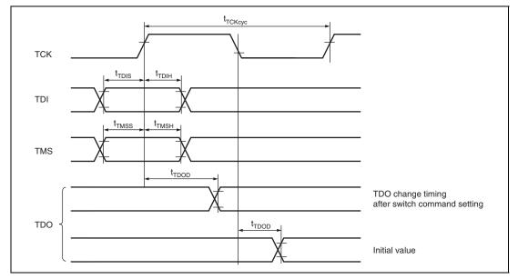
Figure 35.67 H-UDI Data Transmission Timing
