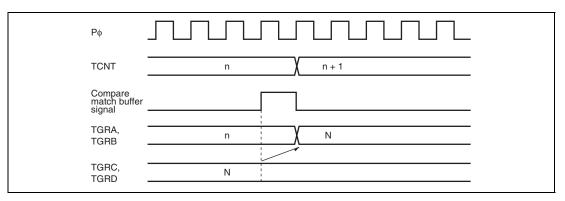
**Figure 12.103 Buffer Operation Timing (Compare Match)**
