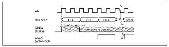
Figure 11.15 Example of DREQ Input Detection in Burst Mode Edge Detection
