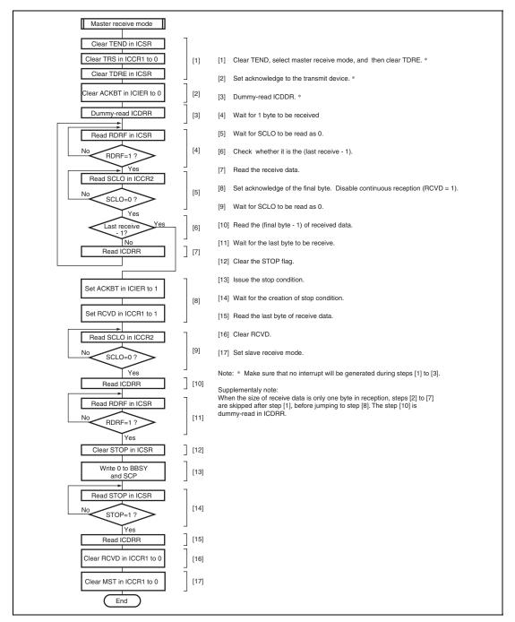
Figure 20.19 Sample Flowchart for Master Receive Mode
