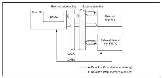
Figure 11.7 Data Flow in Single Address Mode
