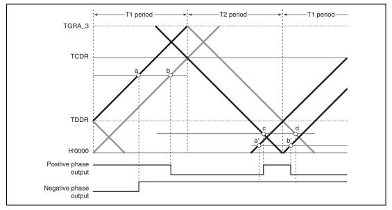
Figure 12.48 Example of Complementary PWM Mode Waveform Output (3)
