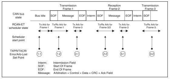
Figure 26.11 Internal Arbitration for Transmission
