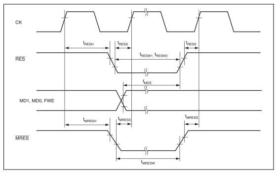
Figure 35.11 Reset Input Timing
