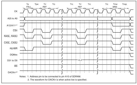
Figure 10.32 SDRAM Mode Write Timing (Based on JEDEC)
