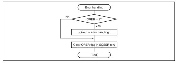
Figure 18.12 Sample Flowchart for Receiving Serial Data (2)
