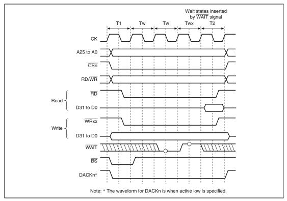
Figure 10.9 Wait Cycle Timing for Normal Space Access (Wait Cycle Insertion Using WAIT Signal)
