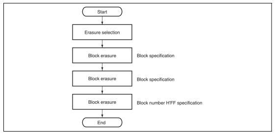
Figure 29.12 Procedure for ROM Erasure in Boot Mode
