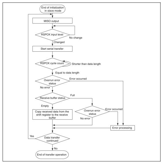
Figure 25.27 Example of Transfer Operation Flowchart in Slave Mode (CPHA = 1)
