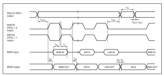
Figure 35.60 RSPI Timing (Master, CPHA = 1)
