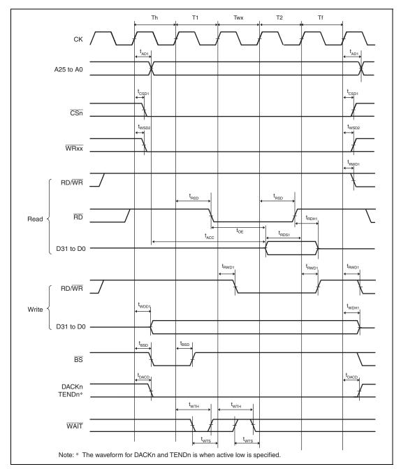
Figure 35.21 Bus Cycle of SRAM with Byte Selection (SW = 1 Cycle, HW = 1 Cycle, One Asynchronous External Wait Cycle, BAS = 1 (Write Cycle WE Control))
