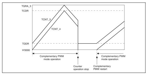
Figure 12.132 Counter Value during Complementary PWM Mode Stop
