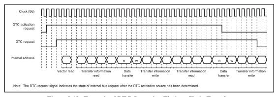
Figure 9.12 Example of DTC Operation Timing: Chain Transfer (Activated by On-Chip Peripheral Module;  $I\phi : B\phi : P\phi = 1 : 1/2 : 1/2$ ; Data Transferred from On-Chip Peripheral Module to On-Chip RAM (High Speed); **Transfer Information is Written in 3 Cycles)**
