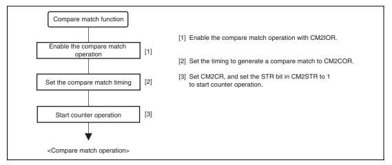
Figure 16.2 Procedure for Setting Compare Match Operation
