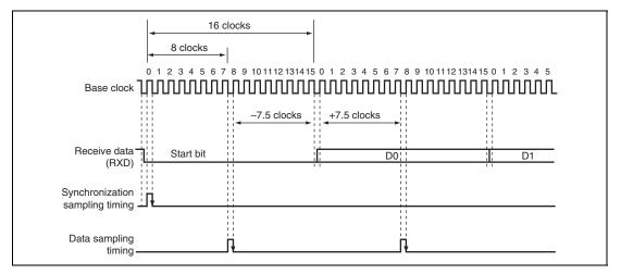
Figure 18.22 Receive Data Sampling Timing in Asynchronous Mode
