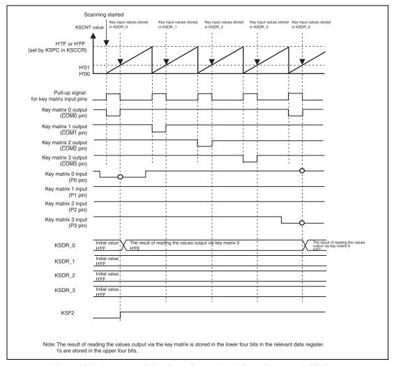
Figure 28.4 Example of Key Scan Operation (4 Scan Outputs: KSOC = 1)
