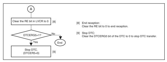
Figure 24.12 Example of Data Transfer from LVDS Receive FIFO Data Register by DTC (2)
