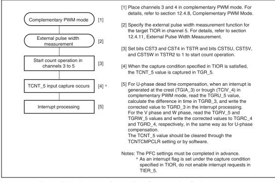
Figure 12.90 Example of Dead Time Compensation Setting Procedure
