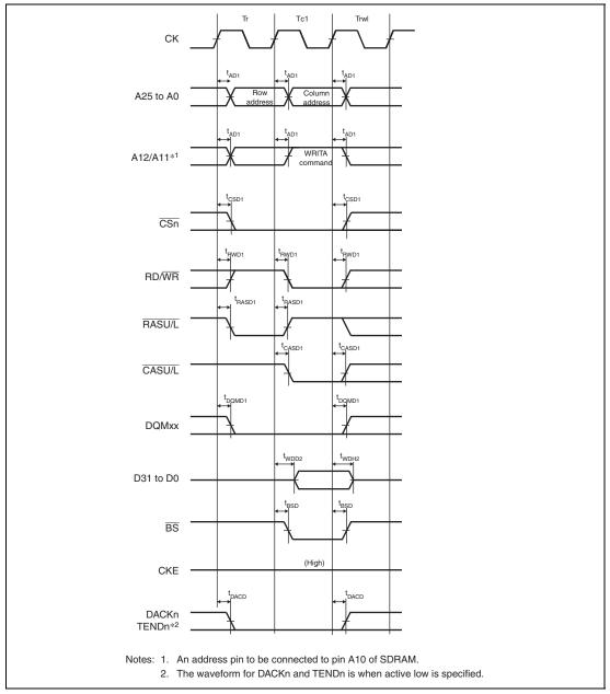
Figure 35.27 Synchronous DRAM Single Write Bus Cycle (Auto Precharge, TRWL = 1 Cycle)
