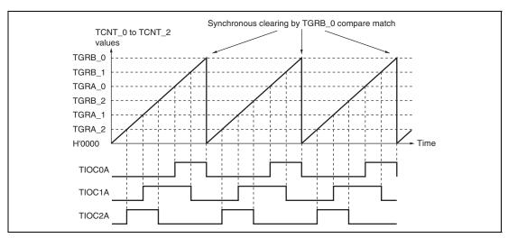
Figure 12.13 Example of Synchronous Operation
