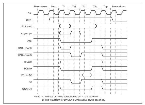
Figure 10.31 Power-Down Mode Access Timing
