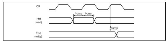
Figure 35.53 I/O Port Timing
