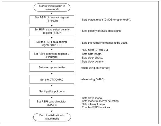
Figure 25.19 Example of Initialization Flowchart in Slave Mode
