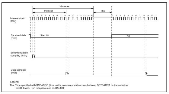
Figure 18.19 Operation Example when Bit Rate Adjustment Function is Enabled (when SPSEL[1:0] = 01 (sampling data on the ninth clock pulse))
