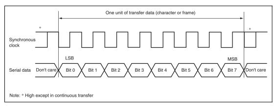
Figure 19.9 Data Format in Clocked Synchronous Communication (when LSB-First Transfer is Selected)
