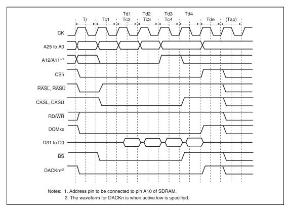
Figure 10.17 Burst Read Basic Timing (CAS Latency 1, Auto-Precharge)
