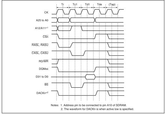
Figure 10.19 Basic Timing for Single Read (CAS Latency 1, Auto-Precharge)
