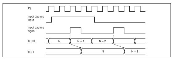
Figure 12.99 Input Capture Input Signal Timing
