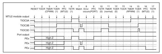
Figure 12.163 Error Occurrence in Complementary PWM Mode, Recovery in Reset-Synchronized PWM Mode
