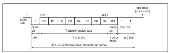
Figure 18.2 Example of Data Format in Asynchronous Communication (8-Bit Data with Parity and Two Stop Bits when LSB-First Transfer is Selected)
