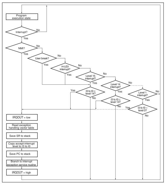
Figure 7.2 Interrupt Operation Flow
