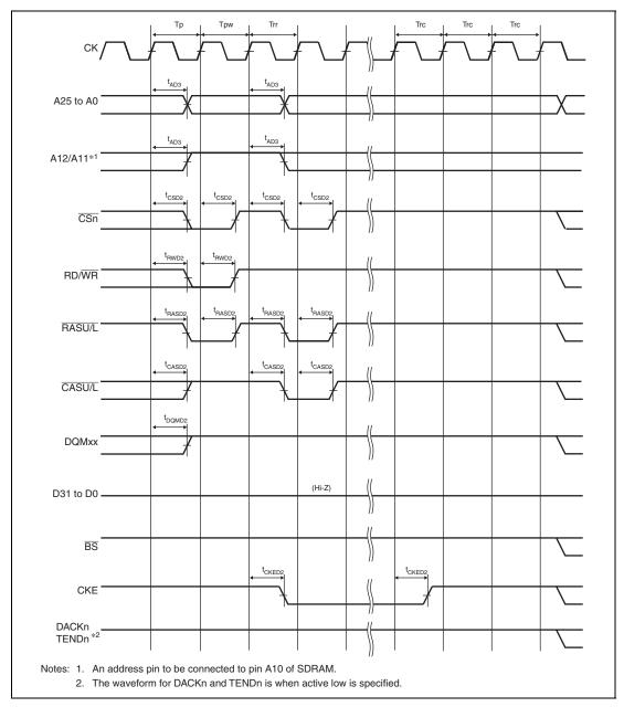
Figure 35.41 Synchronous DRAM Self-Refreshing Timing in Low-Frequency Mode (WTRP = 2 Cycles)
