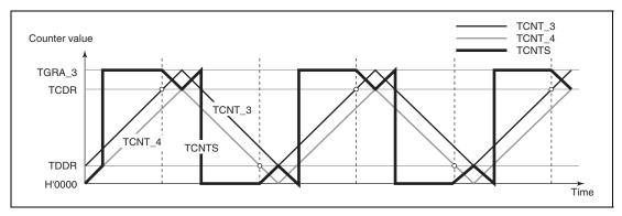
Figure 12.39 Complementary PWM Mode Counter Operation
