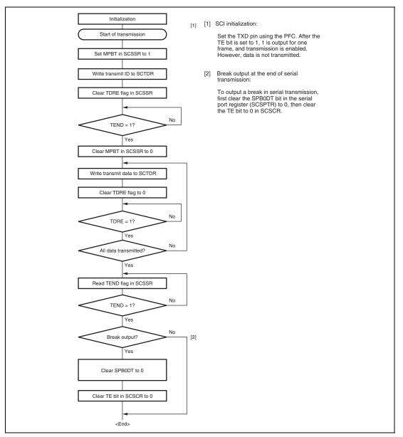
Figure 18.16 Sample Multiprocessor Serial Transmission Flowchart
