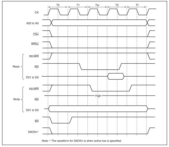
Figure 10.38 Wait Timing for SRAM with Byte Selection (BAS = 1) (SW[1:0] = 01, WR[3:0] = 0001, HW[1:0] = 01)
