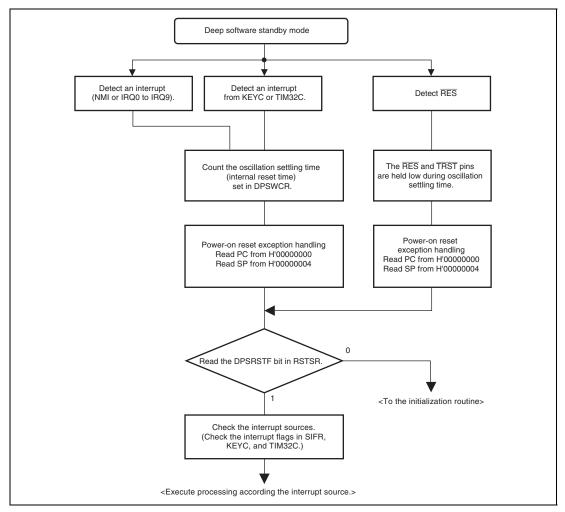
Figure 32.5 Flowchart of Canceling Deep Software Standby Mode
