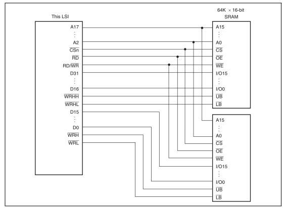
Figure 10.39 Example of Connection with 32-Bit Data-Width SRAM with Byte Selection
