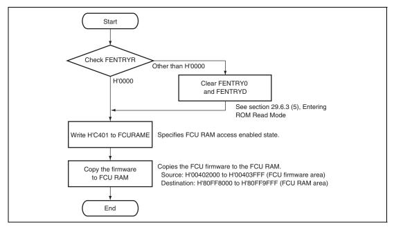
Figure 29.15 Procedure for Firmware Transfer to FCU RAM
