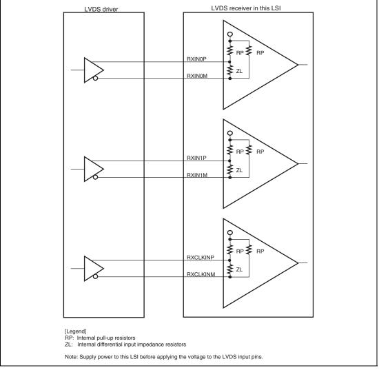
Figure 24.2 Example of Connecting LVDS Differential Input Circuits
