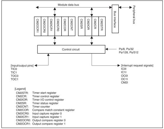
Figure 16.1 Block Diagram of CMT2
