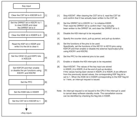
Figure 28.3 Key Input Setting Procedure
