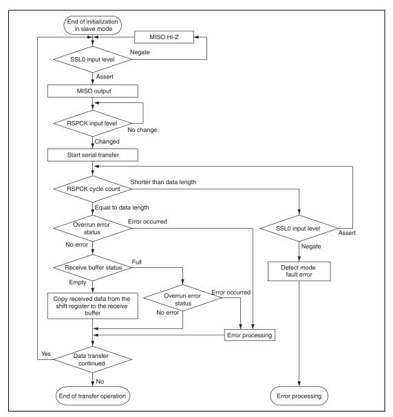
Figure 25.21 Example of Transfer Operation Flowchart in Slave Mode (CPHA = 1)
