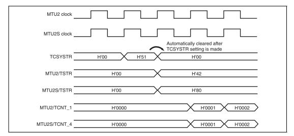
Figure 12.84 (1) Example of Synchronous Counter Start Operation (MTU2-to-MTU2S Clock Frequency Ratio = 1:1)
