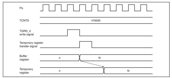
Figure 12.106 Transfer Timing from Buffer Register to Temporary Register (TCNTS Stop)
