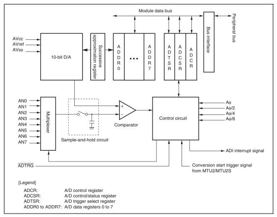
Figure 21.1 Block Diagram of A/D Converter (Figure of One Module)
