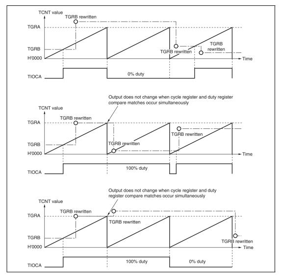
Figure 12.28 Example of PWM Mode Operation (3)
