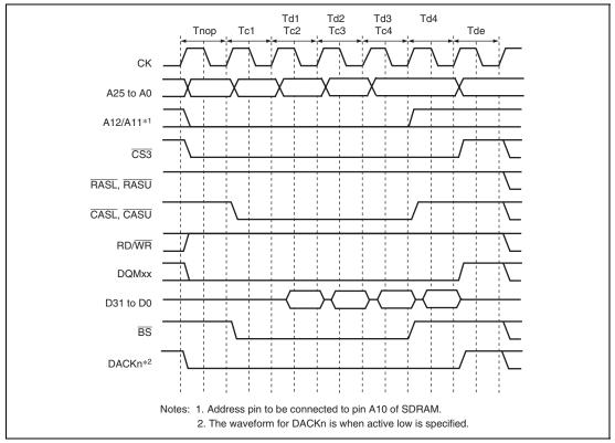
Figure 10.23 Burst Read Timing (Bank Active, Same Row Addresses in the Same Bank, CAS Latency 1)
