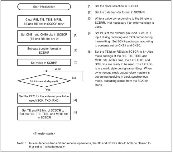
Figure 18.9 Sample Flowchart for SCI Initialization
