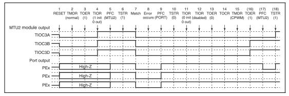
Figure 12.143 Error Occurrence in Normal Mode, **Recovery in Complementary PWM Mode**
