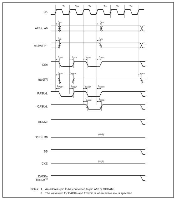
Figure 35.37 Synchronous DRAM Auto-Refreshing Timing (WTRP = 1 Cycle, WTRC = 3 Cycles)
