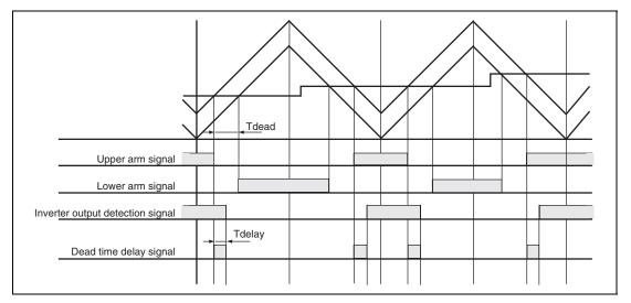
Figure 12.89 Delay in Dead Time in Complementary PWM Operation
