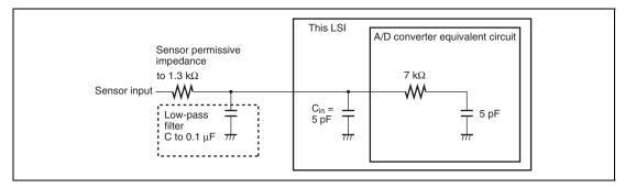
Figure 21.11 Example of Analog Input Circuit
