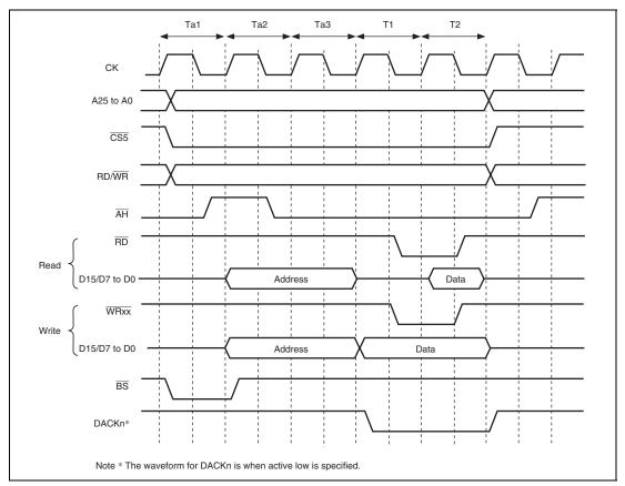
Figure 10.11 Access Timing for MPX Space (Address Cycle No Wait, Data Cycle No Wait)
