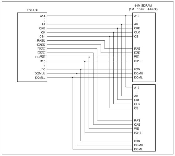
Figure 10.16 Example of 16-Bit Data Width SDRAM Connection (RASU and CASU are Used)
