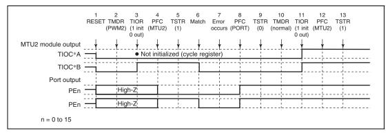
Figure 12.151 Error Occurrence in PWM Mode 2, Recovery in Normal Mode
