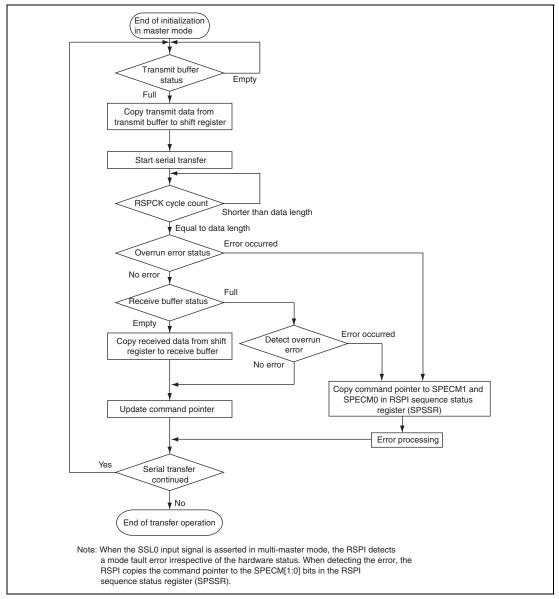
Figure 25.25 Example of Transfer Operation Flowchart in Master Mode
