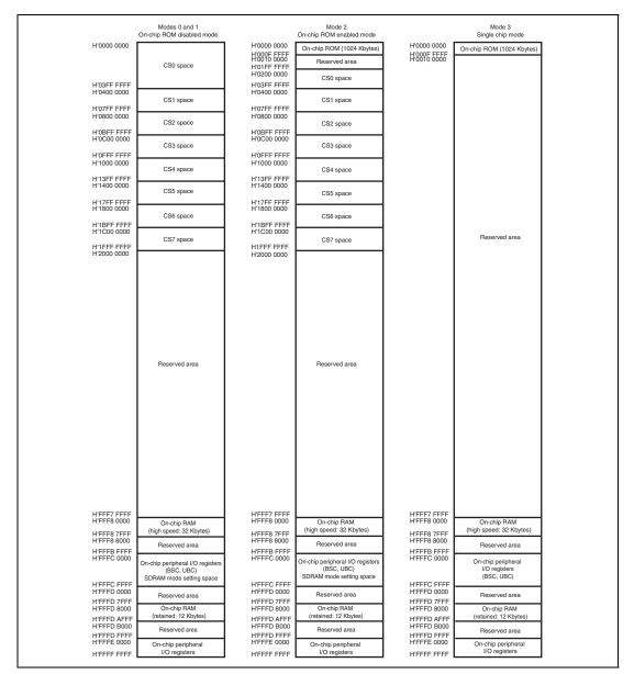
Figure 4.1 Address Map in Each Operating Mode (SH72315A/SH72315L)
