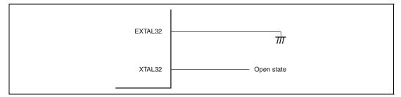
Figure 5.7 Handling of Pins when the Clock for the KEYC and TIM32C Modules is Not in Use
