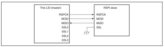
Figure 25.3 Single-Master/Single-Slave Configuration Example (This LSI = Master)
