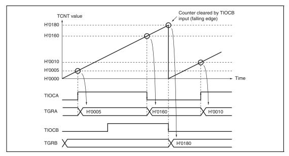
Figure 12.11 Example of Input Capture Operation
