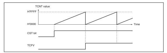
Figure 12.5 Free-Running Counter Operation
