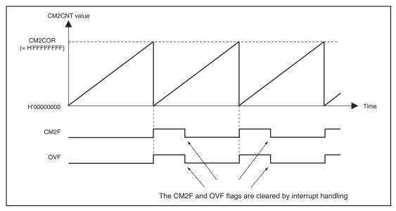
Figure 16.4 Example of Compare Match Operation (overflow detected)
