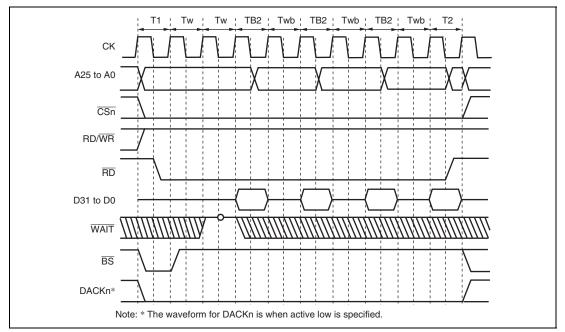
Figure 10.35 Burst ROM Access Timing (Clock Asynchronous)
