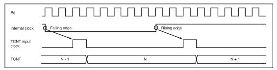
Figure 12.93 Count Timing in Internal Clock Operation (Channels 0 to 4)
