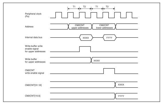
Figure 16.12 CM2CNT Write Operation Example
