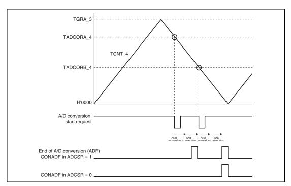
Figure 21.5 Example of 2-Channel Scan Mode Operation
