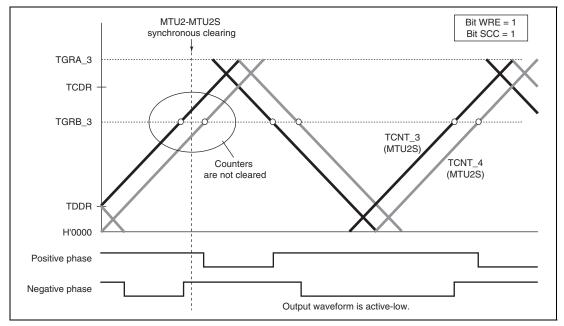
Figure 12.64 Example of Synchronous Clearing in Dead Time during Up-Counting (Timing (3) in Figure 12.56; Bit WRE is 1 and Bit SCC is 1 in TWCR of MTU2S)
