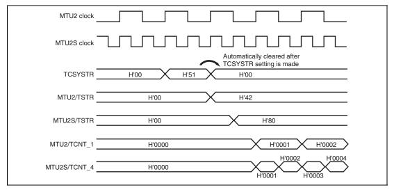
Figure 12.84 (2) Example of Synchronous Counter Start Operation (MTU2-to-MTU2S Clock Frequency Ratio = 1:2)
