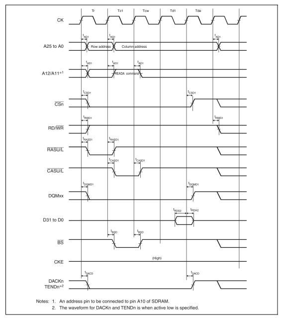
Figure 35.23 Synchronous DRAM Single Read Bus Cycle (Auto Precharge, CAS Latency 2, WTRCD = 0 Cycle, WTRP = 0 Cycle)
