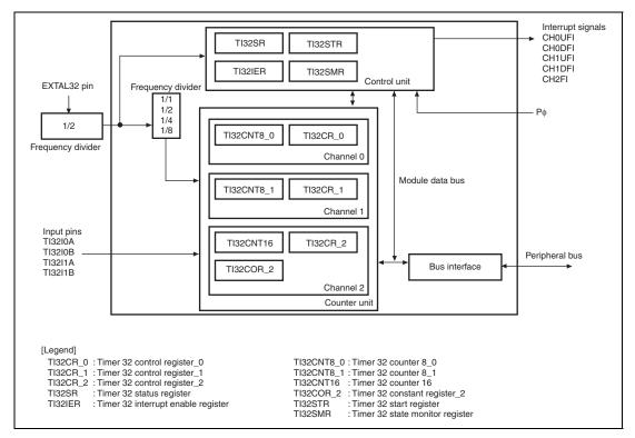
Figure 27.1 Block Diagram of TIM32C
