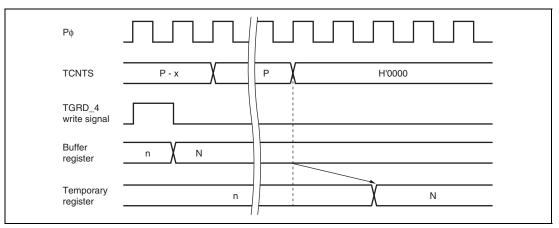
Figure 12.107 Transfer Timing from Buffer Register to Temporary Register (TCNTS Operating)
