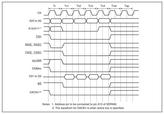
Figure 10.20 Basic Timing for Burst Write (Auto-Precharge)
