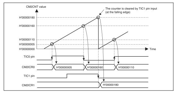
Figure 16.8 Example of Input Capture Operation
