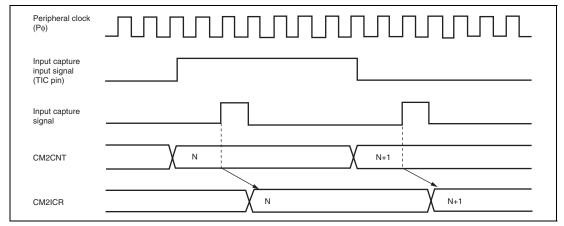
Figure 16.11 Input Capture Input Signal Timing
