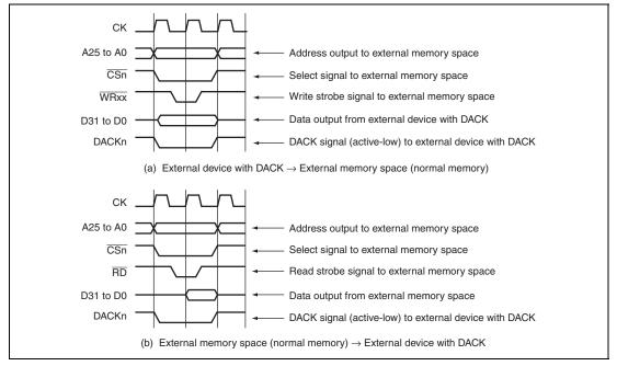
Figure 11.8 Example of DMA Transfer Timing in Single Address Mode
