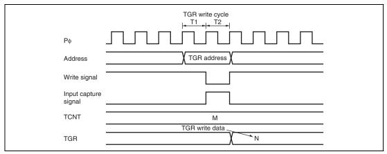
Figure 12.129 Contention between TGR Write and Input Capture (Channel 5)
