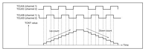
Figure 12.30 Example of Phase Counting Mode 1 Operation
