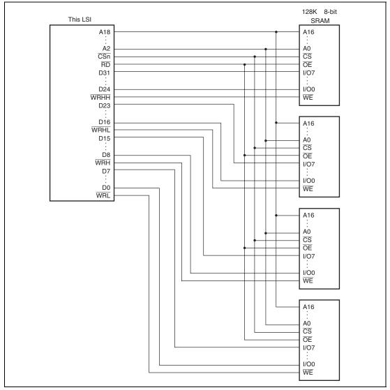
Figure 10.5 Example of 32-Bit Data-Width SRAM Connection
