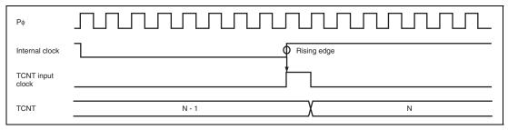
Figure 12.94 Count Timing in Internal Clock Operation (Channel 5)
