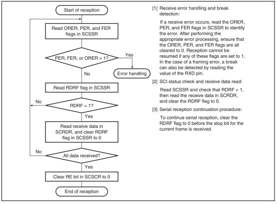
Figure 18.6 Sample Flowchart for Receiving Serial Data (1)
