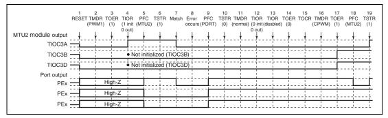
Figure 12.149 Error Occurrence in PWM Mode 1, **Recovery in Complementary PWM Mode**
