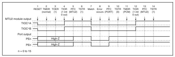
Figure 12.142 Error Occurrence in Normal Mode, Recovery in Phase Counting Mode
