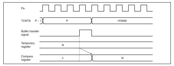
Figure 12.108 Transfer Timing from Temporary Register to Compare Register
