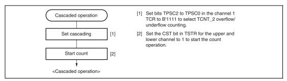
Figure 12.20 Cascaded Operation Setting Procedure
