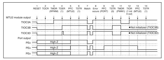
Figure 12.165 Error Occurrence in Reset-Synchronized PWM Mode, Recovery in PWM Mode 1
