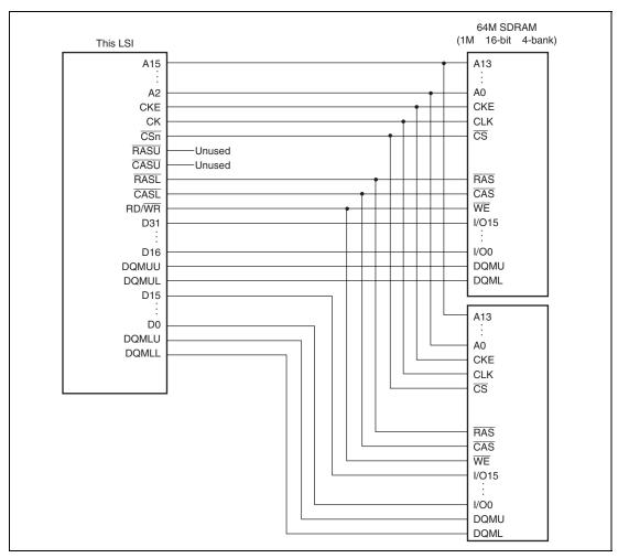
Figure 10.14 Example of 32-Bit Data Width SDRAM Connection (RASU and CASU are Not Used)
