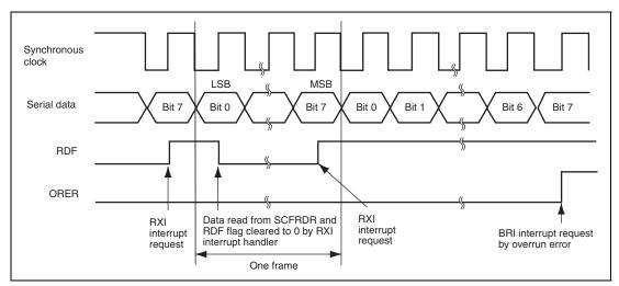
Figure 19.15 Example of SCIF Receive Operation (when LSB-First Transfer is Selected)
