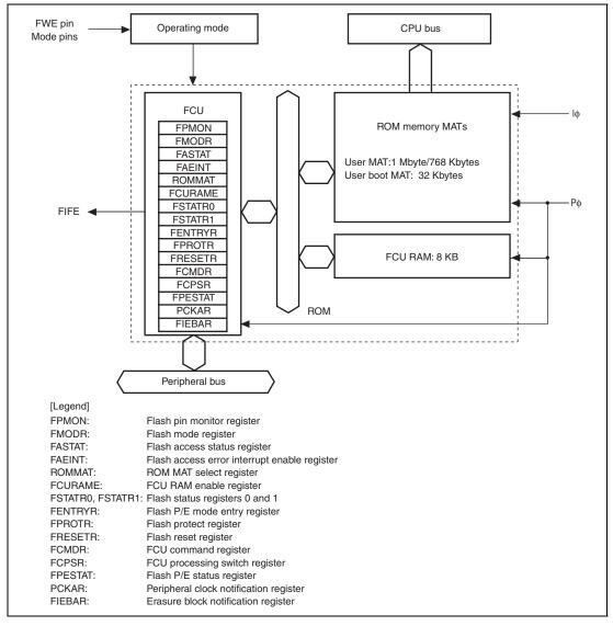
Figure 29.2 Block Diagram of ROM
