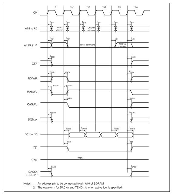
Figure 35.29 Synchronous DRAM Burst Write Bus Cycle (Four Write Cycles)
