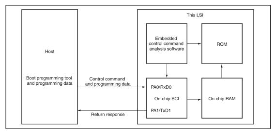
Figure 29.5 System Configuration in Boot Mode
