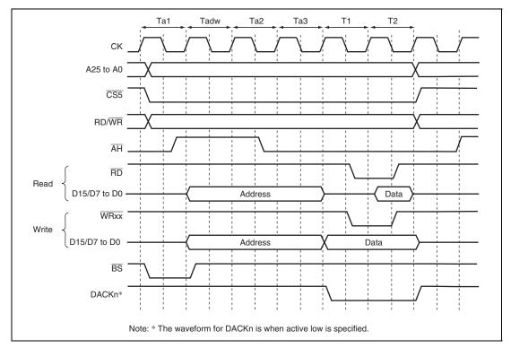
Figure 10.12 Access Timing for MPX Space (Address Cycle Wait 1, Data Cycle No Wait)
