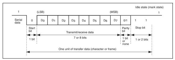
Figure 19.2 Example of Data Format in Asynchronous Communication (8-Bit Data with Parity and Two Stop Bits when LSB-First Transfer is Selected)
