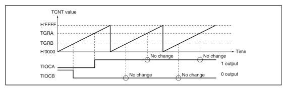
Figure 12.8 Example of 0 Output/1 Output Operation
