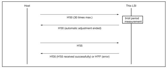
Figure 29.8 Communication Sequence between Host and This LSI
