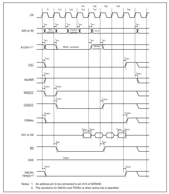
Figure 35.25 Synchronous DRAM Burst Read Bus Cycle (Four Read Cycles) (Auto Precharge, CAS Latency 2, WTRCD = 0 Cycle, WTRP = 1 Cycle)
