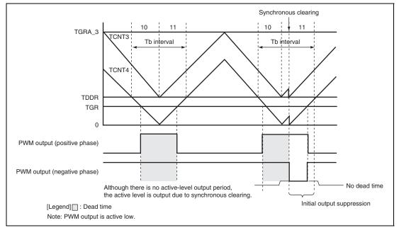
Figure 12.138 Example of Synchronous Clearing for Condition 2
