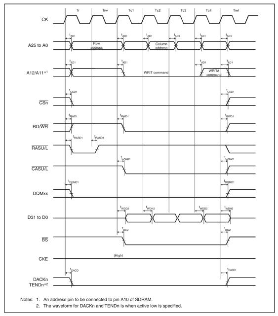
Figure 35.30 Synchronous DRAM Burst Write Bus Cycle (Four Write Cycles)
