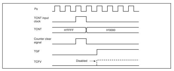
Figure 12.135 Contention between Overflow and Counter Clearing
