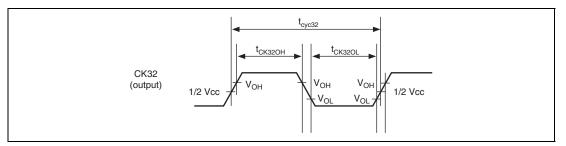
Figure 35.6 CK32 Clock Output Timing
