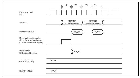
Figure 16.13 CM2CNT Read Operation Example
