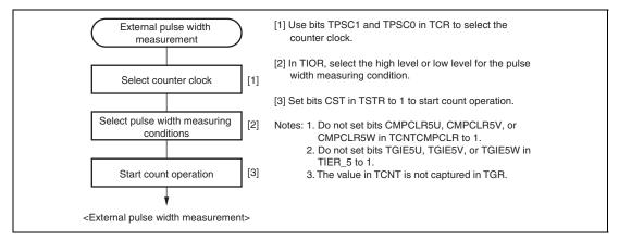
Figure 12.87 Example of External Pulse Width Measurement Setting Procedure
