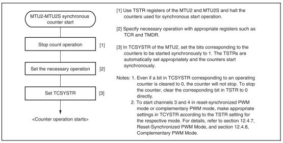
Figure 12.83 Example of Synchronous Counter Start Setting Procedure
