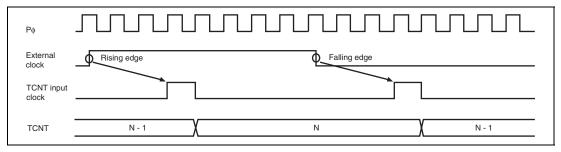
Figure 12.96 Count Timing in External Clock Operation (Phase Counting Mode)
