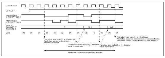
Figure 27.3 Example of TI32CNT8 Increment Operation in Normal Two-Phase Counter Mode
