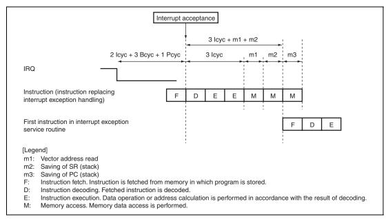
Figure 7.4 Example of Pipeline Operation when IRQ Interrupt is Accepted (No Register Banking)
