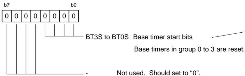
This setting reset Base Timers in Groups 0 to 3. Base Timer of Group i starts counting from 0000<sub>16</sub> by selecting a count source of Base Timer with register GiBCR0 and then set bit BTS = 1 in register GiBCR1.
