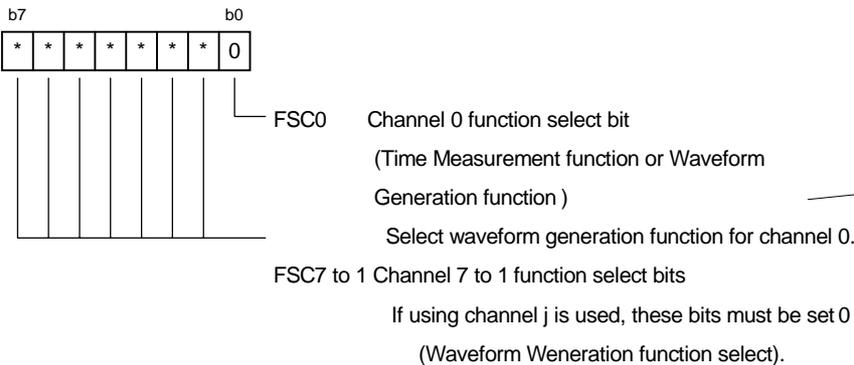
The FSCj bit can select either time measurement function or waveform generation function. The setting doesn't matter if respective channel is not used.
