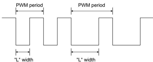
When Group 0 is selected, up to three PWM waveform having the same period can be output. In this case, the low-state of each waveform can be controlled by each channel.
