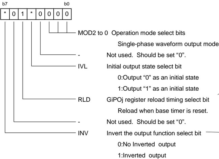
Set the reload timing of the GiPO0 and 1 register as Base Timer reset by the RLD bit set "1".
