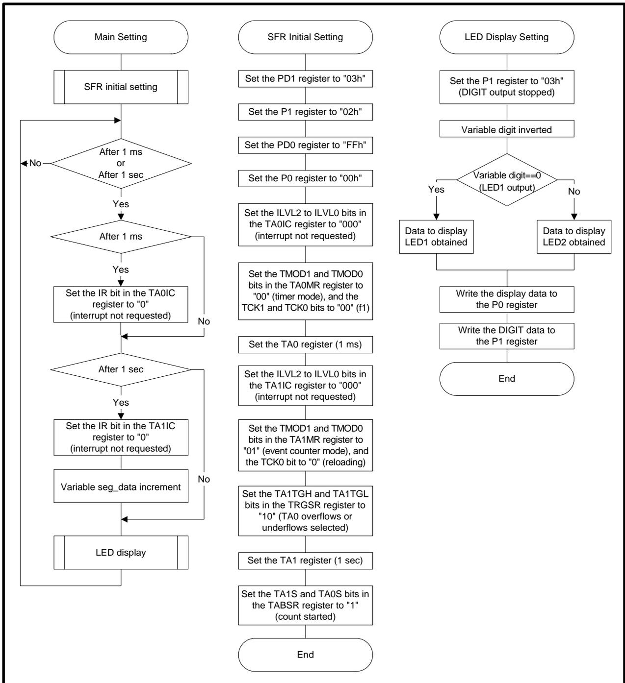
Figure 3. Register Setting Configuration
