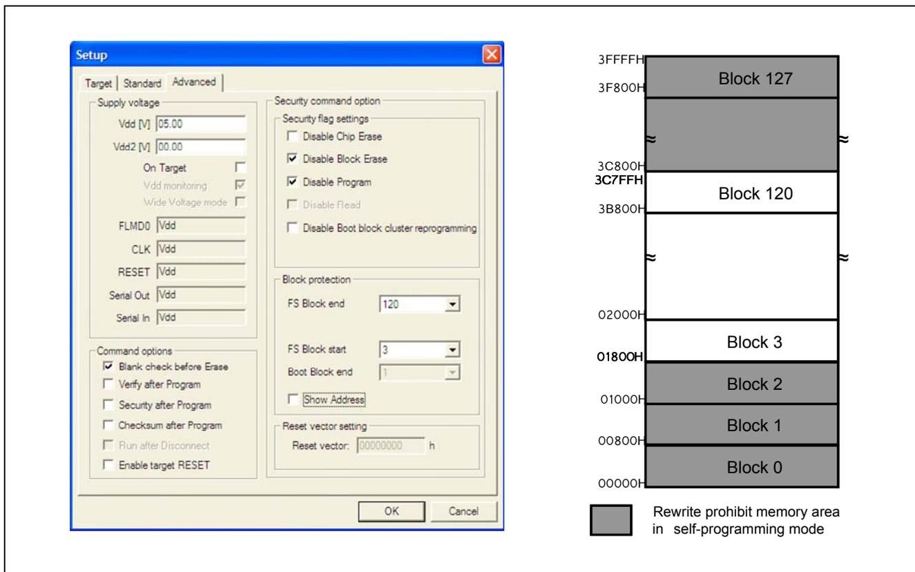
Figure 8 Example of the option data settings in PG-FP5 and its Flash Shield Window memory map
