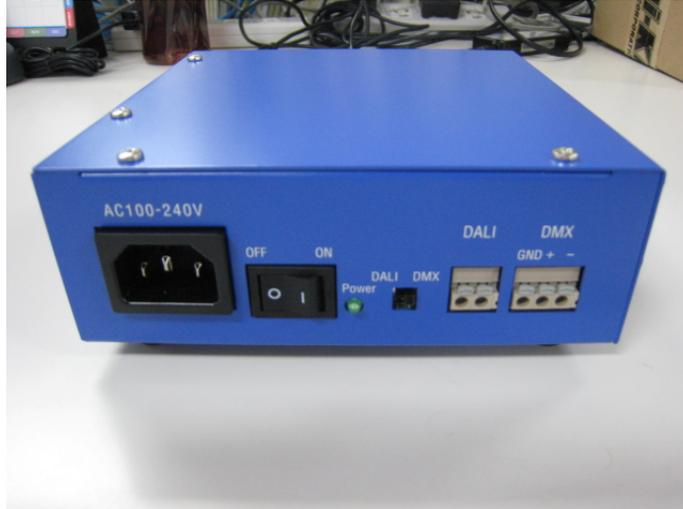
Figure A-2. Front Side of EZ-0011 Main Unit (Switch Input, MINICUBE2 Connection, and LED Connection Side)
