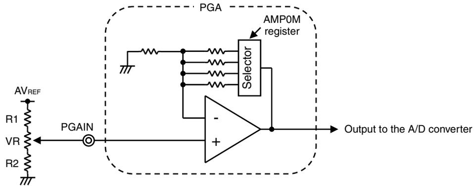
In the figure above, the analog voltage from the variable resistor (VR) connected to the PGAIN pin is amplified by the gain selected using the AMP0M register (fourfold, eightfold, sixteen-fold, or thirty-two-fold), and then output to the A/D converter.
