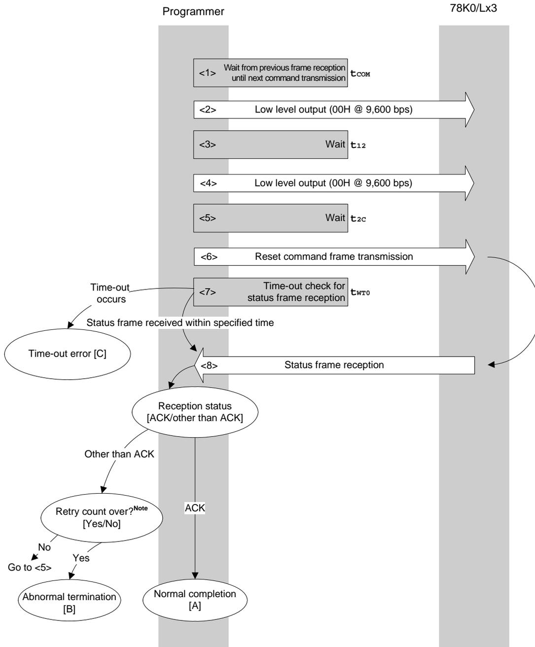
**Note** Do not exceed the retry count for the reset command transmission (up to 16 times).
