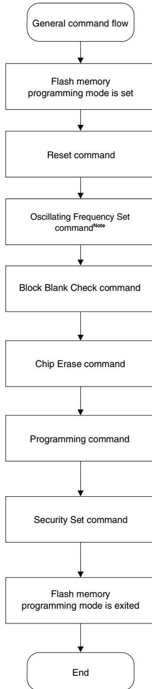
**Note** In the 78K0/Lx3, execution of this command is not necessary when writing to the flash memory during CSI communication mode or UART communication mode with high-speed internal oscillation clock ( $f_{RH}$ ).
