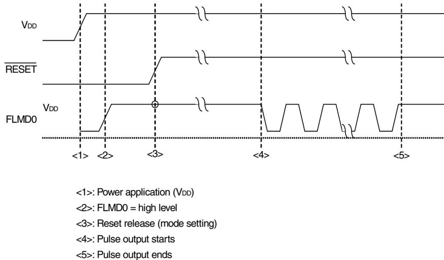
The relationship between the setting of the FLMD0 pin after reset release and the operating mode is shown below.
