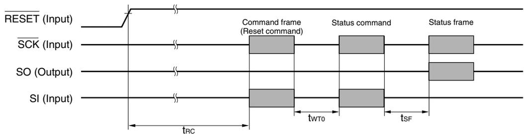
(d) Chip Erase command/Block Erase command/ Block Blank Check command/Oscillating Frequency Set command
