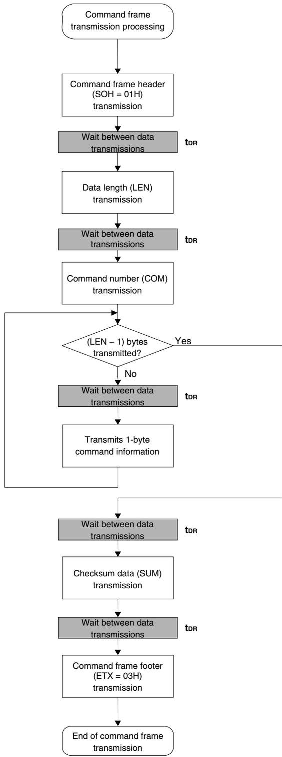
6.2 Data Frame Transmission Processing Flowchart
