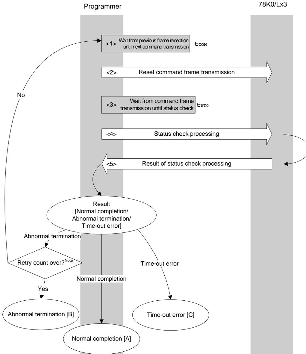
**Note** Do not exceed the retry count for the reset command transmission (up to 16 times).
