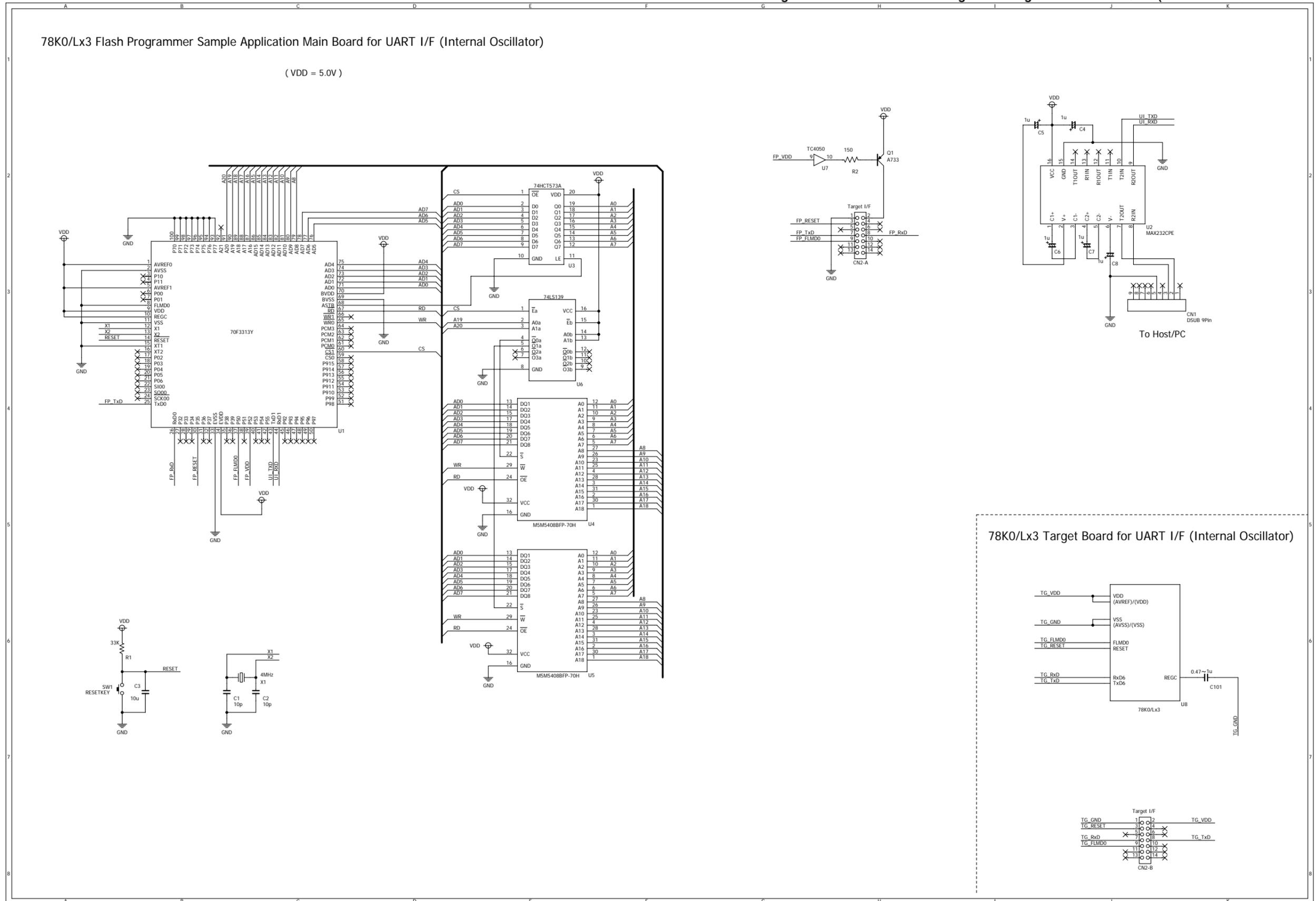
Figure A-4. Reference Circuit Diagram of Programmer and 78K0/Lx3 (During CSI Communication)
