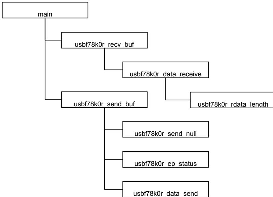
Figure 3-7 Calling Functions during the Processing for the USB function controller
