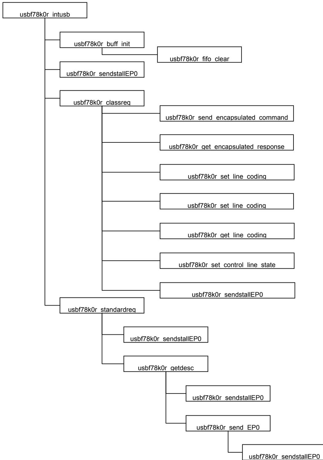
Figure 3-8 Calling Functions during the Processing for the USB Communication Class (1)
