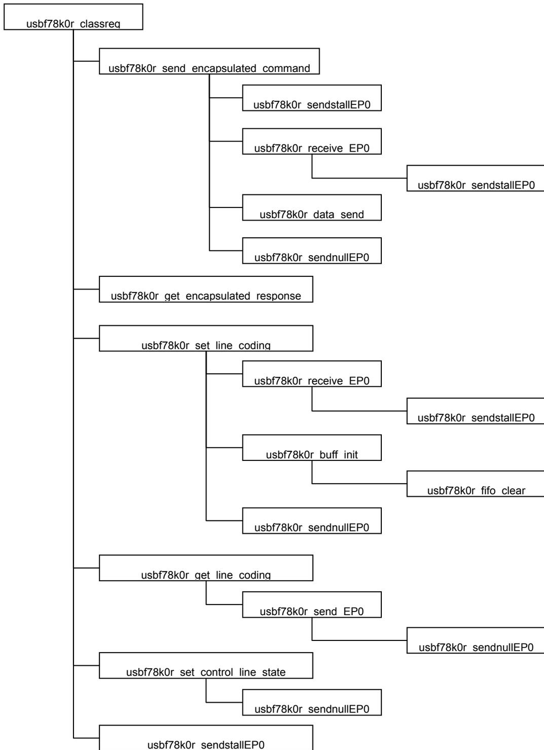
Figure 3-9 Calling Functions during the Processing for the USB Communication Class (2)
