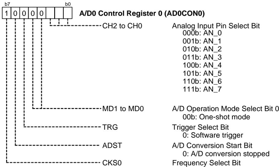
Use the following bits to select the A/D converter operation clock (fAD):
