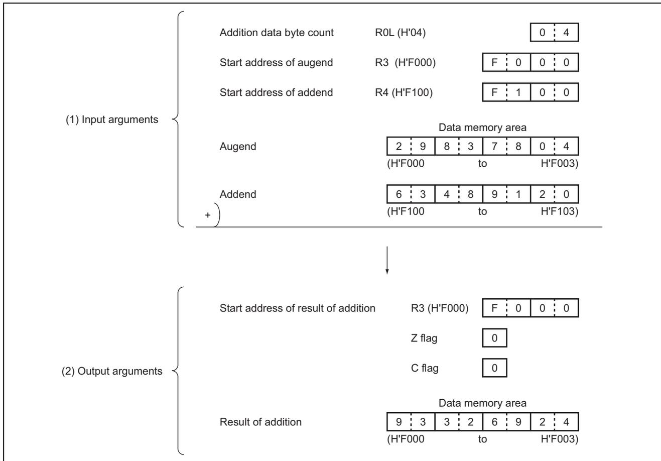
**Figure 1 Example of Software ADDD2 Execution**
