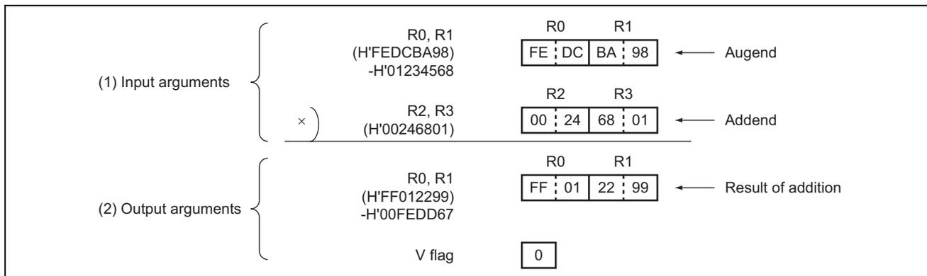
Figure 1 Example of Software SADD Execution
