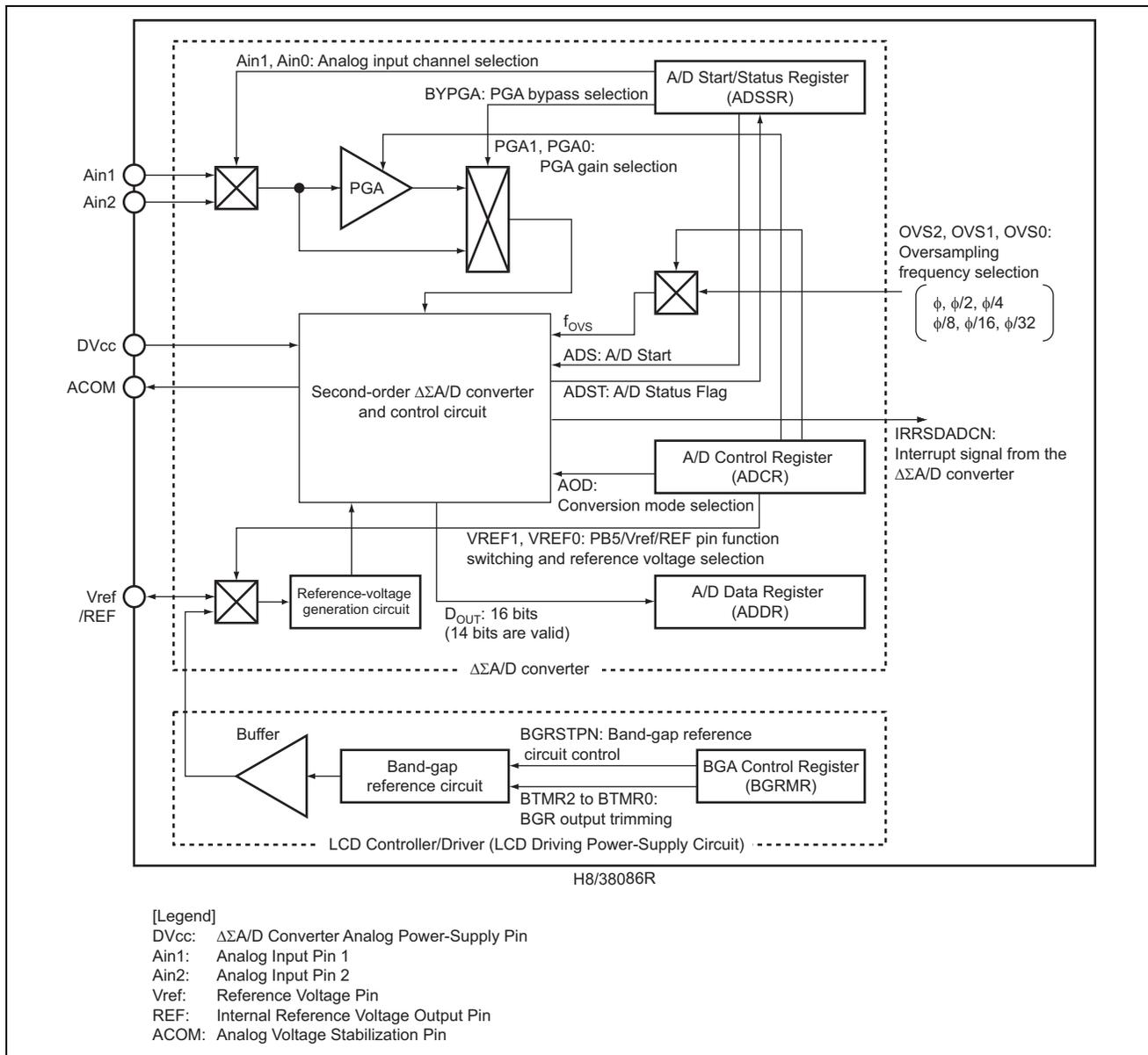
Figure 3 Block Diagram of the  $\Delta\Sigma$ /D Converter
