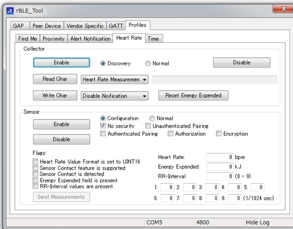
**Figure 7-41 Profiles – Heart Rate tab**
