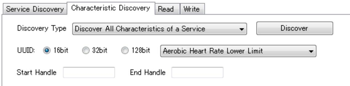
**Figure 7-28 GATT Client – Characteristic Discovery**
