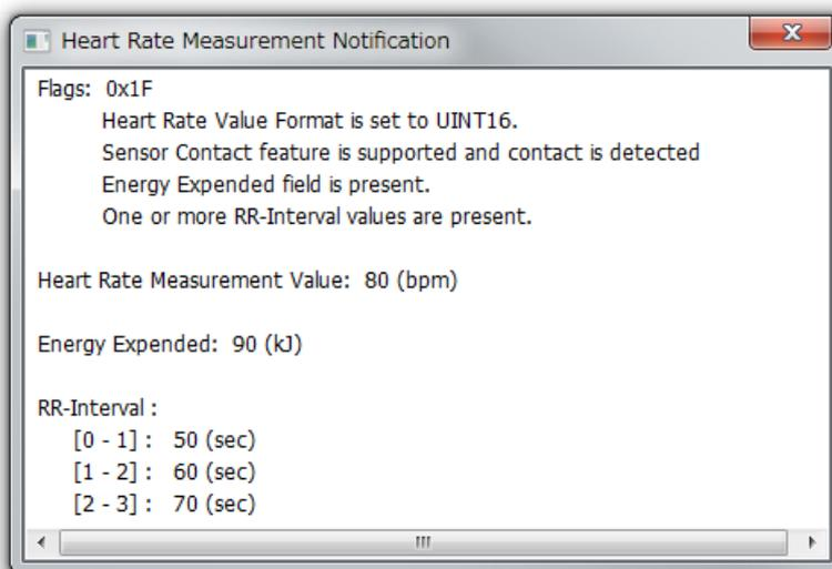
**Figure 7-42 Heart Rate Measurement Notification**
