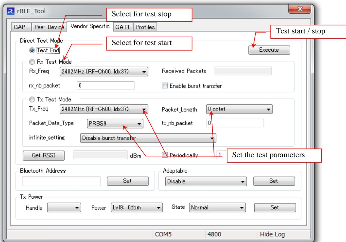
**Figure 8-3 Control of Direct Test Mode (Transmitter)**
