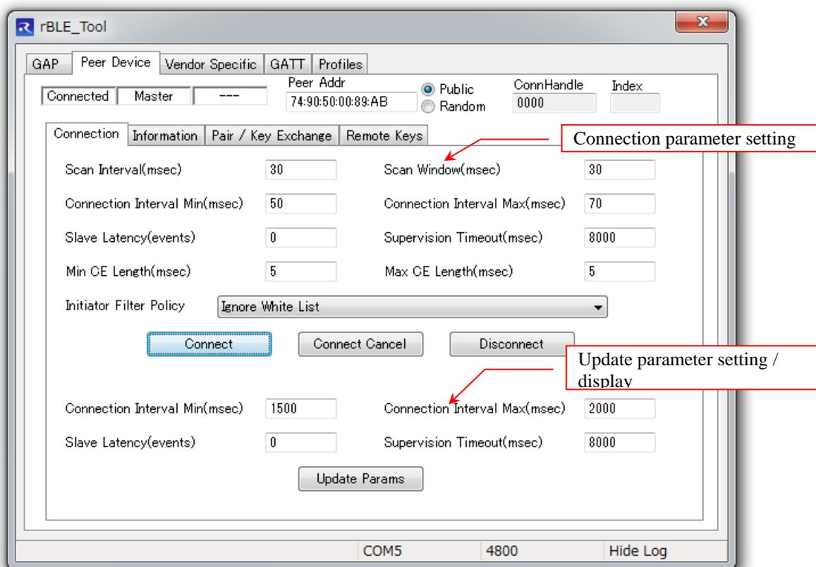
**Figure 7-17 Peer Device – Connection tab**
