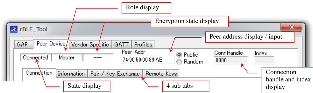
Figure 7-16 Peer Device tab
