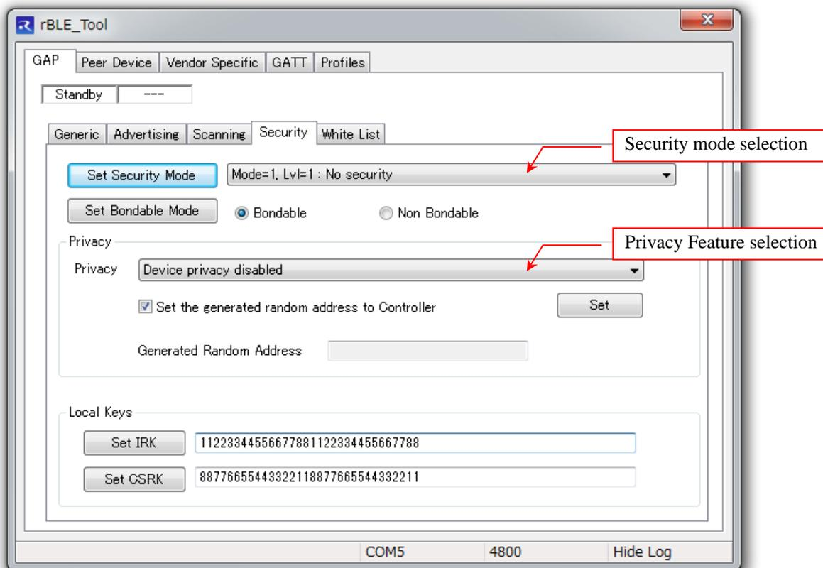
**Figure 7-14 GAP – Security tab**
