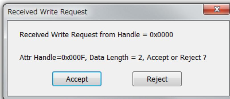
Figure 7-32 Write Indication by “Write Request”
