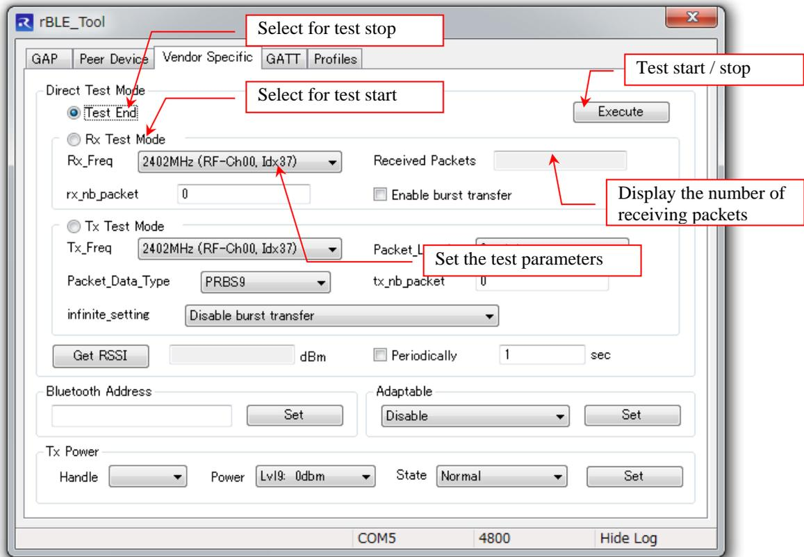
**Figure 8-2 Control of Direct Test Mode (Receiver)**
