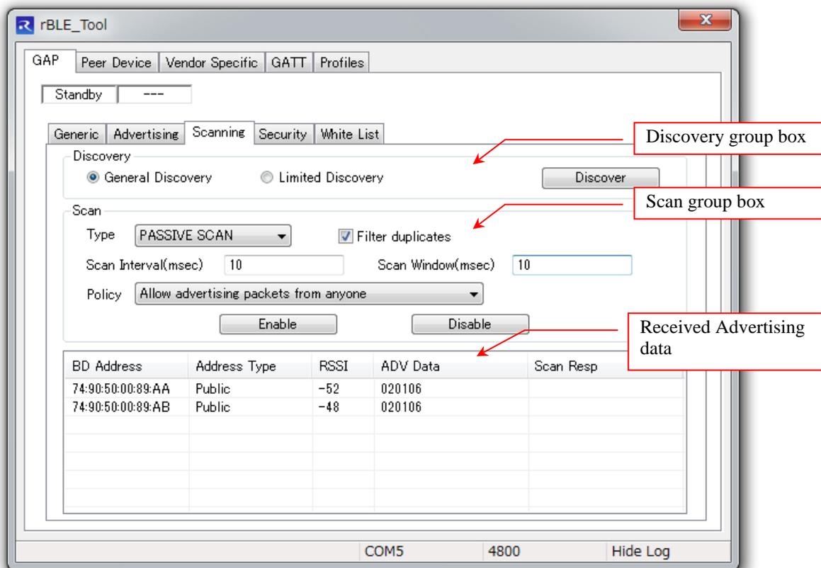
**Figure 7-11 GAP – Scanning tab**
