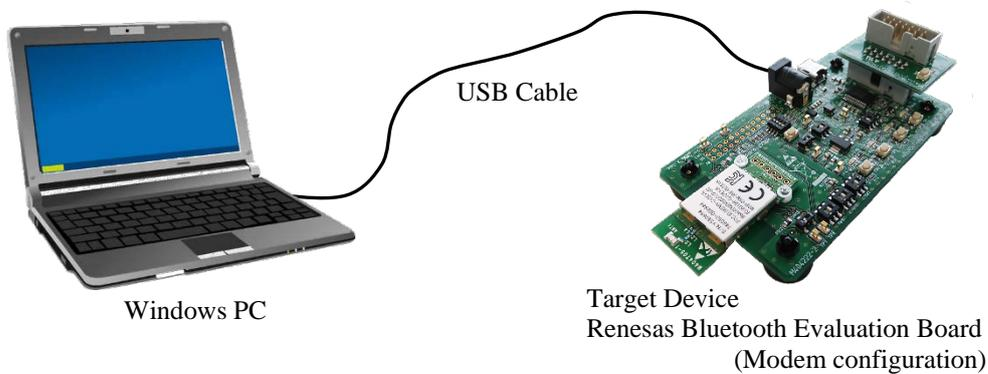
**Figure 6-1 The GUI Tool interface setup**
