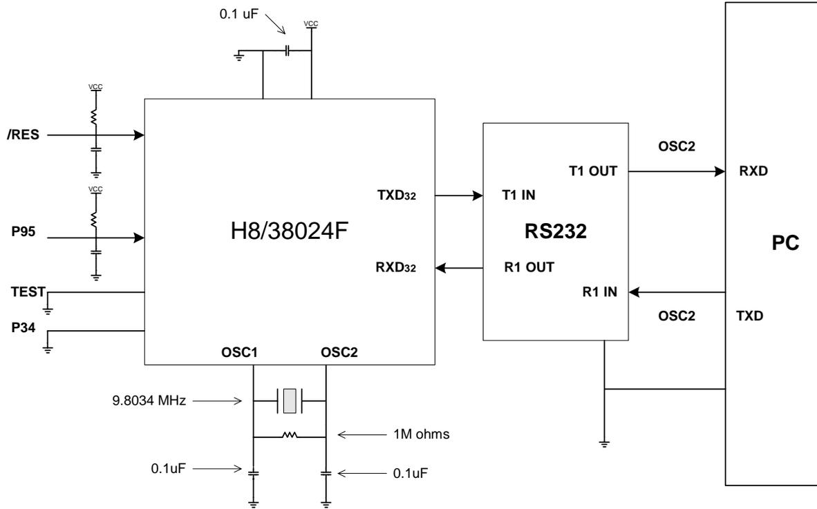
Figure 3.1 Block Diagram of Onboard Flash Circuitry
