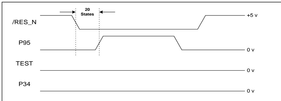
Figure 2.1 Reset Timing of Boot Mode
