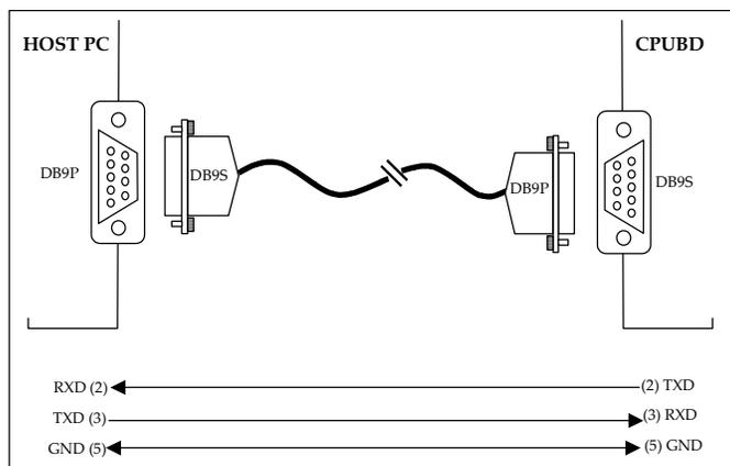
Figure 2.2 Serial Connection
