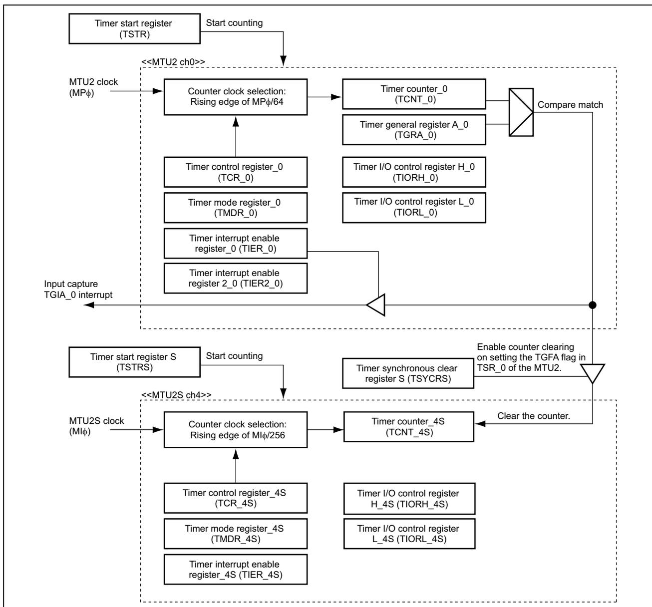
Figure 2 Operational Block Diagram of Channel 0 of MTU2 and Channel 4 of MTU2S
