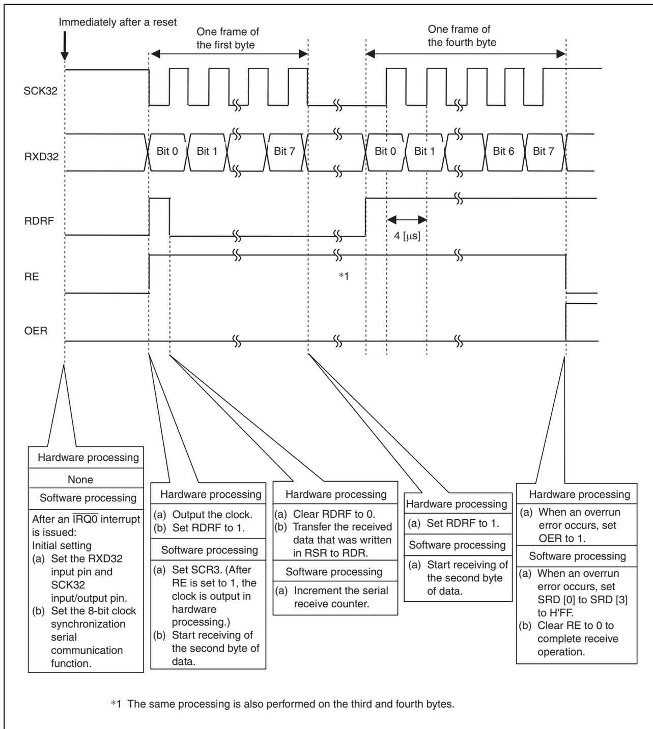
Figure 3 Operation during Reception of Data
