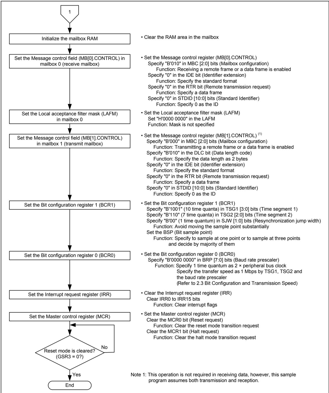
Figure 3 Flow Chart for Configuring the CAN Module (2/2)
