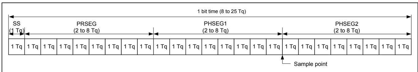
**Figure 4 Bit Configuration**
