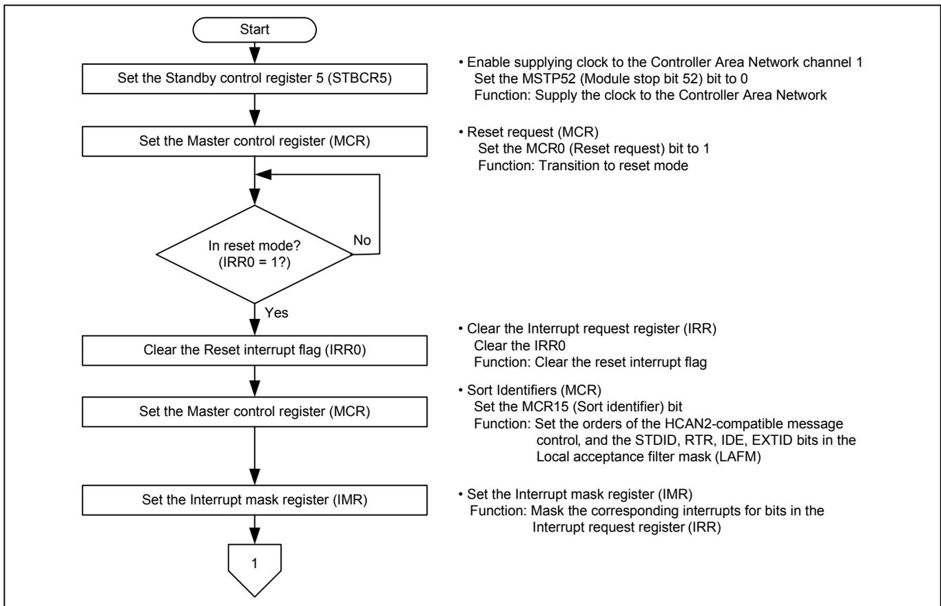
Figure 2 Flow Chart for Configuring the CAN Module (1/2)
