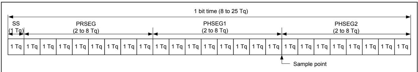
Figure 4 Bit Configuration
