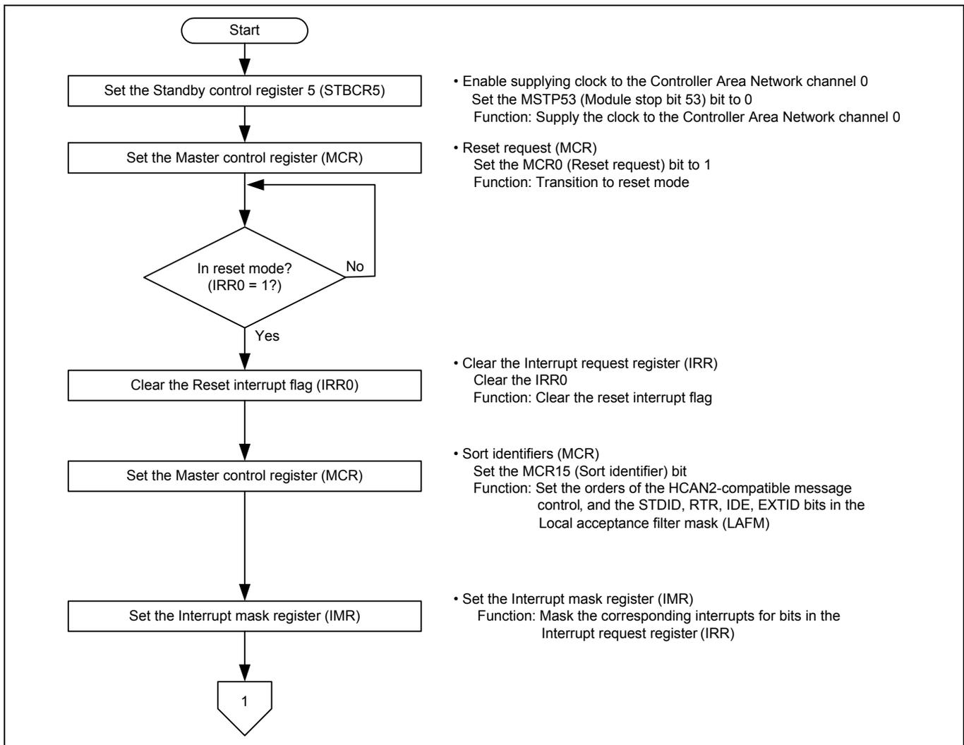
Figure 2 Flow Chart for Configuring the CAN Module (1/2)
