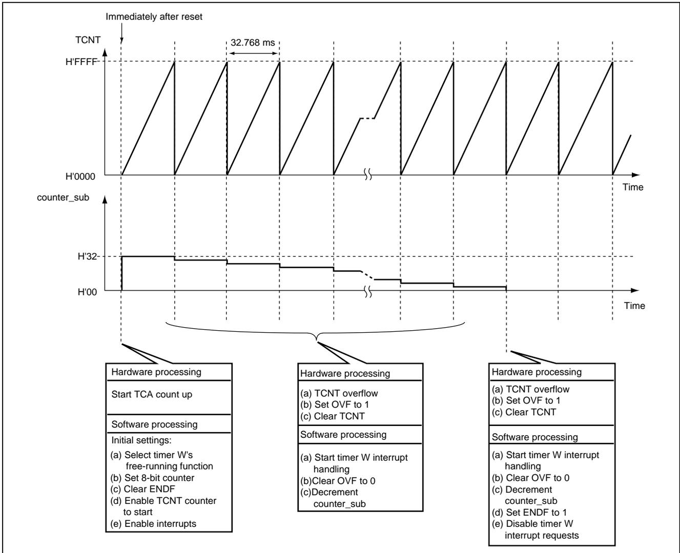
Figure 3.1 Operation Principle: Using 16-Bit Free-Running Function of Timer W to Count Interrupts
