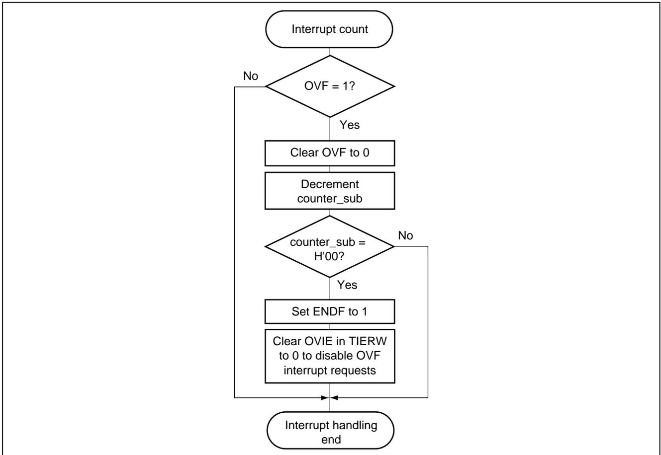
**Figure 5.2 Flowchart for Timer W Interrupt Handling Routine**
