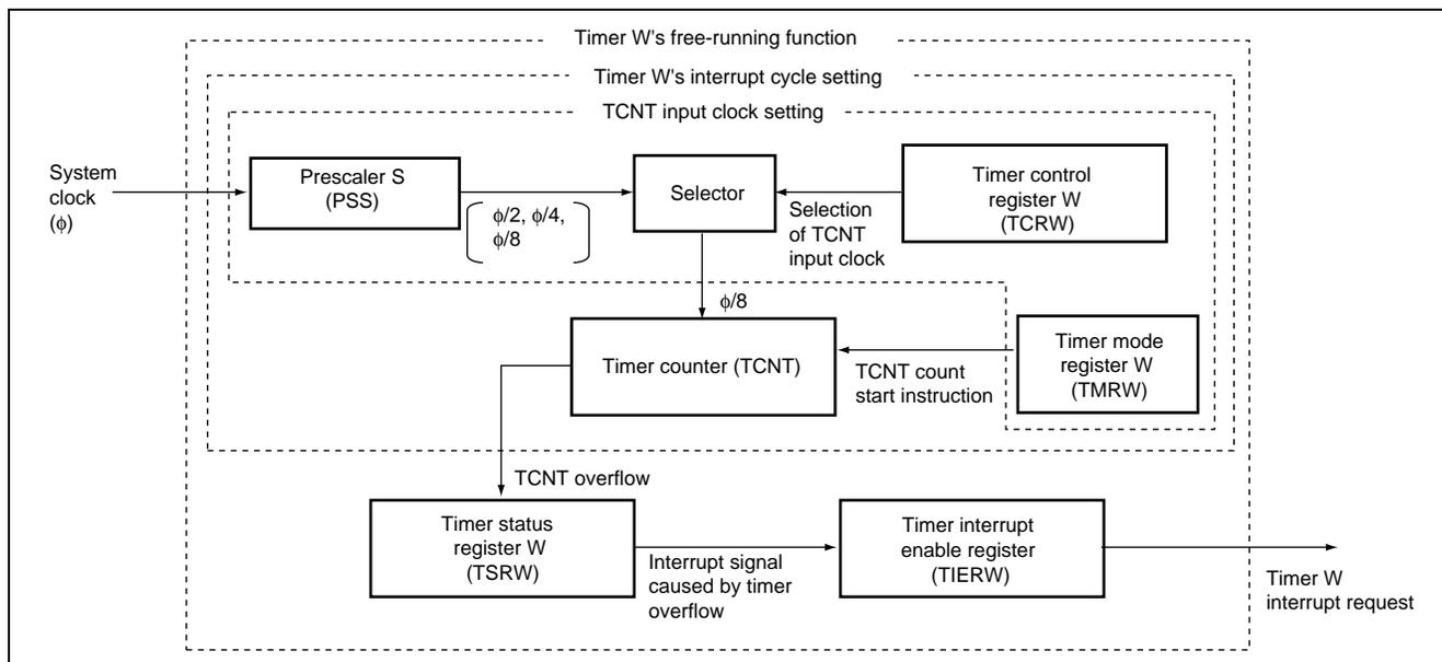
**Figure 2.1 Timer W's 16-Bit Free-Running Function**
