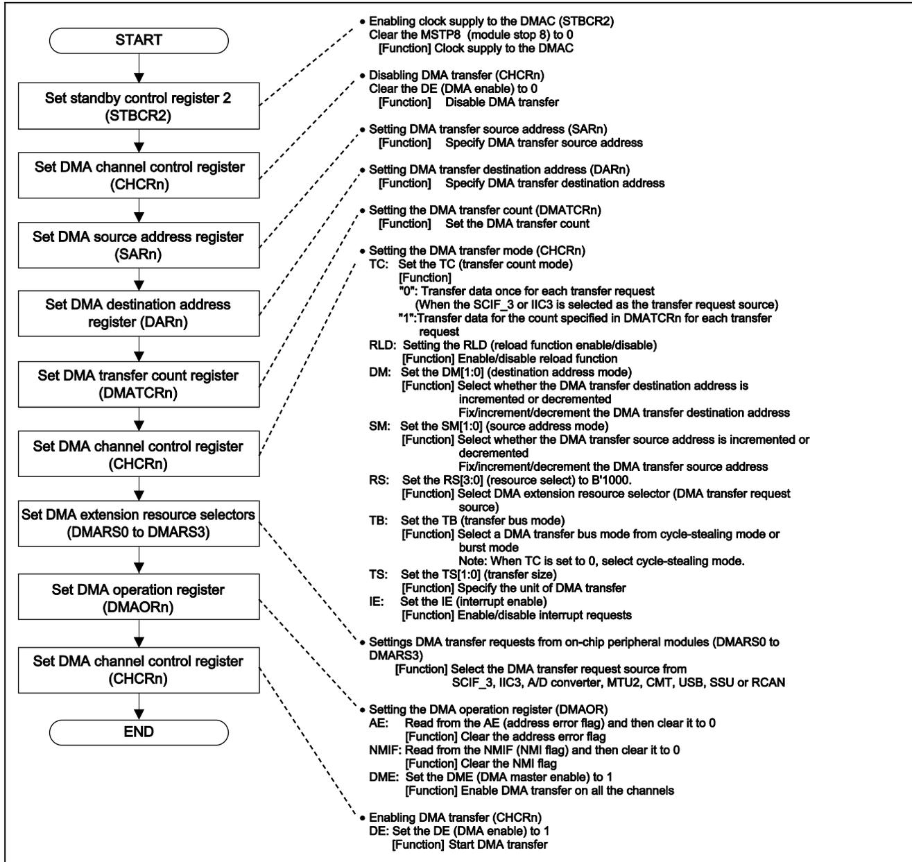
Figure 2 Flowchart of DMAC Initialization
