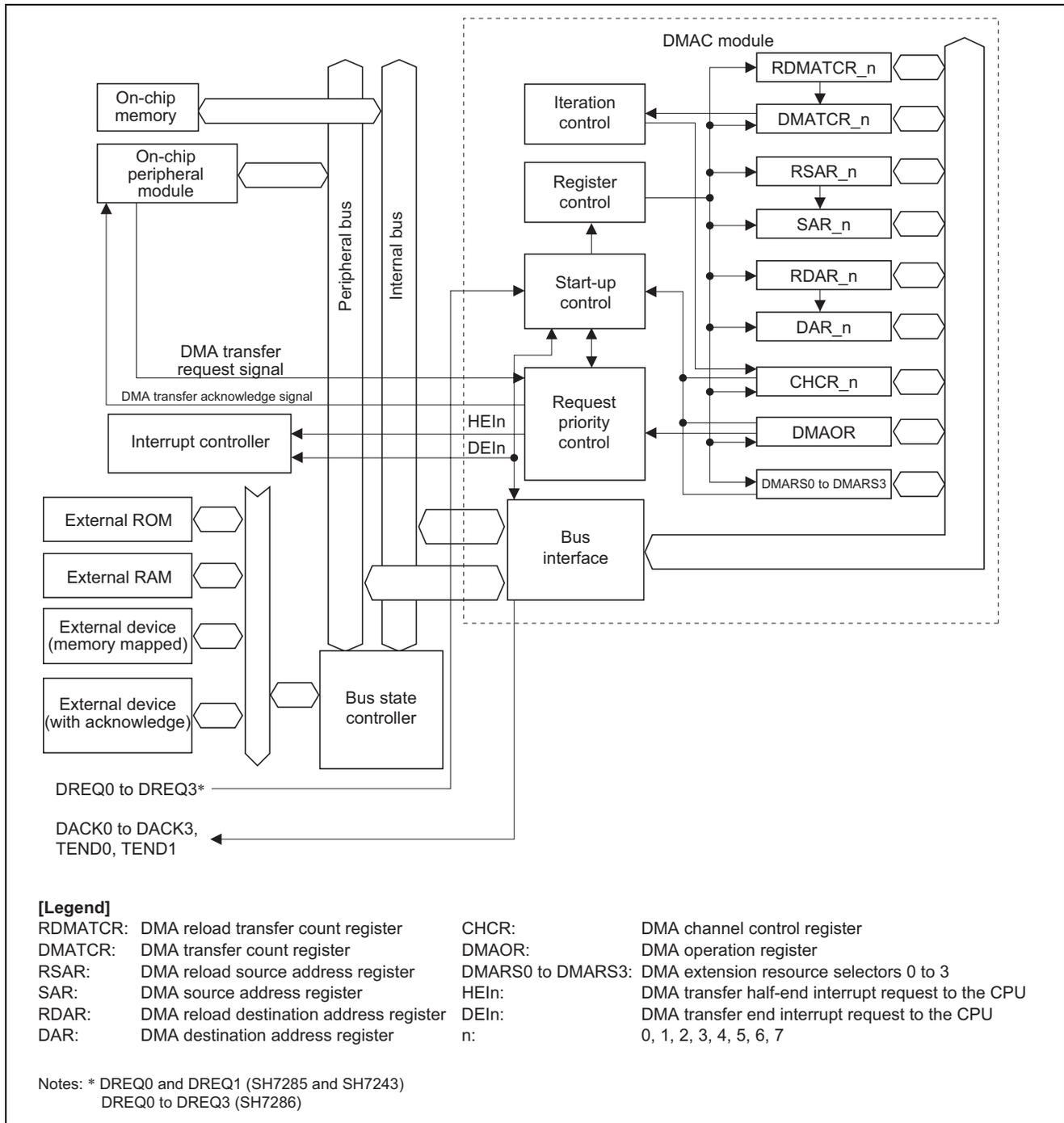
Figure 1 Block Diagram of DMAC
