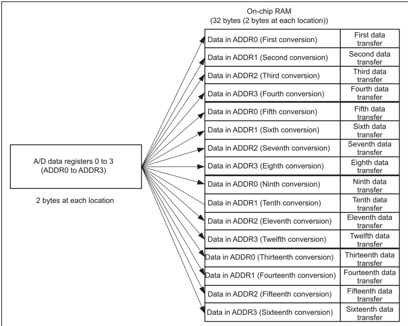
Figure 2 Flow of Data in Repeat Transfer Mode
