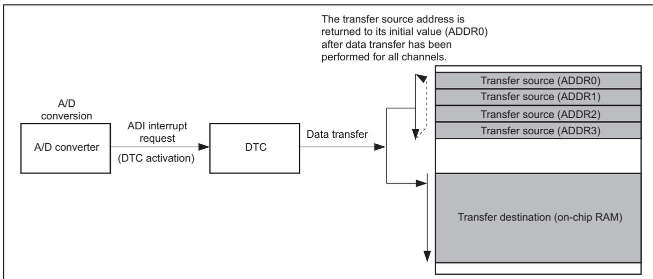
Figure 1 Overview of DTC Operation
