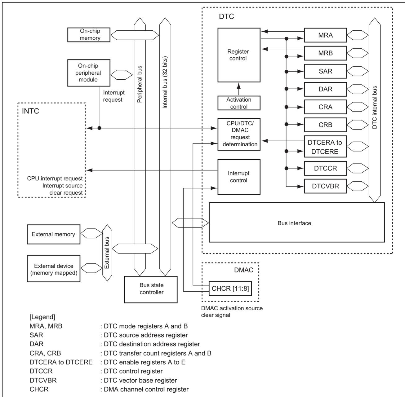
Figure 3 Block Diagram of the DTC
