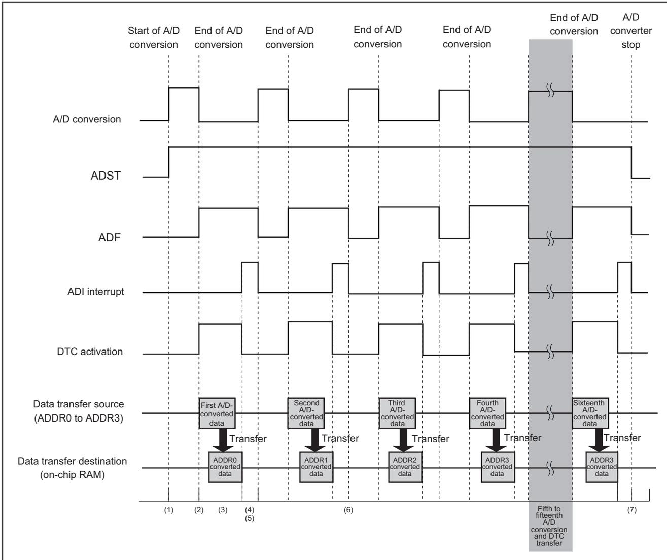
Figure 4 Timing of A/D Conversion and DTC Transfer
