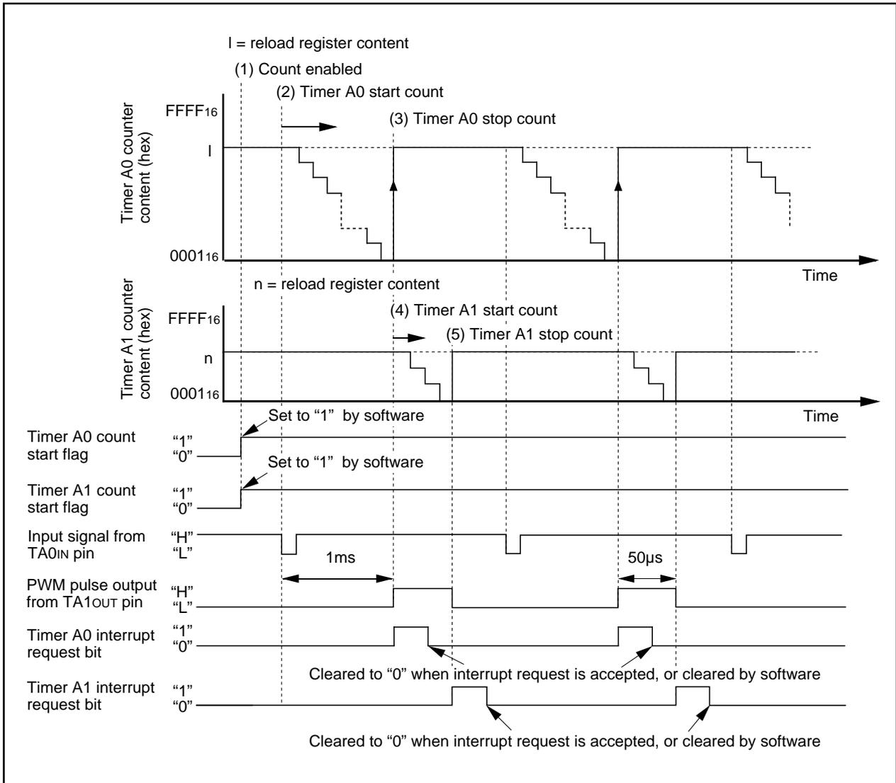
Figure 1. Operation timing of delayed one-shot output
