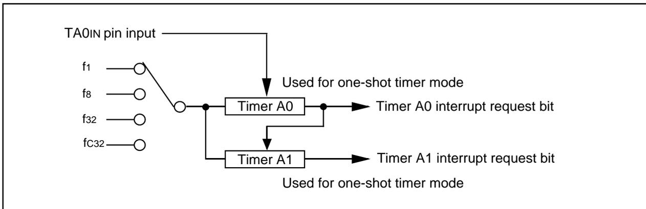
Figure 2. Connection diagram of delayed one-shot output
