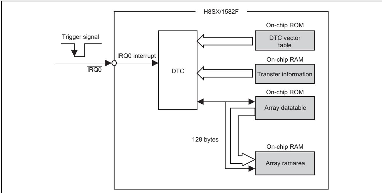
Figure 1 Block Diagram of DTC Data Transfer
