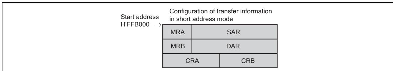
**Figure 4 Configuration of Transfer Information in Short Address Mode**
