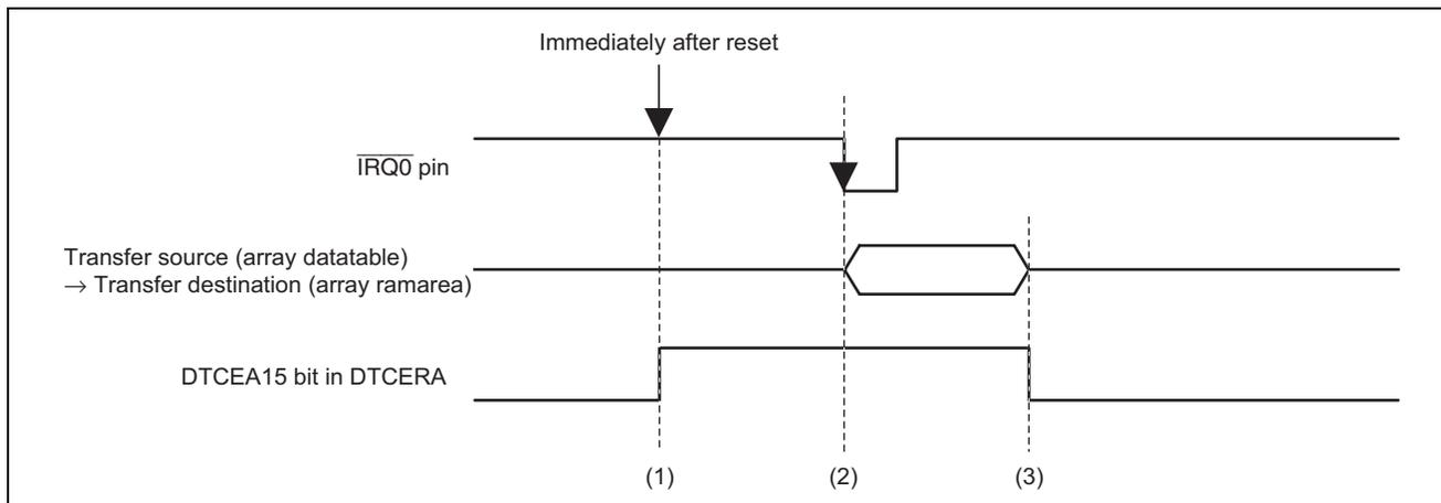
**Figure 3 Data Transfer Operation Initiated by IRQ0 Interrupt**
