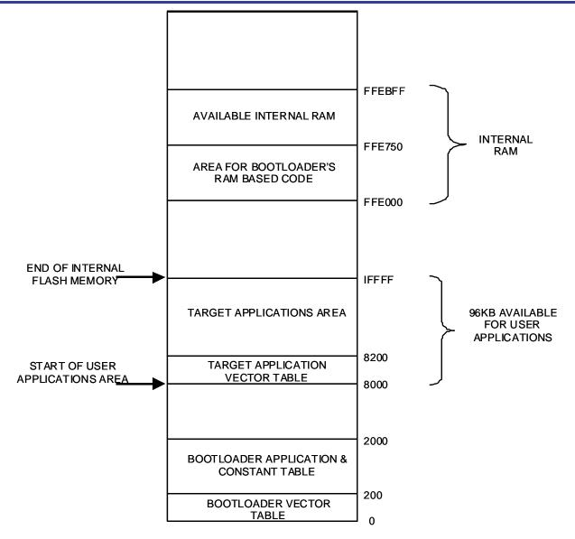
Figure 3: Bootloader and Target Application Memory Map
