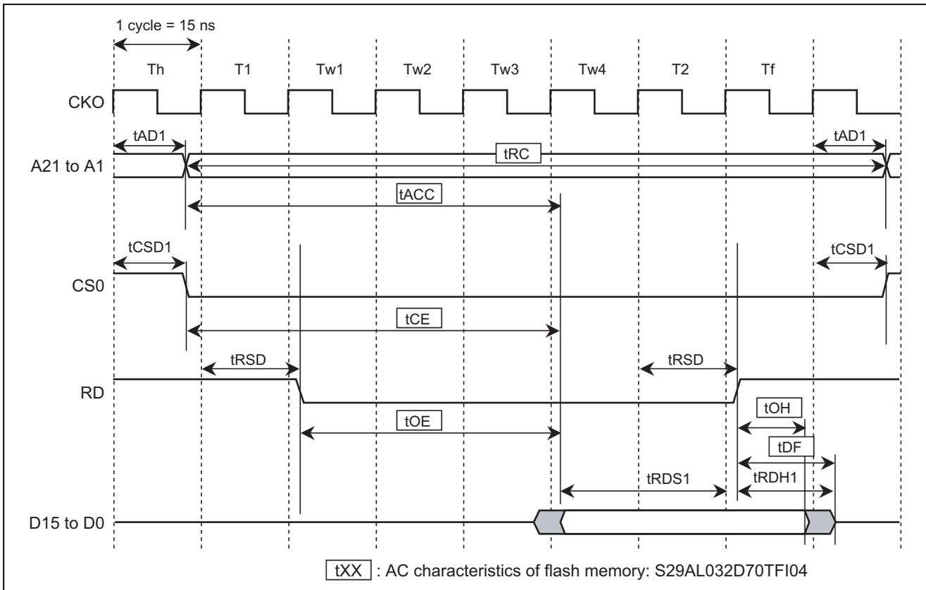
Figure 6 Read Timing for Flash Memory (tRSD = Max.)
