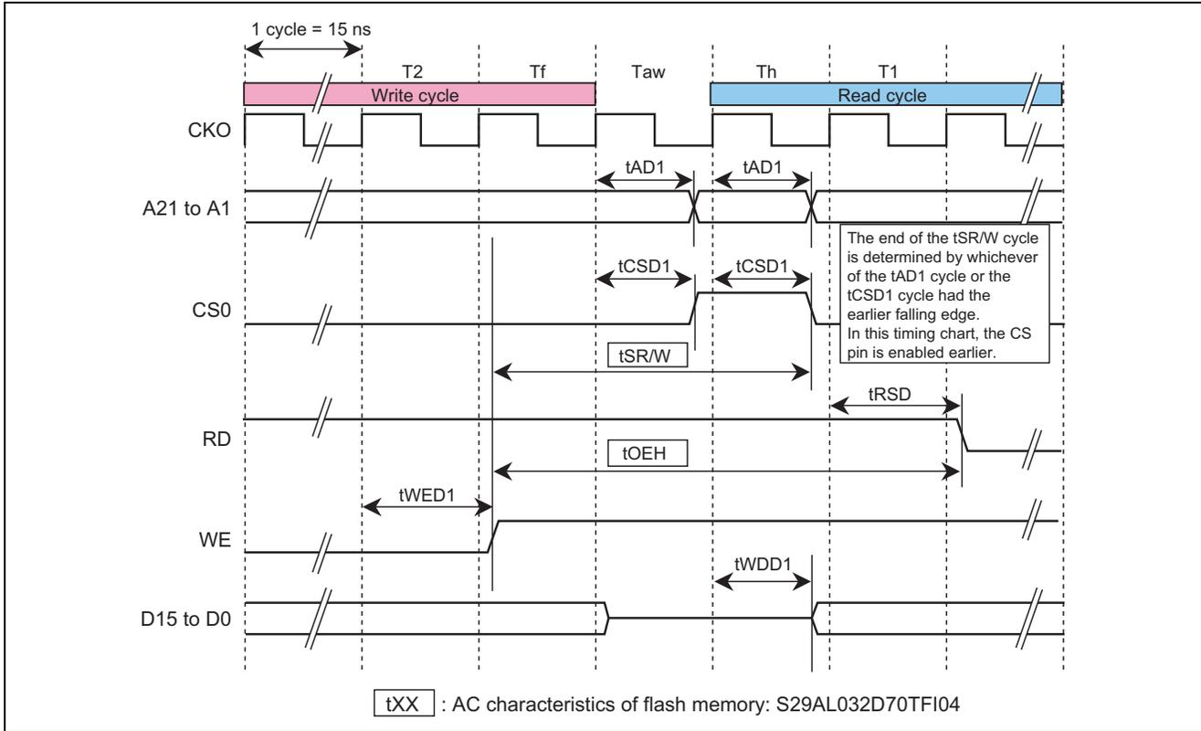
Figure 9 Timing between Write and Read Cycles for Flash Memory
