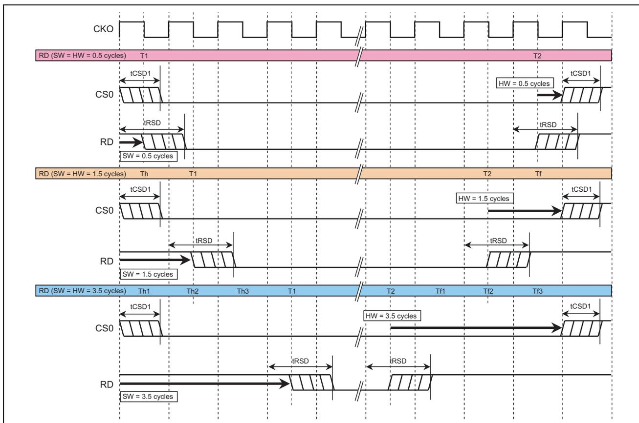
Figure 4 Relations between Delay Cycles and Delay Time
