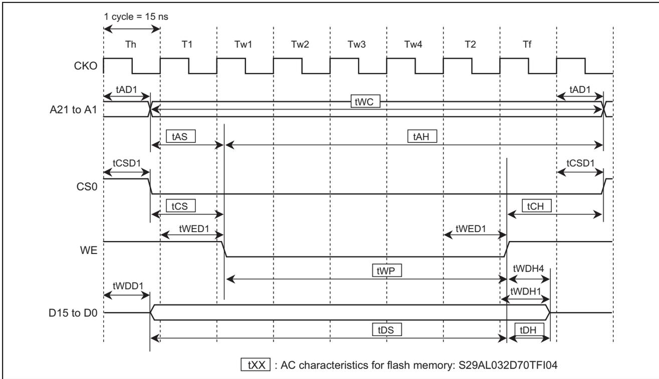
Figure 7 Write Timing for Flash Memory
