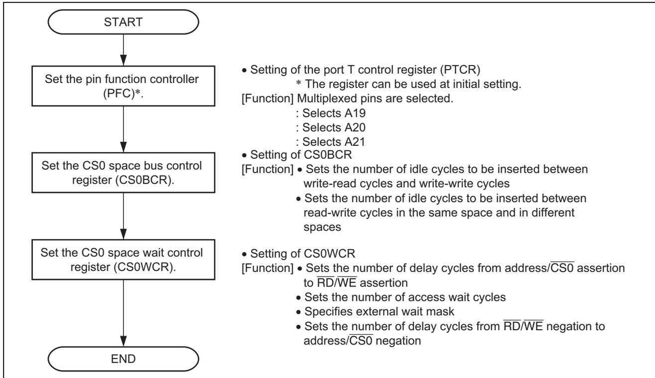
**Figure 3 Example of Procedure for Setting Bus State Controller (CS0 Space)**
