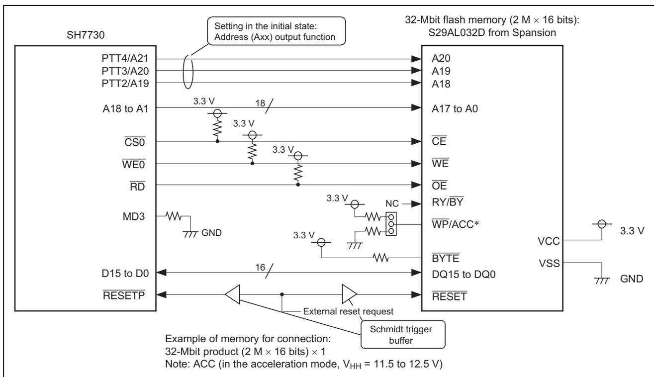
**Figure 2 Circuit Example for Flash Memory Connection (4 MB, 16-Bit Bus)**
