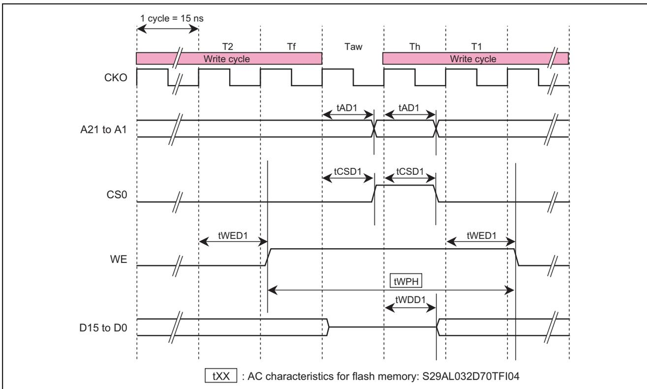
Figure 8 Timing between Write and Write Cycles for Flash Memory
