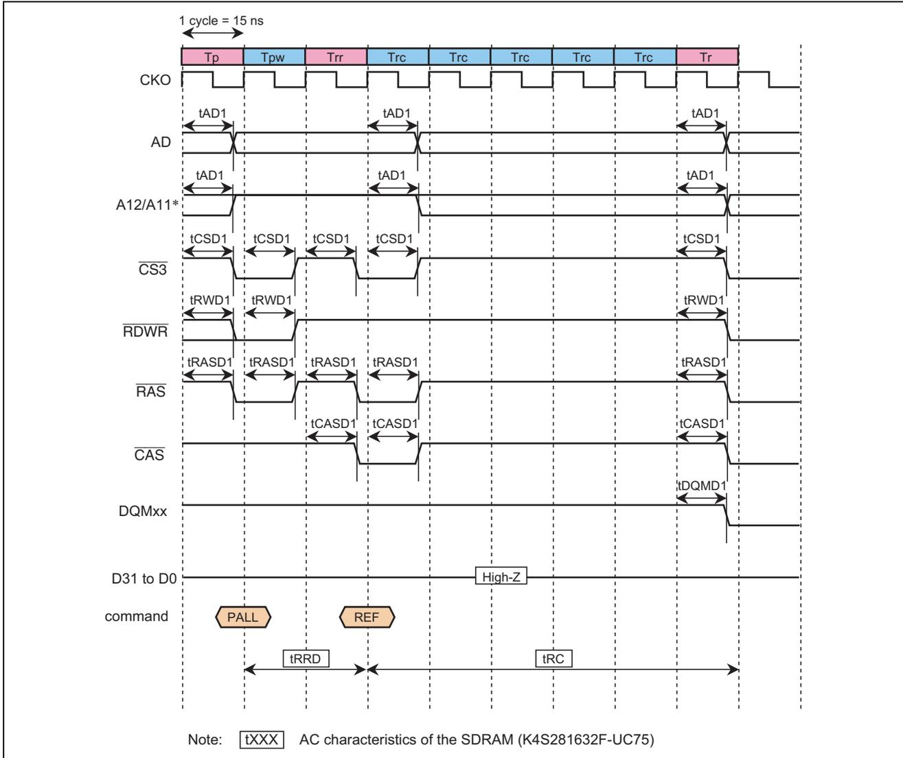
Figure 9 Timing for Refreshing of the SDRAM
