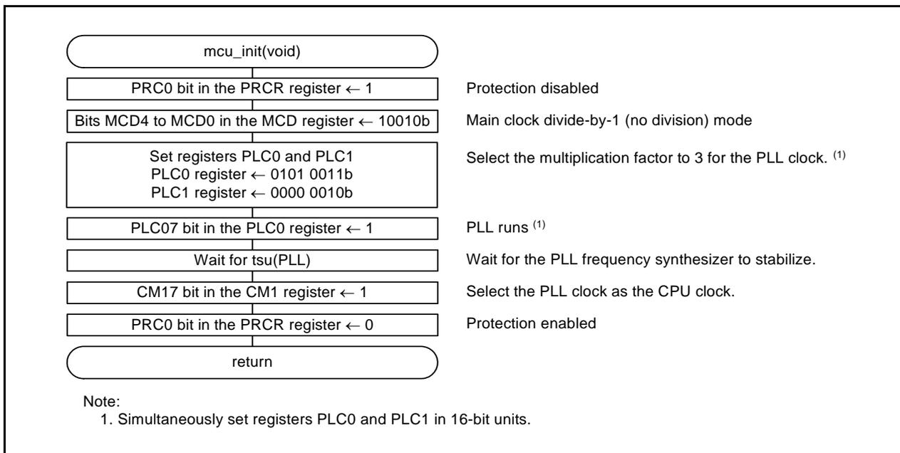
Figure 7.2 CPU Initial Setting Function
