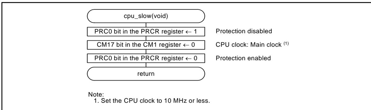
Figure 7.4 CPU Slow Down Processing Function
