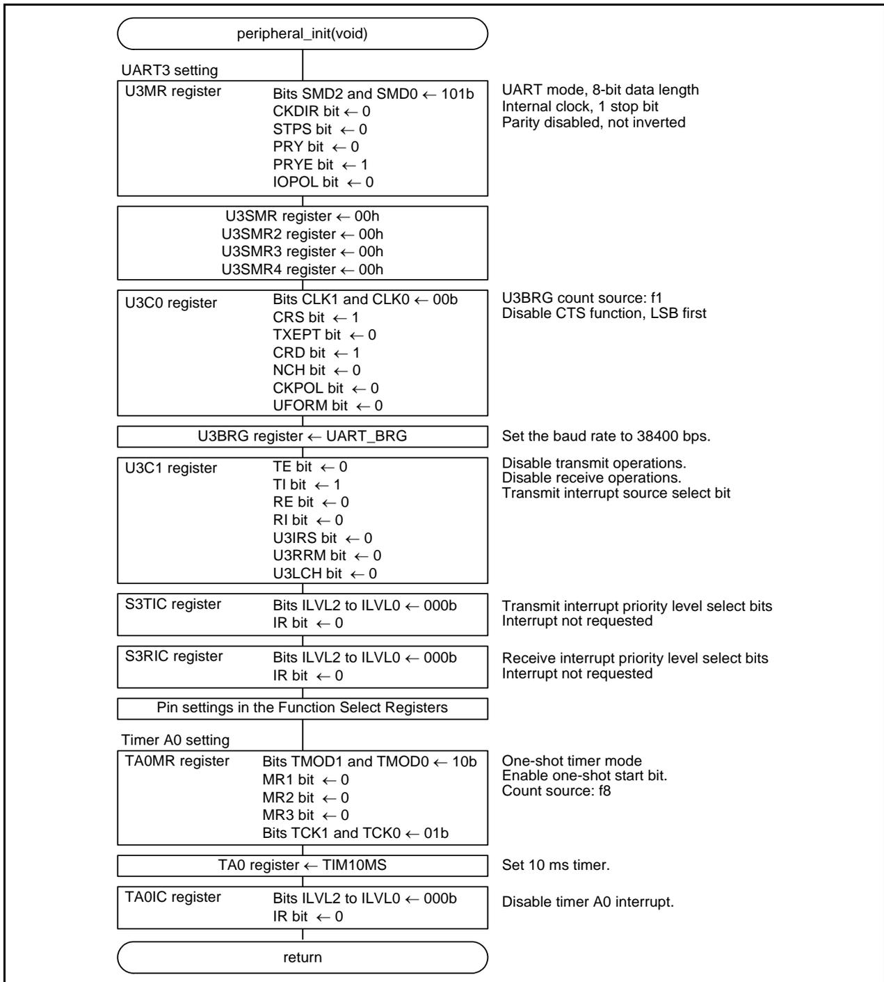
Figure 7.3 Peripheral Function Initial Setting Function
