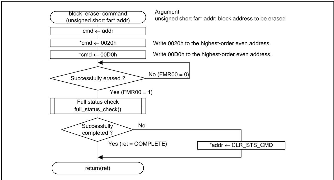
Figure 7.13 Block Erase Function
