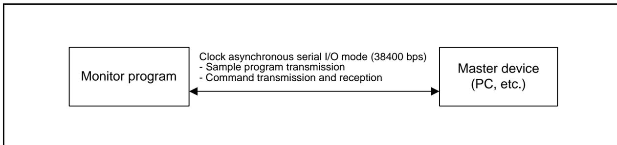
**Figure 4.1 System Structure Diagram**
