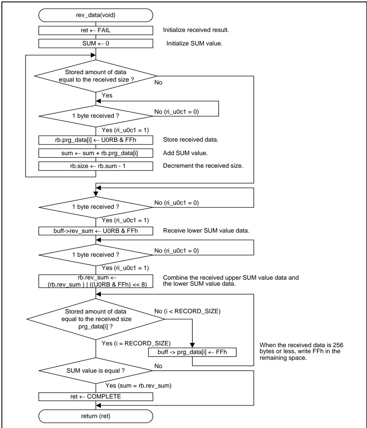
Figure 7.9 Program Data Receive Function
