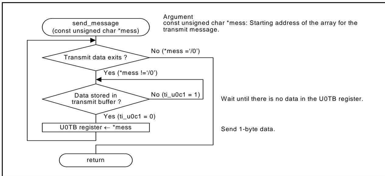
Figure 7.10 Message Transmit Function
