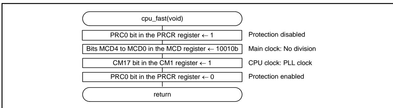
Figure 7.5 CPU Speed Up Processing Function
