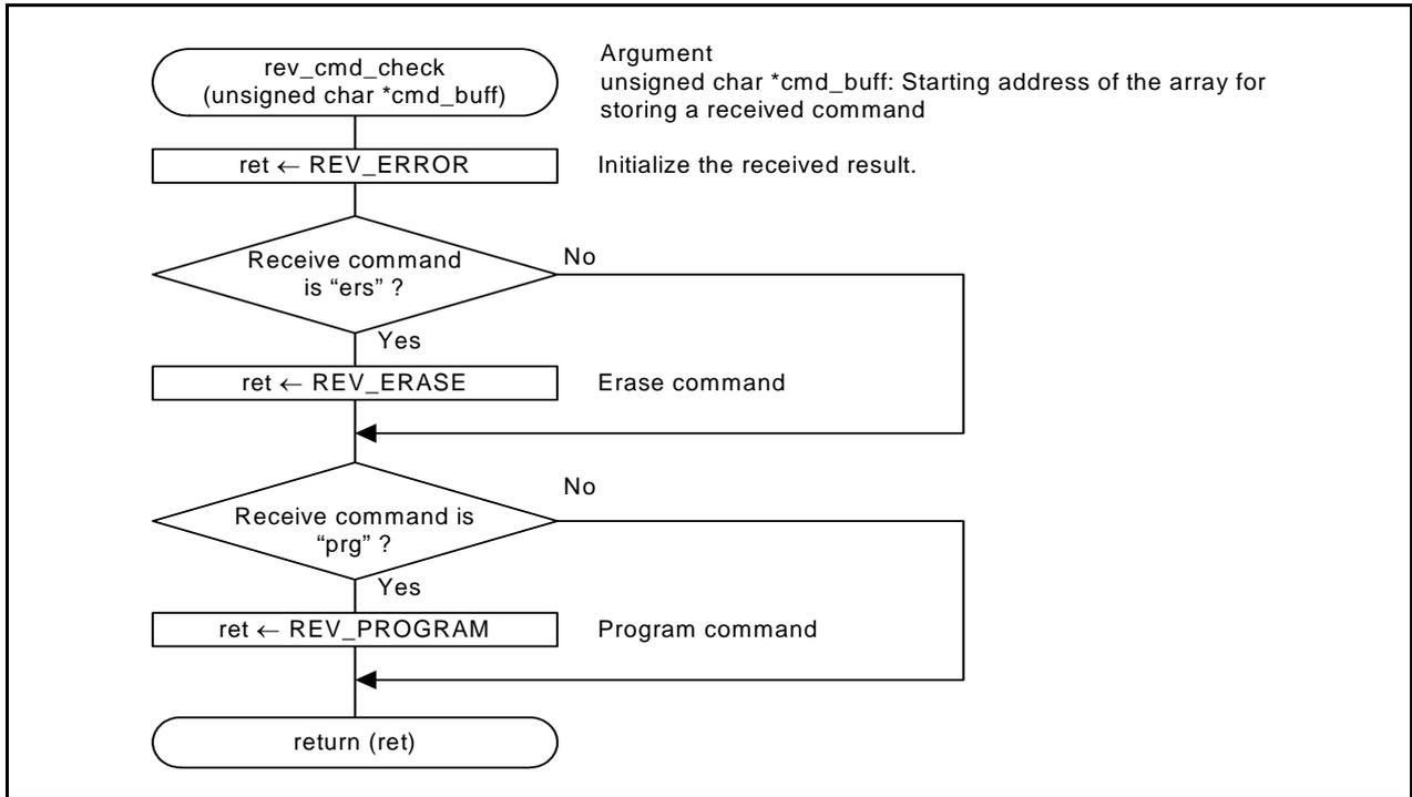
Figure 7.7 Command Check Function
