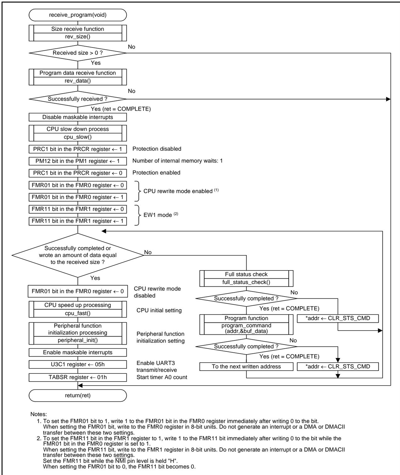
Figure 7.12 Flash Memory Write Function
