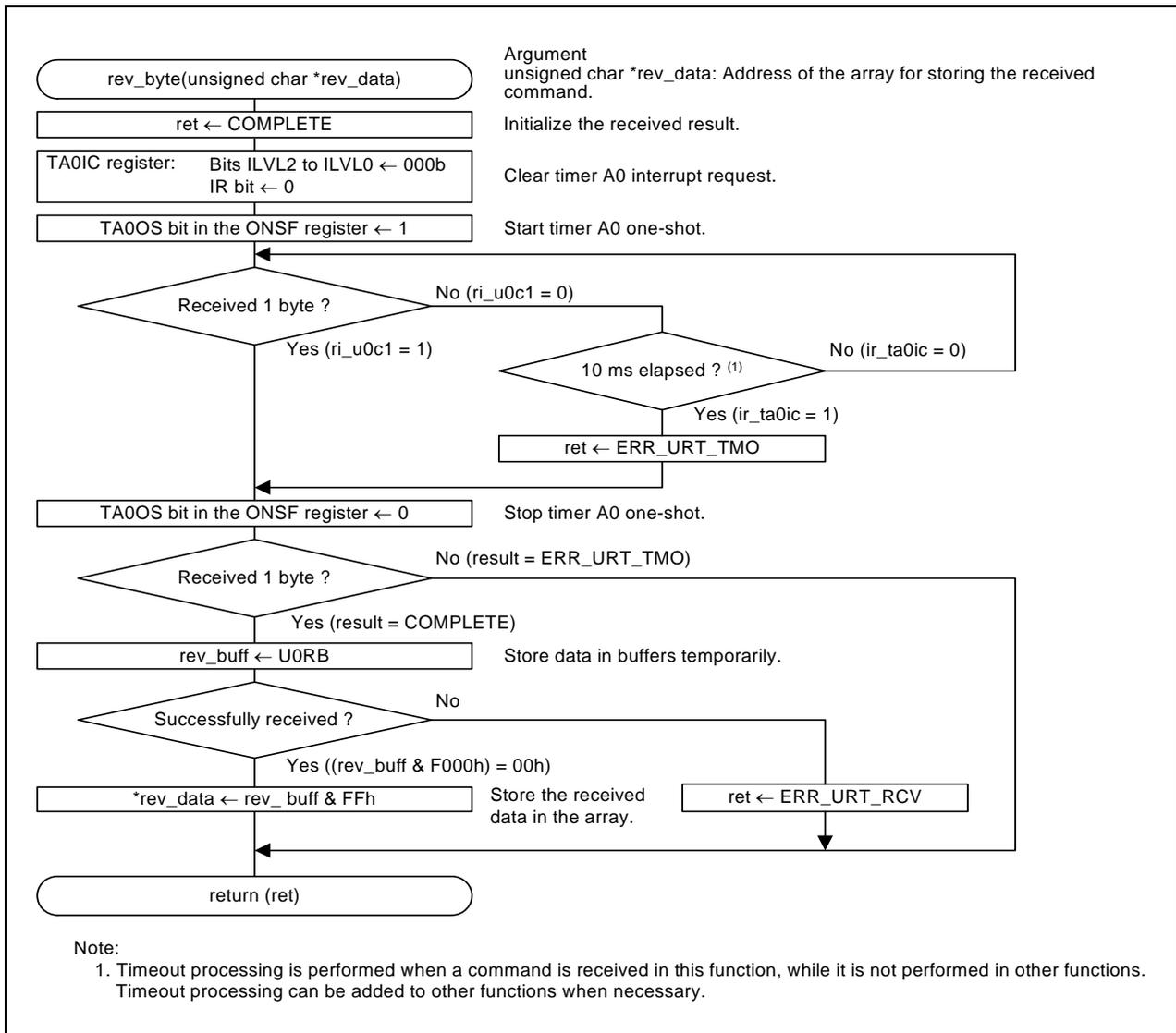
Figure 7.6 1-byte Command Receive Function
