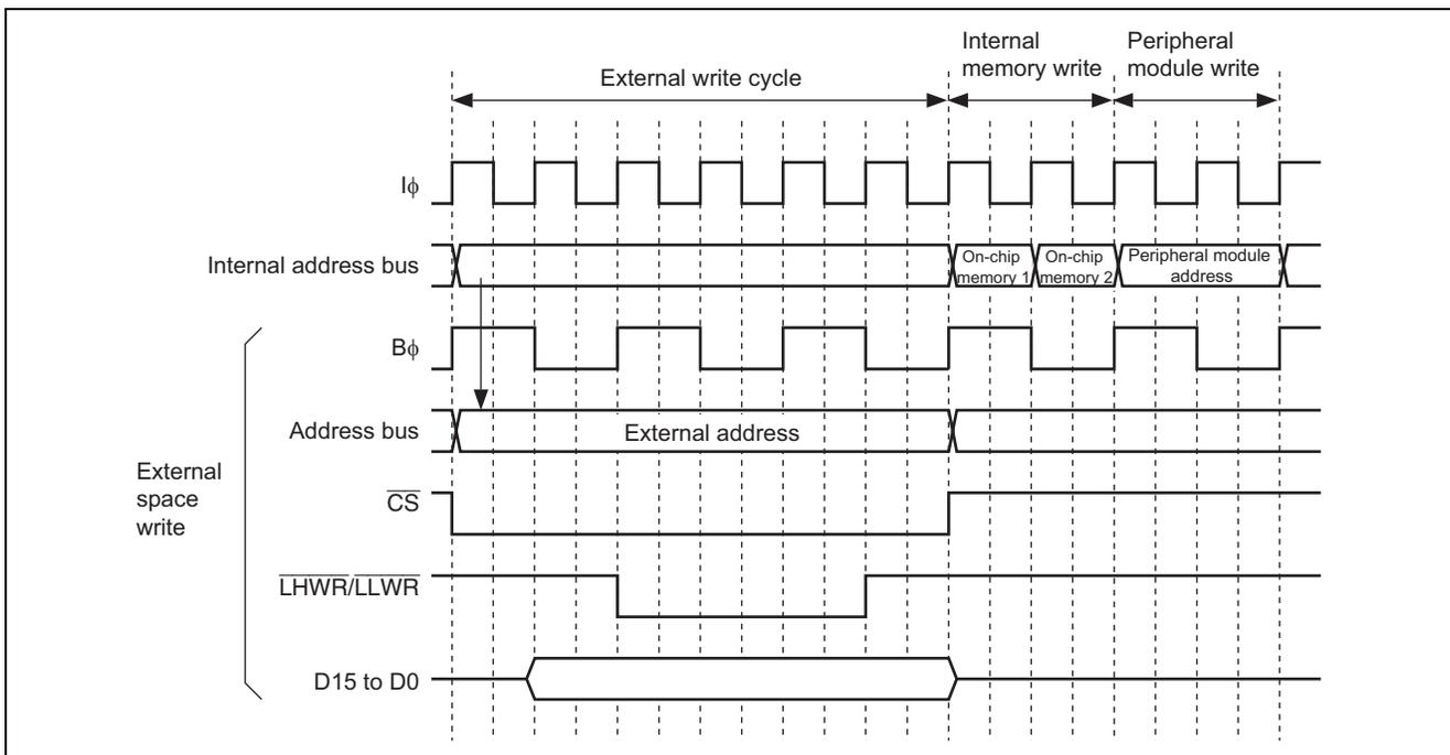
Figure 1 Example of Timing when the External-Write-Data Buffer is Not in Use (WDBE = 0)
