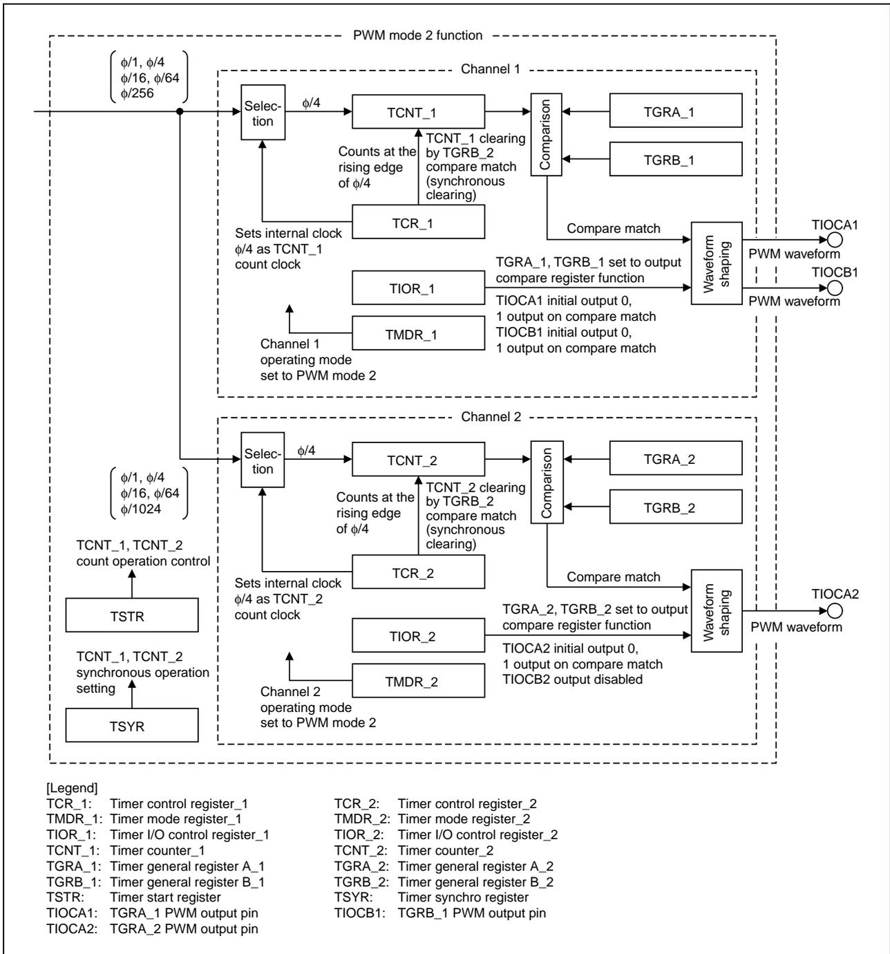
Figure 2 Block Diagram of PWM Mode 2 Function
