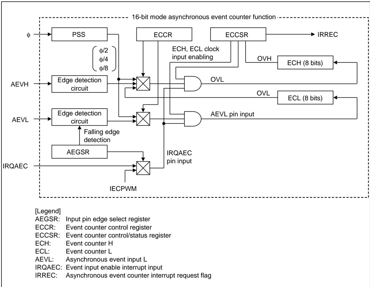
Figure 2 Block Diagram of the 16-Bit Mode Asynchronous Event Counter Function
