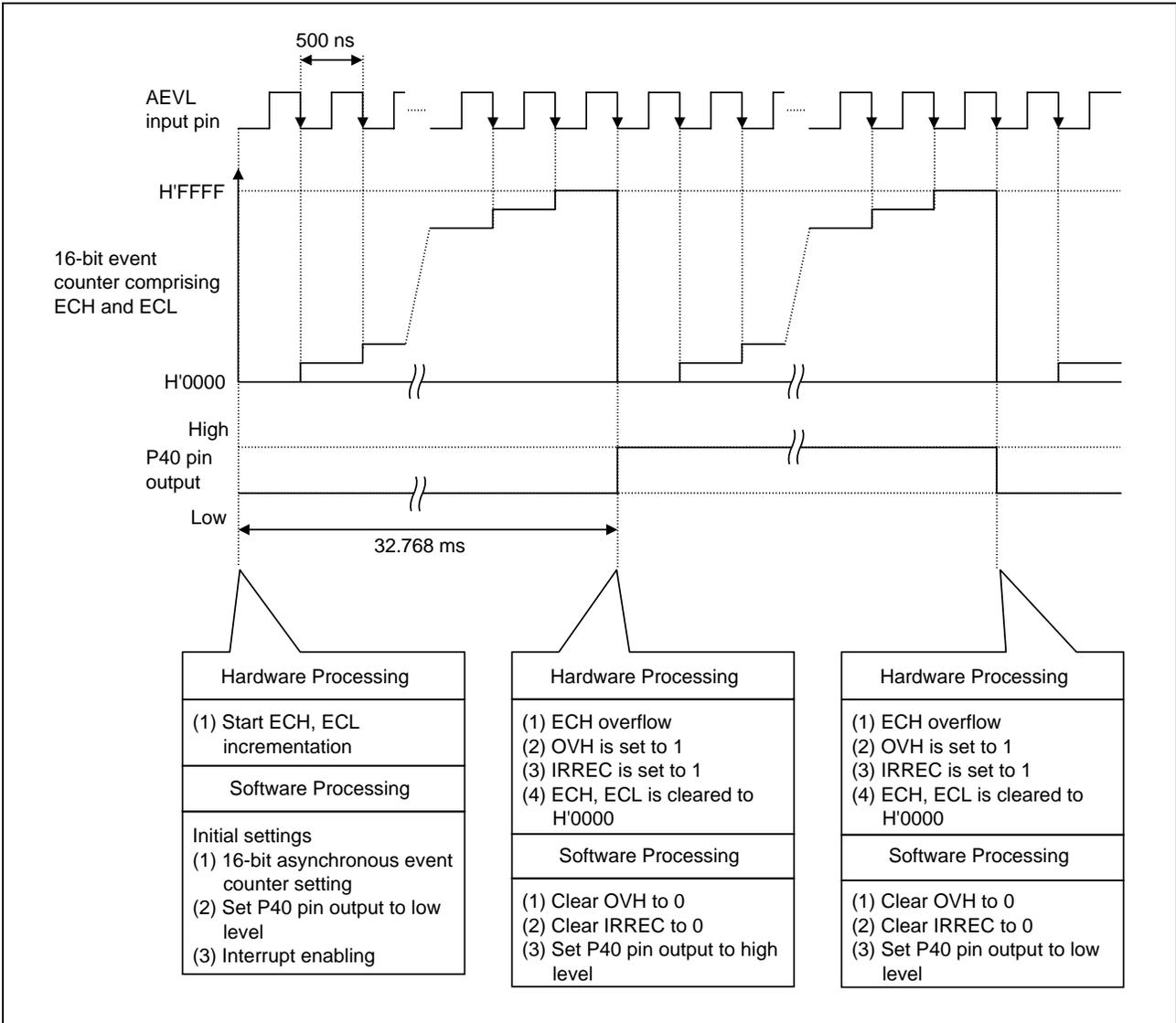
Figure 3 Principles of Operation
