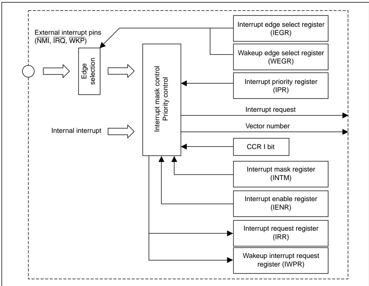
Figure 2 Block Diagram of Interrupt Controller
