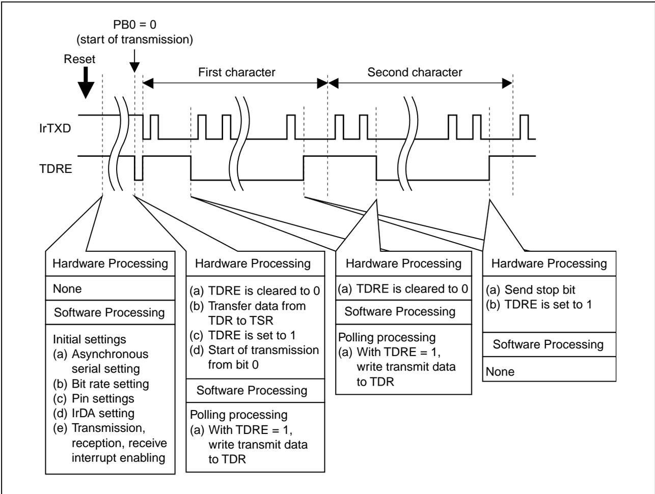
Figure 4 Principles of IrDA Transmit Operation
