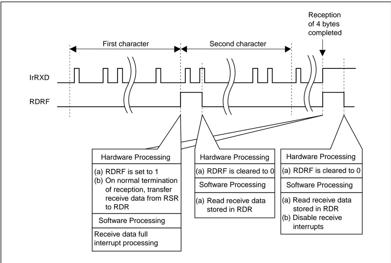
Figure 5 Principles of IrDA Receive Operation
