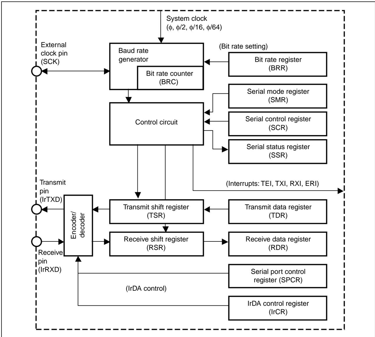
Figure 2 Block Diagram of SCI
