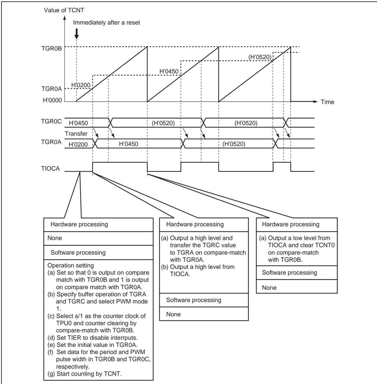
**Figure 3 PWM Pulse Output Operation**
