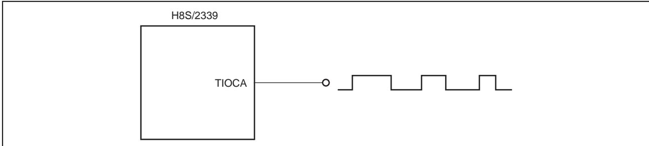
Figure 1 Example of PWM Waveform Output by TPU Buffer Operation
