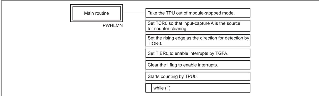
(2) Measurement of high and low widths of a pulse
