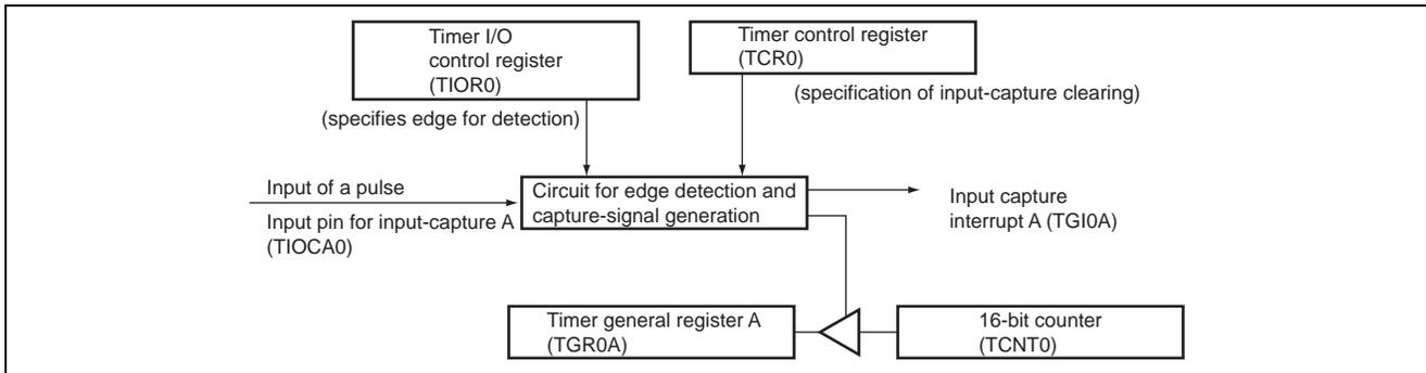
**Figure 2 Blocks Used in Measuring the High and Low Periods of a Pulse**
