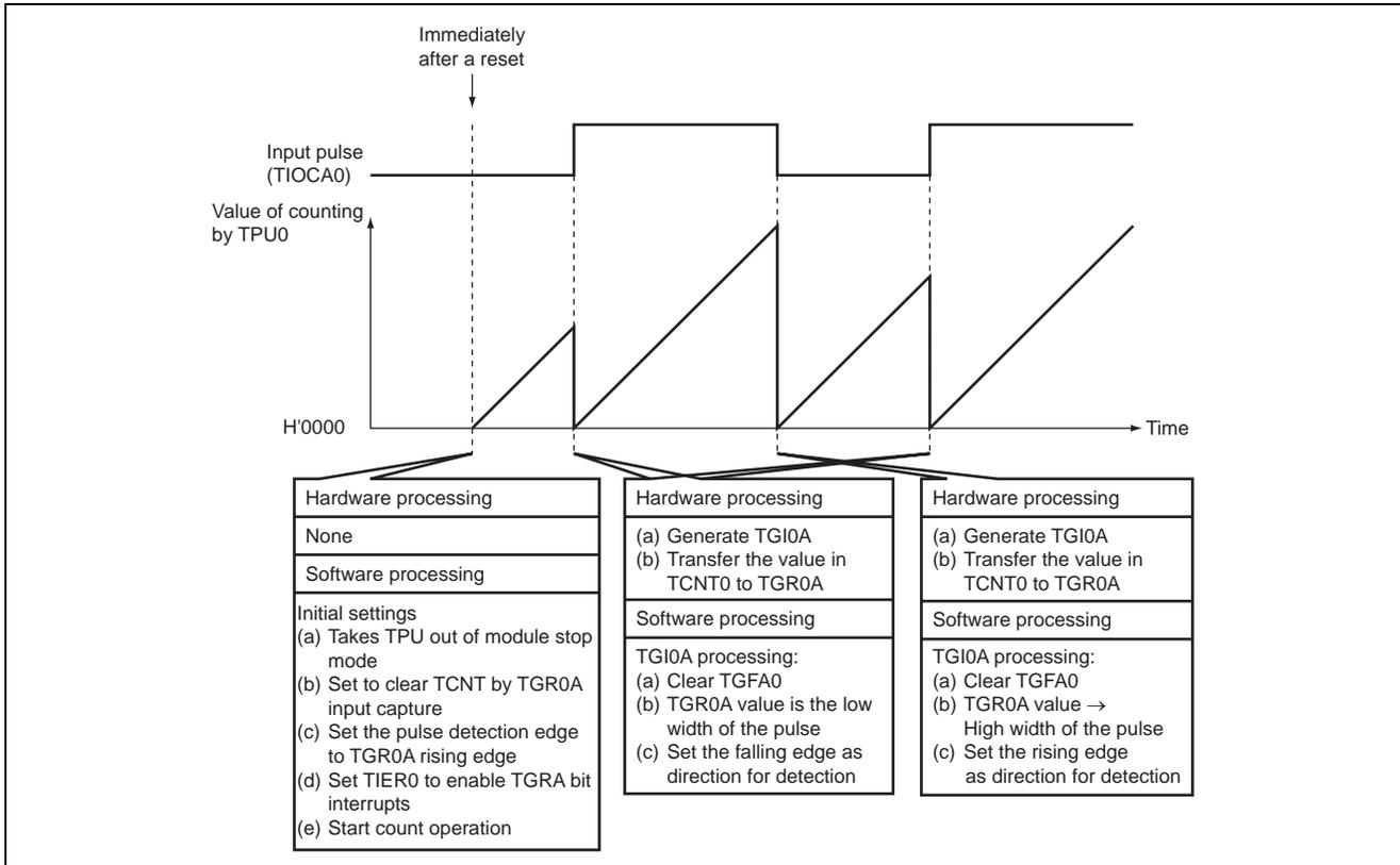
Figure 3 Measuring the Pulse Width
