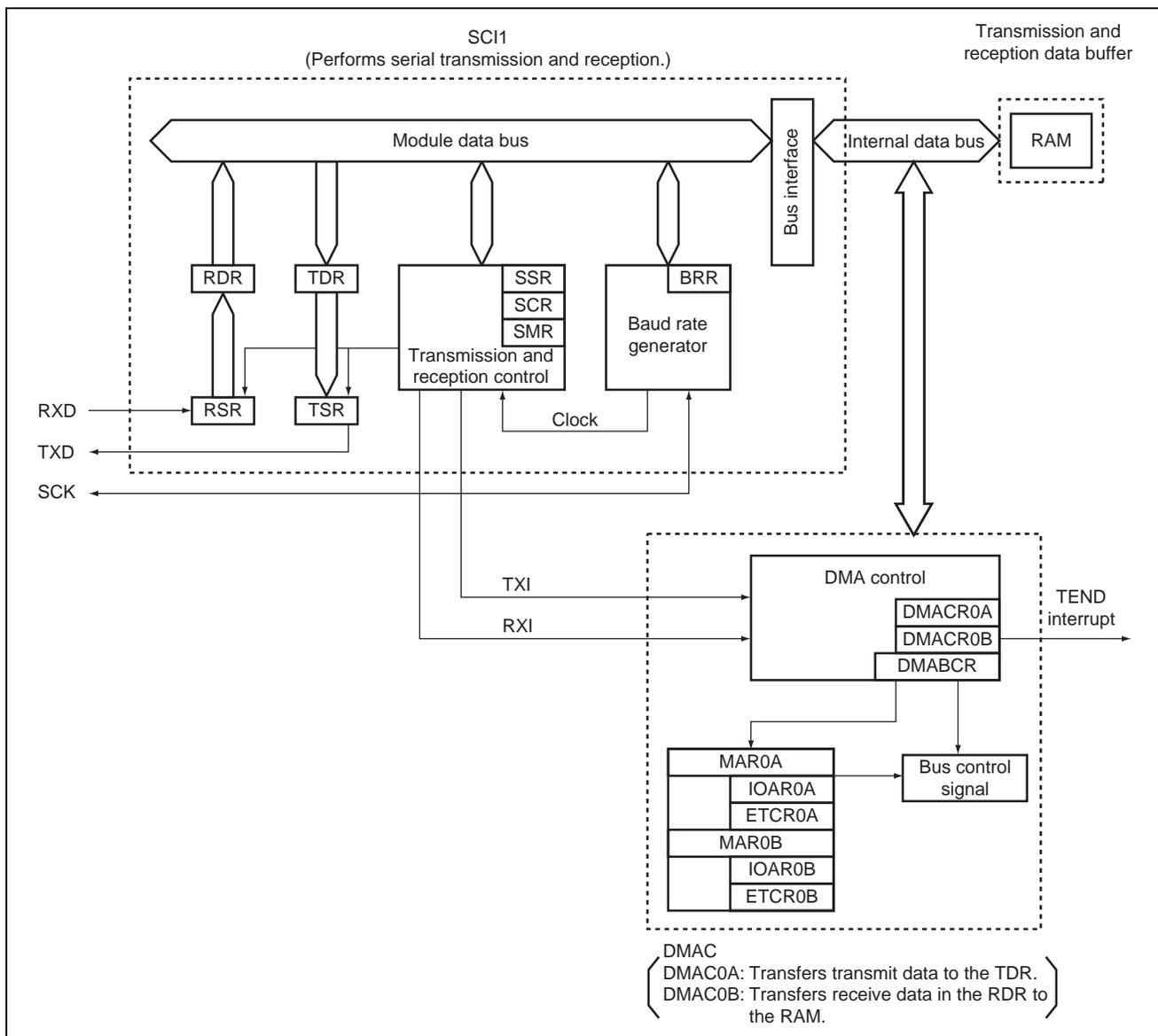
Figure 2 Block Diagram of Continuous Transmission and Reception
