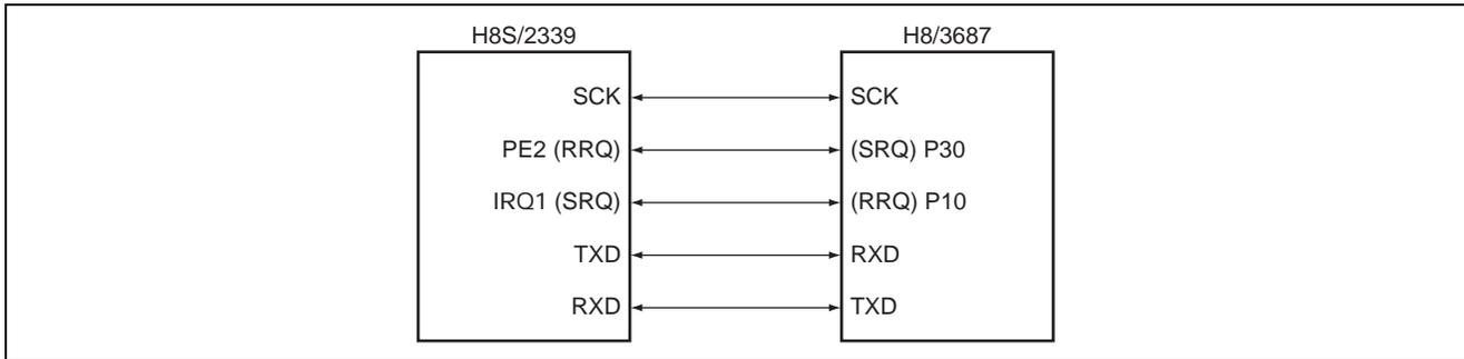
**Figure 1 Block Diagram of the Clock Synchronous Mode SCI by the H8S/2339**
