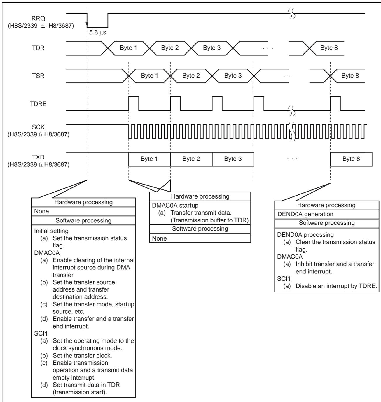
Figure 3 Principles of Operations Used of Data Transmission
