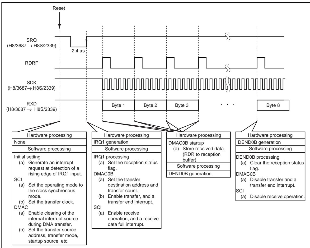
**Figure 4 Principles of Operations Used of Data Reception**
